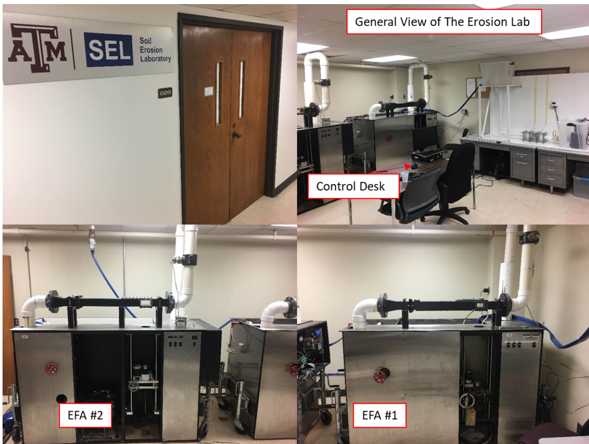
Figure 44. Erosion laboratory at Texas A&M University, showing the two EFAs and the control desk
