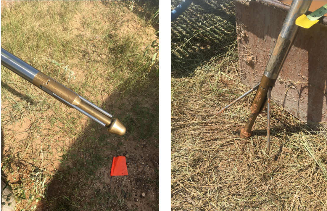
Figure 67. Photographs taken from the mechanical caliper (3 arms) in closed-arm and opened-arm conditions
