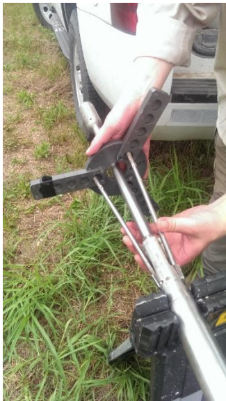
Figure 18- Borehole mechanical caliper
