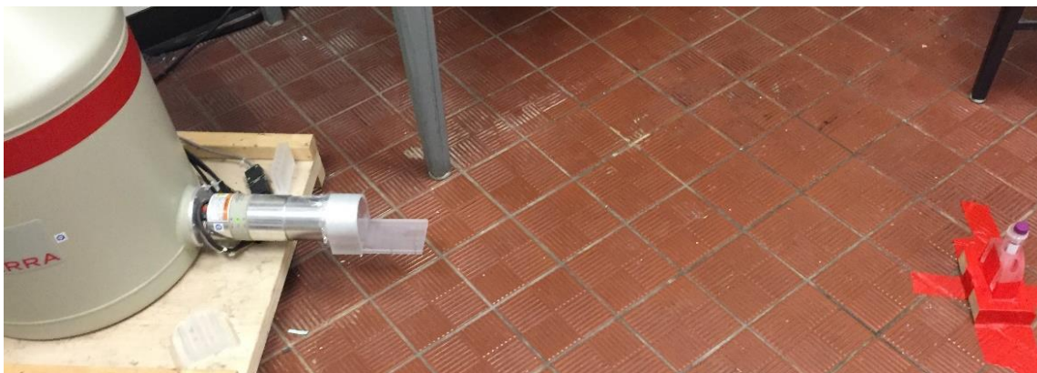
Figure 23: The initial gamma measurement setup for determining the burnup of each fuel disc.
