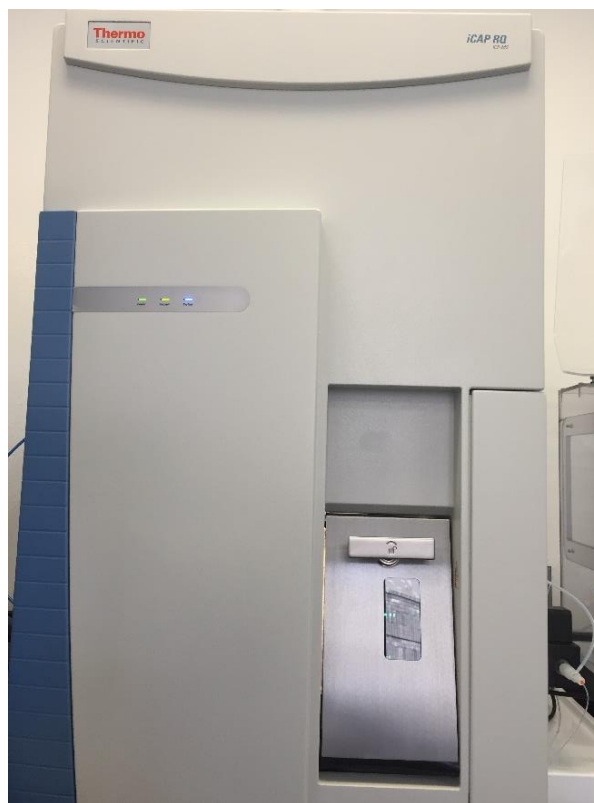
Figure 27: The Thermo Fisher Scientific iCAP RQ ICP-MS used for mass spectrometry measurements.
