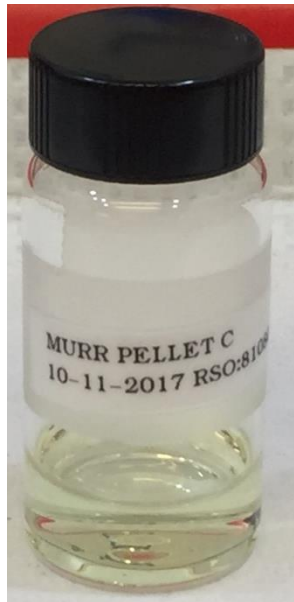
Figure 25: ~4.5 mL solution containing approximately 95% of the dissolved fuel disc.
