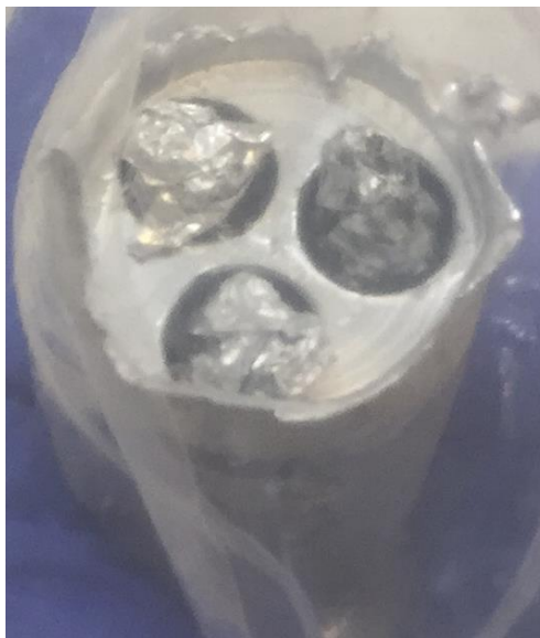
Figure 20: The irradiation capsule housing three wrapped fuel discs following the irradiation at MURR.
