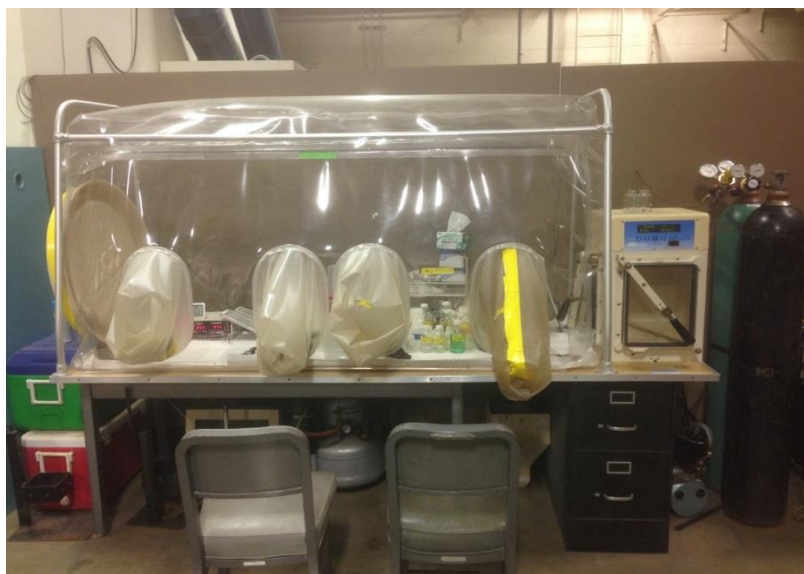
Fig. 3.1 Photograph of the anaerobic chamber used in this study
