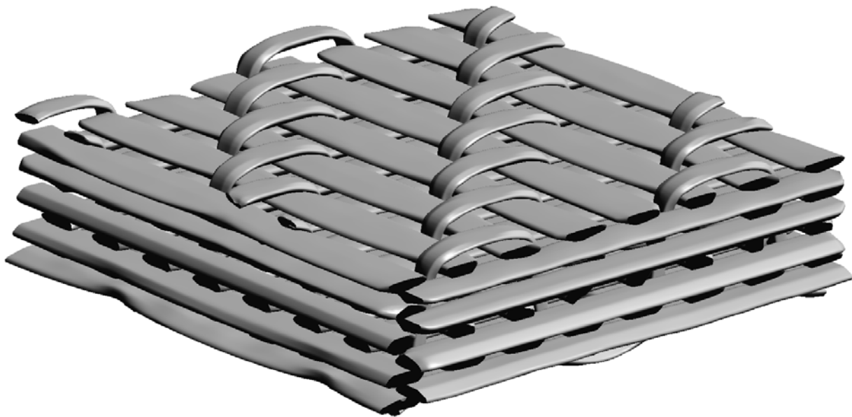
Figure 2.27. Tow surfaces after cross-sections are contracted
