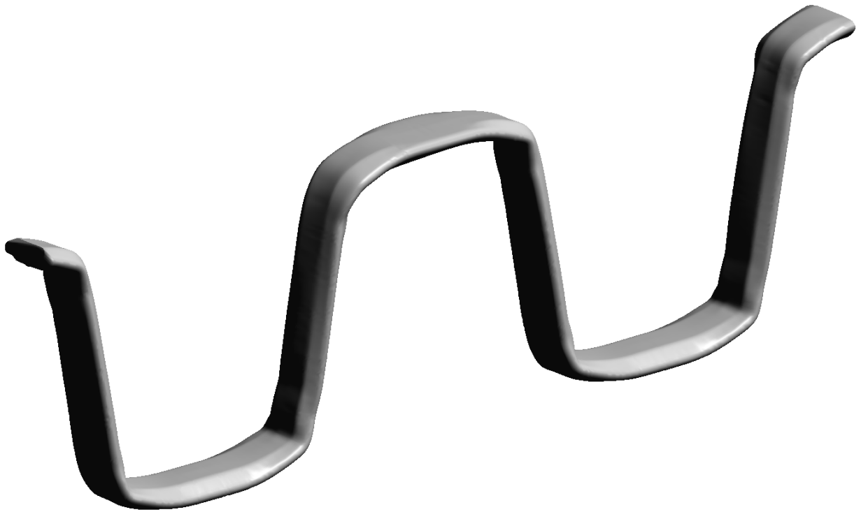
Figure 2.25. Tow surface using splines with a minimum radius of curvature 10x that of the digital chains
