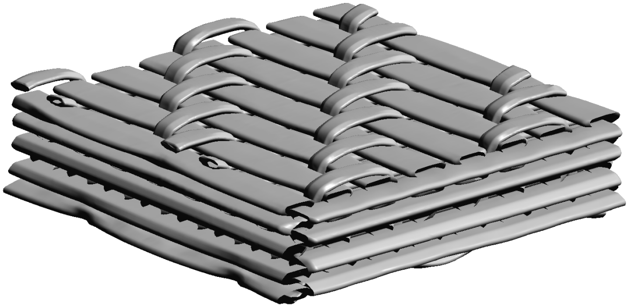
Figure 2.26. Tow surfaces based on the group of digital chains used for each tow
