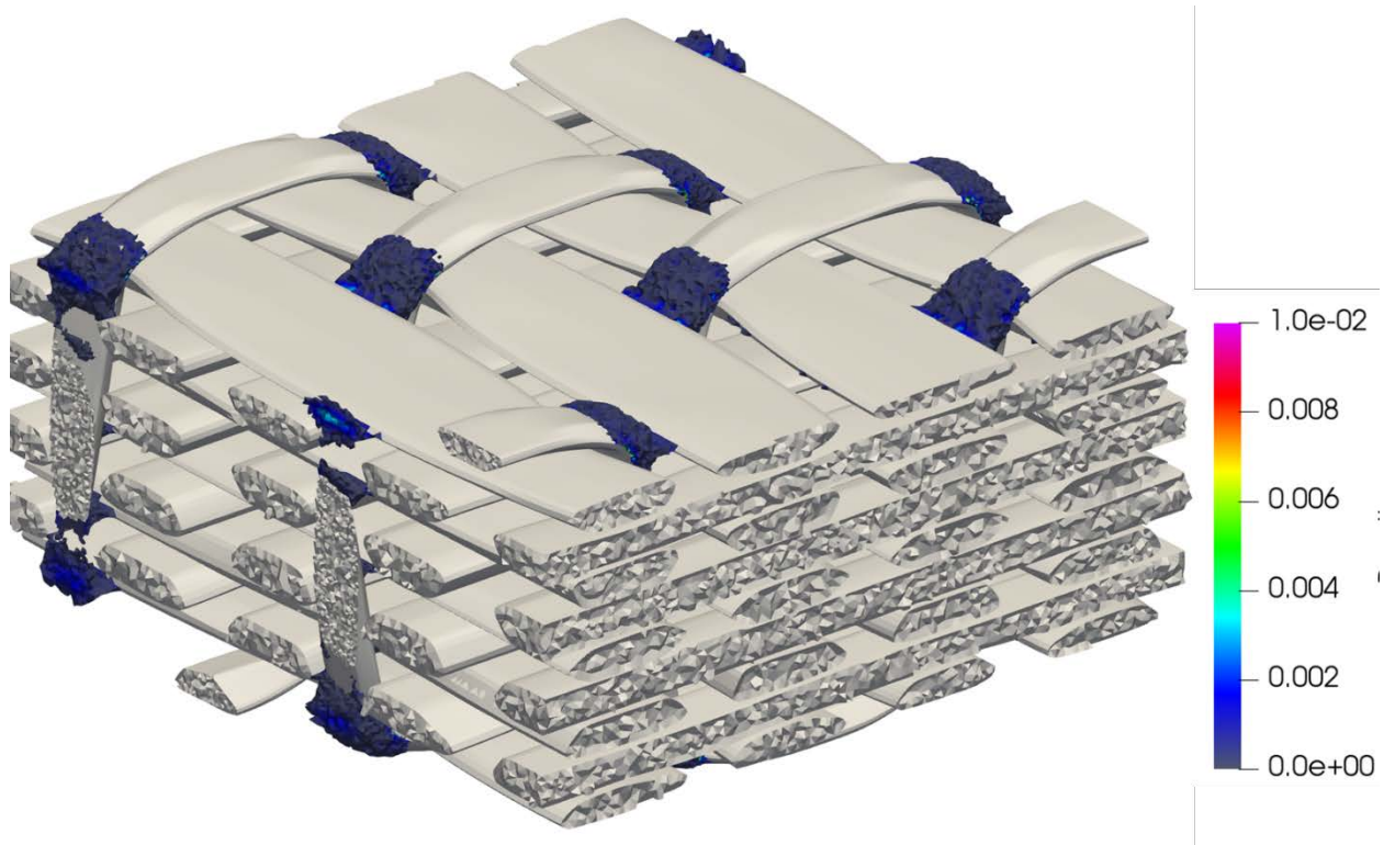
Figure 6.59. Contours of the effective plastic strain in the matrix (binders shown in gray)
