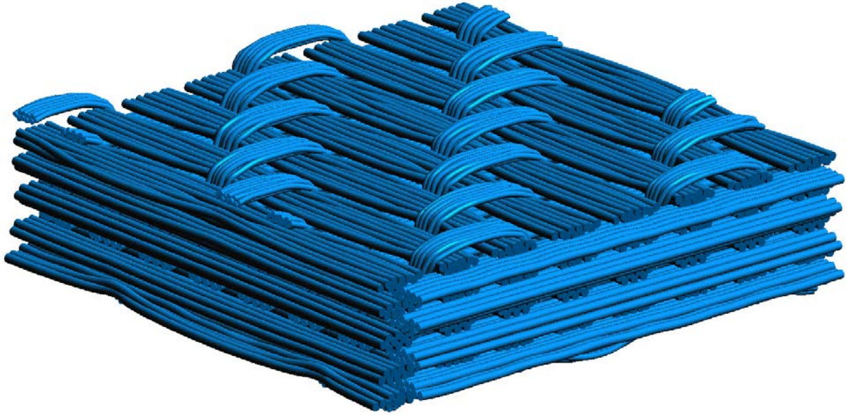
Figure 2.23. Textile model with digital chains clipped to smaller region to avoid surface meshing issues
