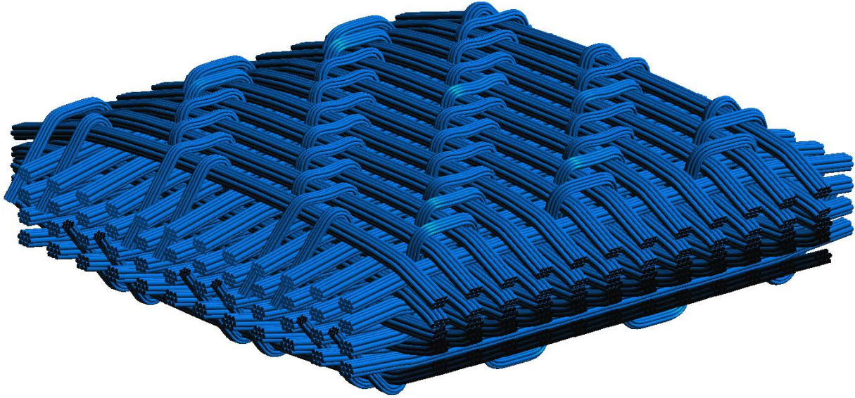
Figure 2.18. Textile model with 10 digital chains per a tow
