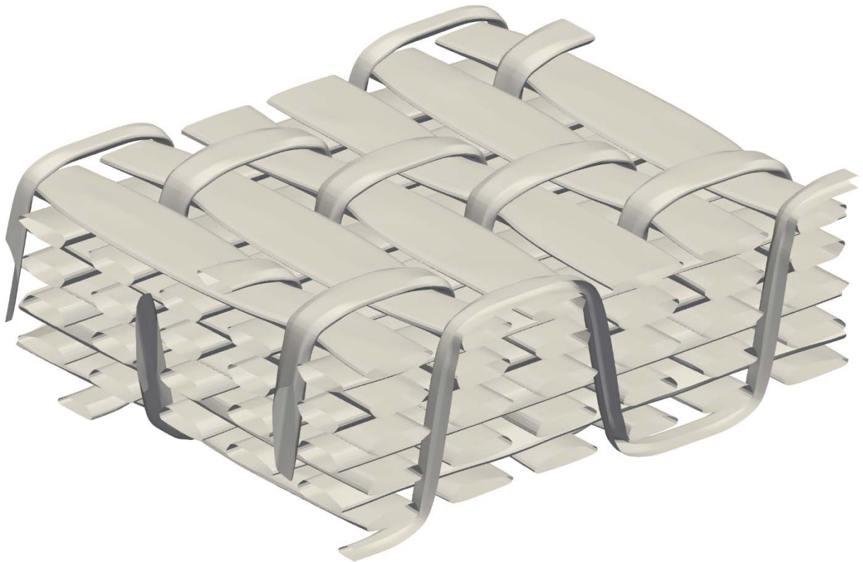
Figure 2.34. Surface meshes of tows without elements that lie on the textile boundaries
