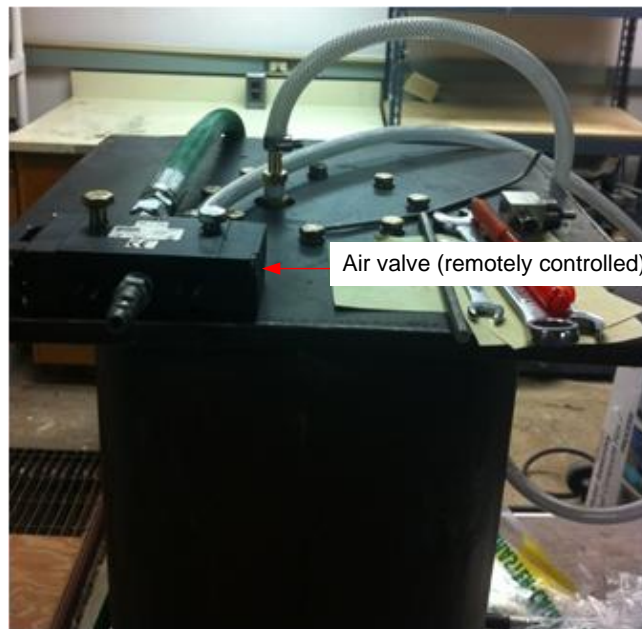
Figure 146. Top half of the ignition test rig
