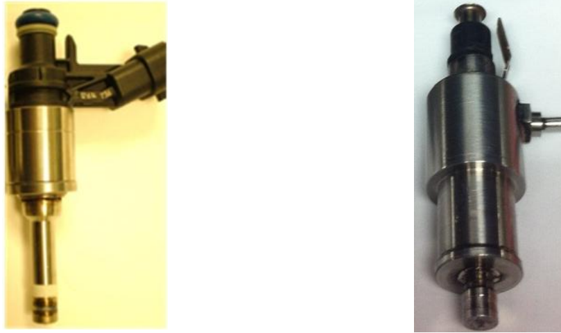
Figure 121. Direct fuel injector before (left) and after (right) modified (Proprietary. Texas A&M. Patent pending)
