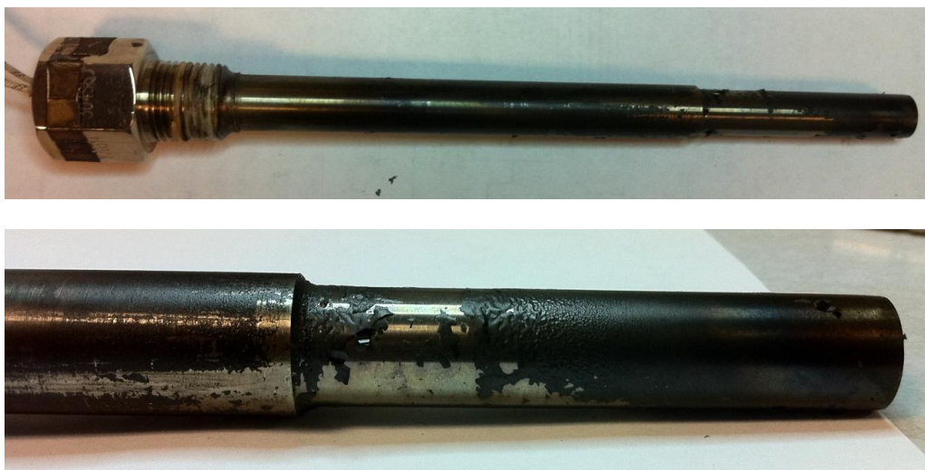
Figure 15. Thermowell is surrounded by carbonized JP-8 fuel
