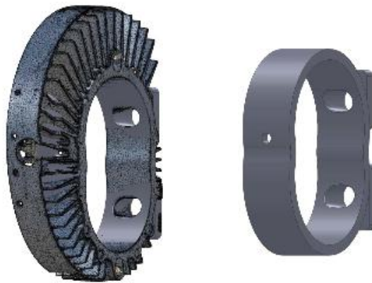
Figure 156. Scanned Wankel engine housing
