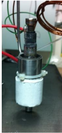
Figure 122. Heated fuel injector assembly (Proprietary. Texas A&M. Patent pending)
