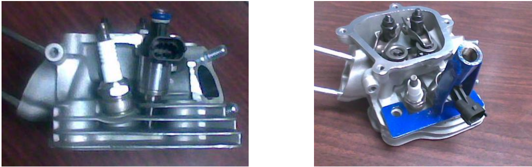
Figure 4. Modified piston head to include direct fuel injector
