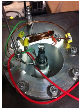
Figure 122. Heated fuel injector assembly (Proprietary. Texas A&M. Patent pending)
