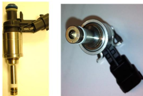
Figure 16. BOSCH direct fuel injector used in this study
