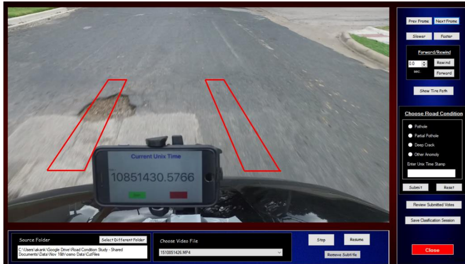
Figure 14. Road Condition Classifier Software with Tire-Trajectory Overlay
