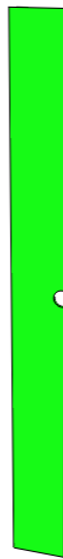
Figure 5.10: Notched plate utilized to study combined effects of stress redistribution and damage evolution during cyclic thermal actuation.
