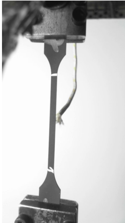
Figure 4.4: Actuation fatigue dogbone loaded within test frame for monitoring the evolution of the effective modulus
