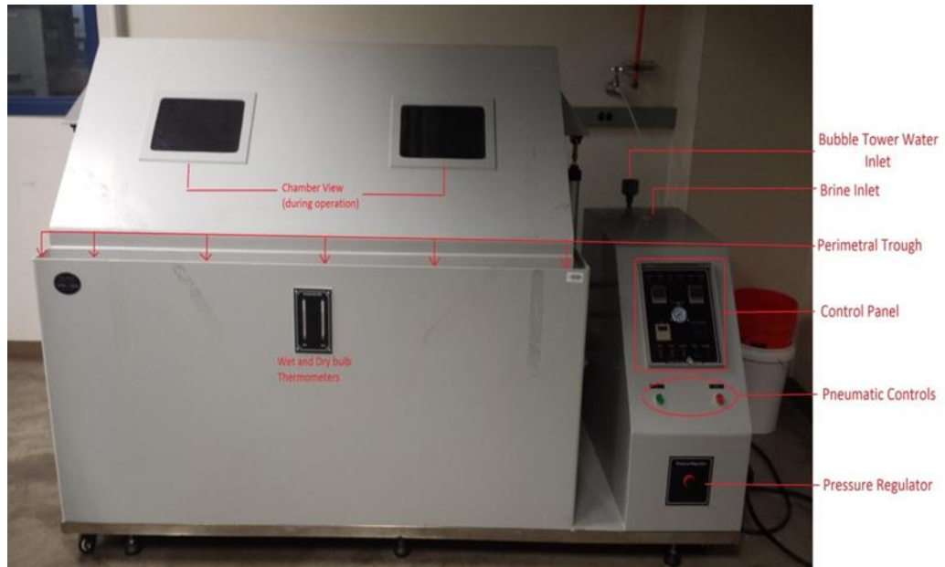
Figure 9. Salt spray equipment exterior view.
