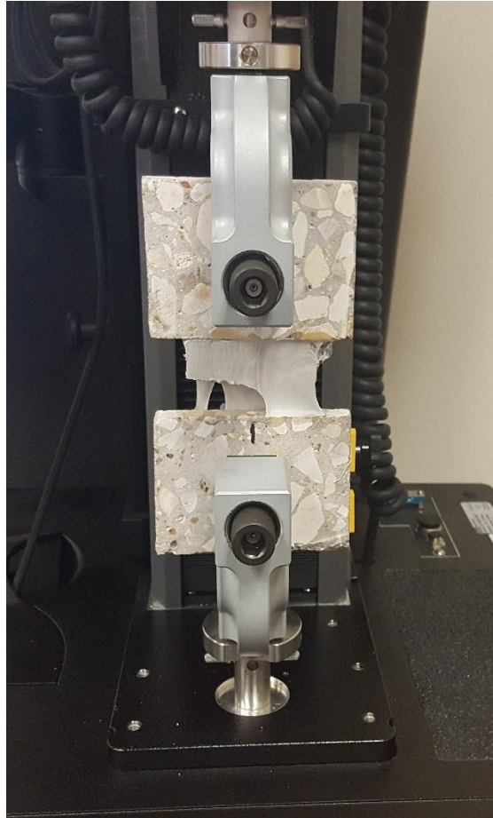
Figure 41 - Tensile bond testing with Instron Tensile meter
