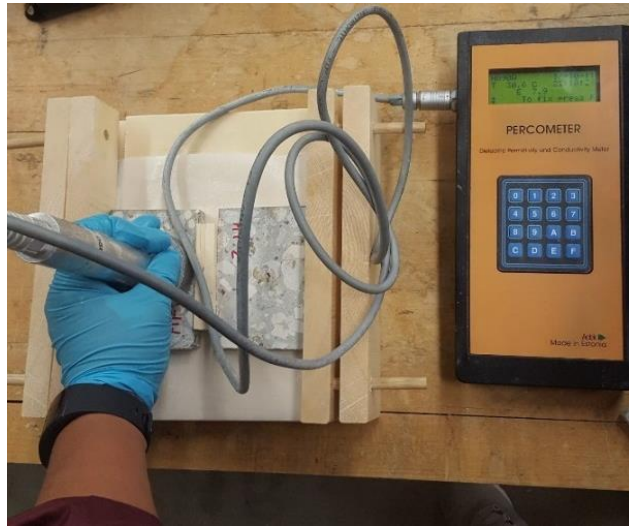
Figure 29- Dielectric measurement through Percometer
