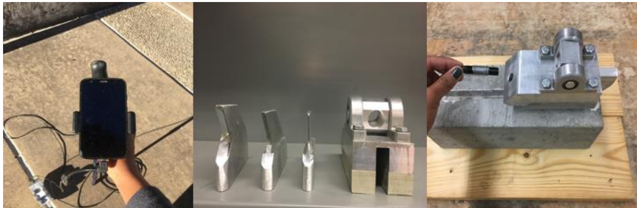
Figure 6- Joint inspection assembly
