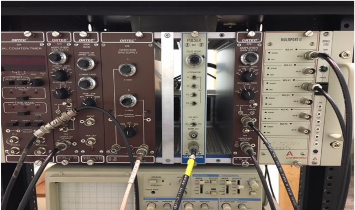
Figure 3.6 The signal processing system: Amplifier, high voltage supply, and MCA.
