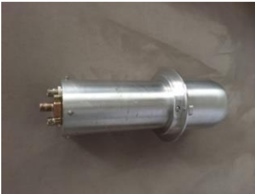
Figure 3.2 Cylindrical aluminum mounting base connected to detector
