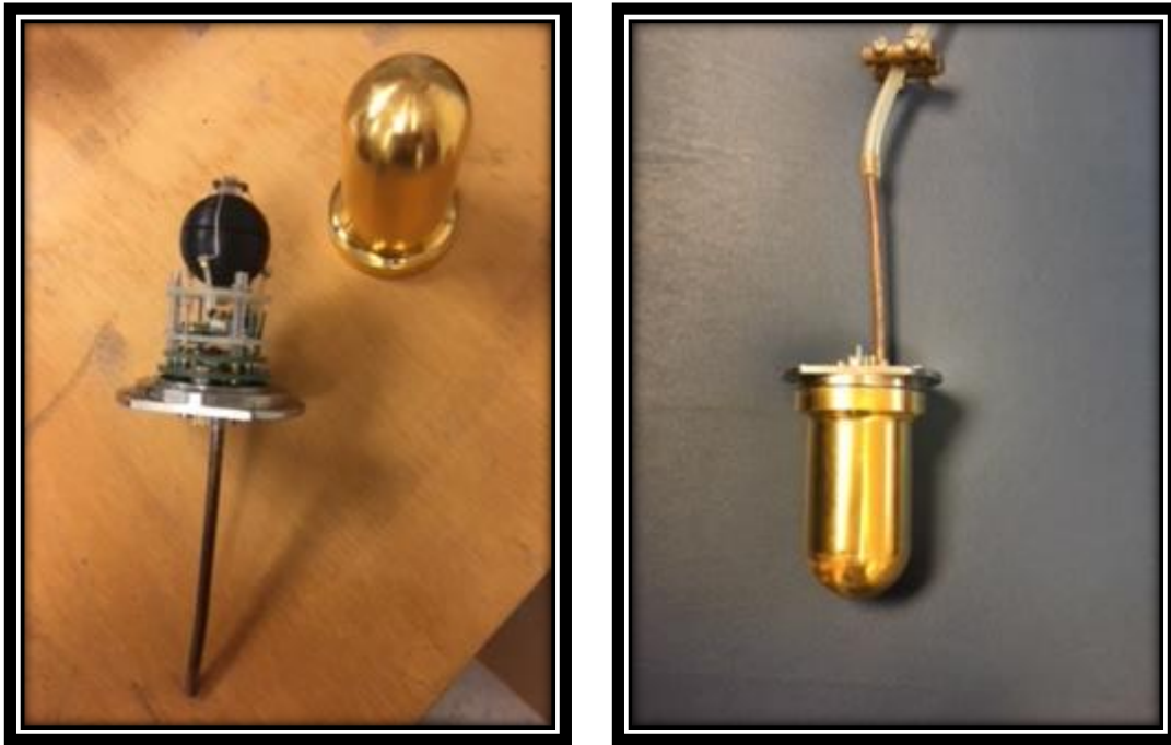
Figure 3.3 TEPC 1.8 cm detector assembly (left) attached to preamplifier circuit board enclosed in gold-plated vacuum chamber (right).
