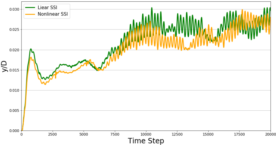
Figure 60 In-Line Motions at Mudline, Nonlinear SSI
