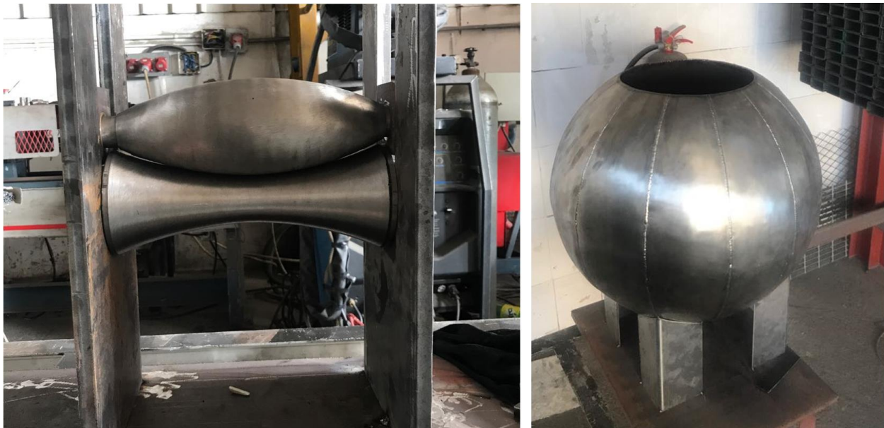
Figure 23. Photos of the manufactured solar heater for the pilot testing
