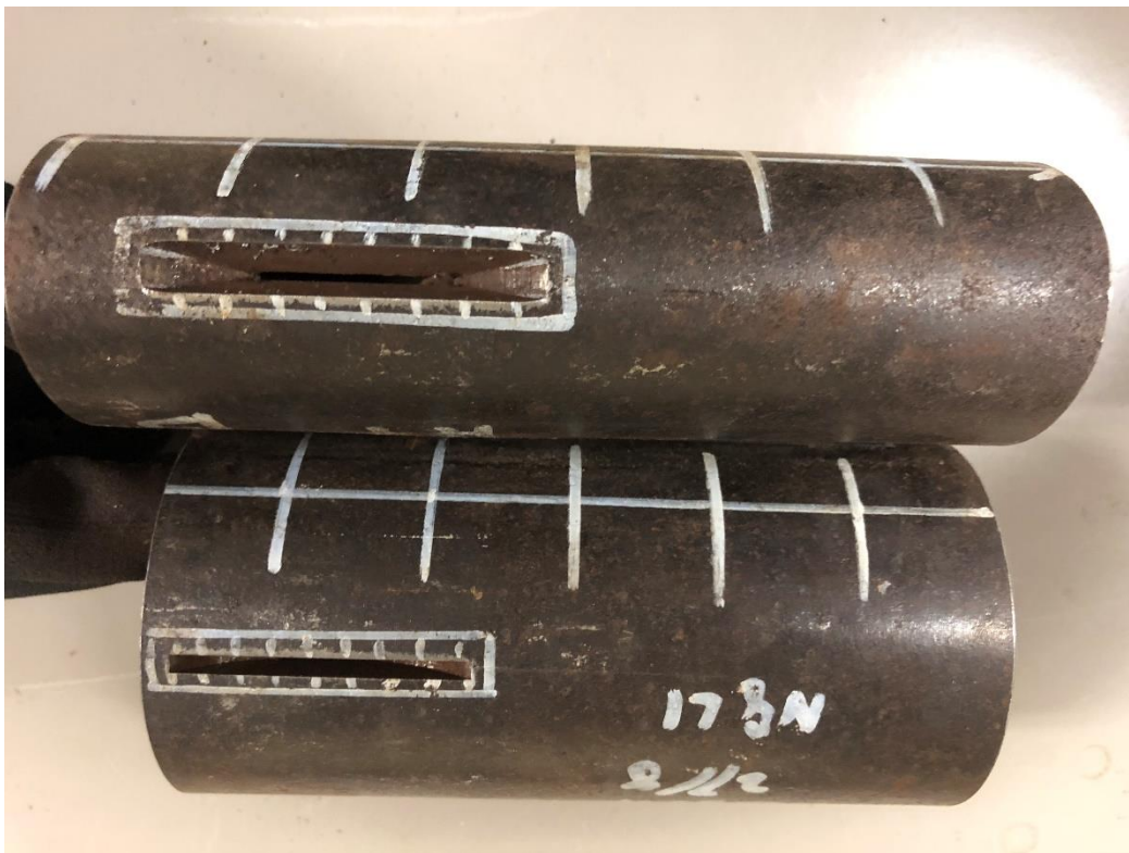
Figure 49 Slot opening on the side of the load comparing with original slot
