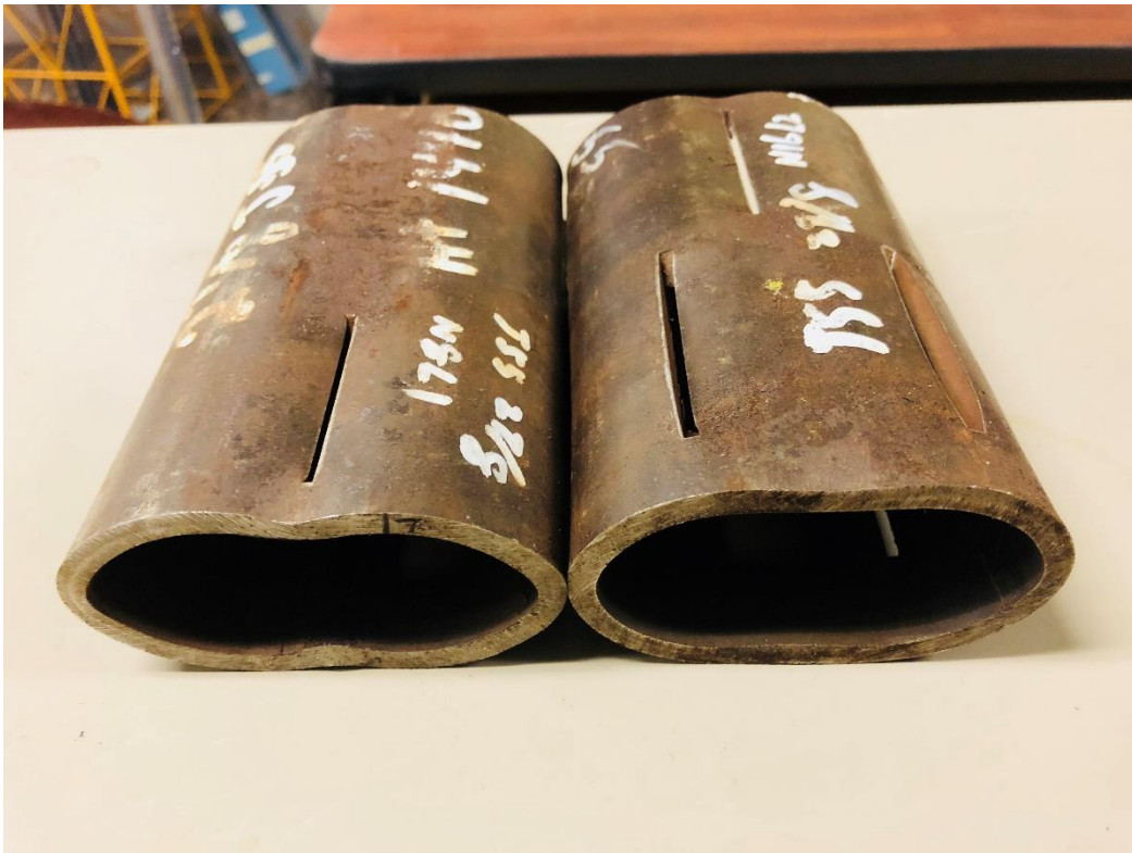
Figure 46 2 7/8" J55 samples after line load test
