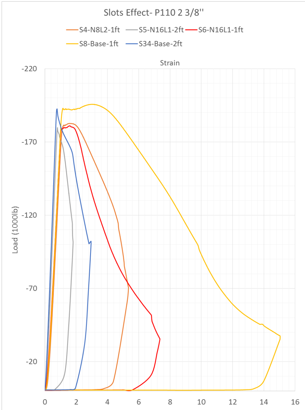
Figure 62 Slot pattern effect on 2 3/8" P110 slotted liners
