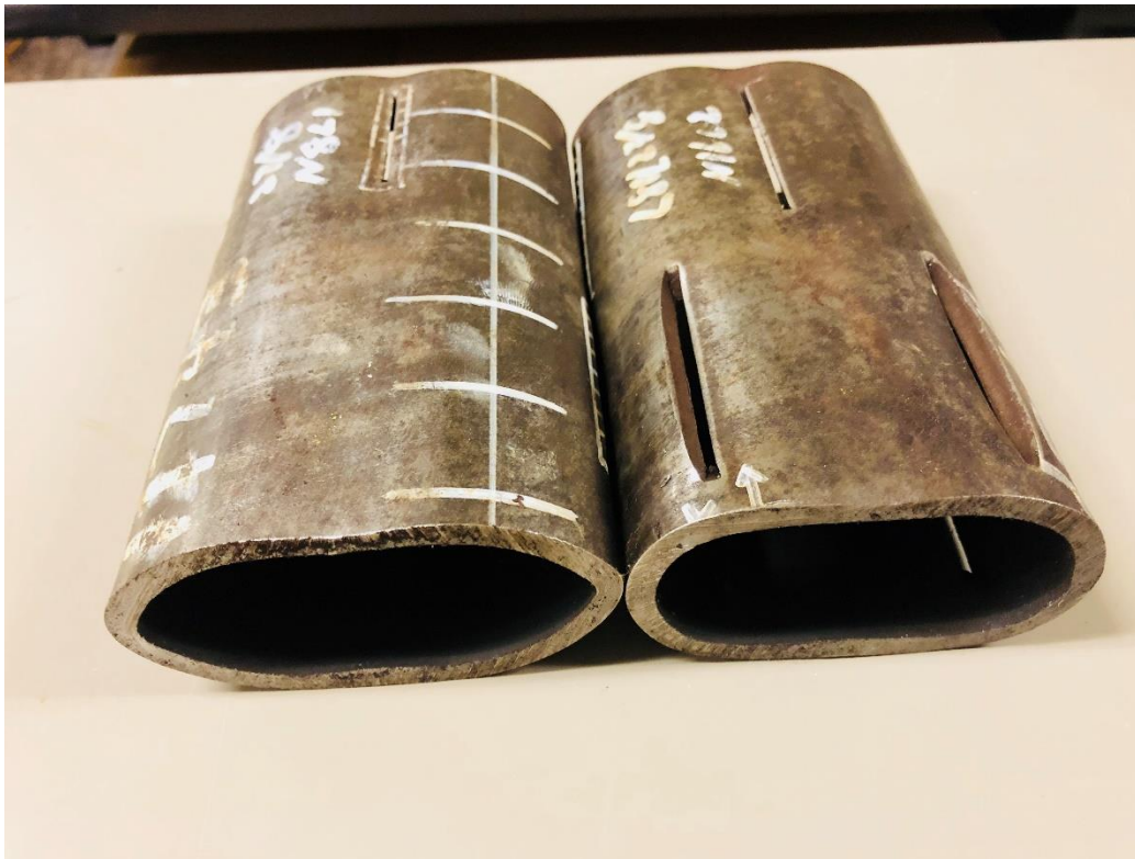
Figure 47 2 7/8" thin wall L80 samples after line load test
