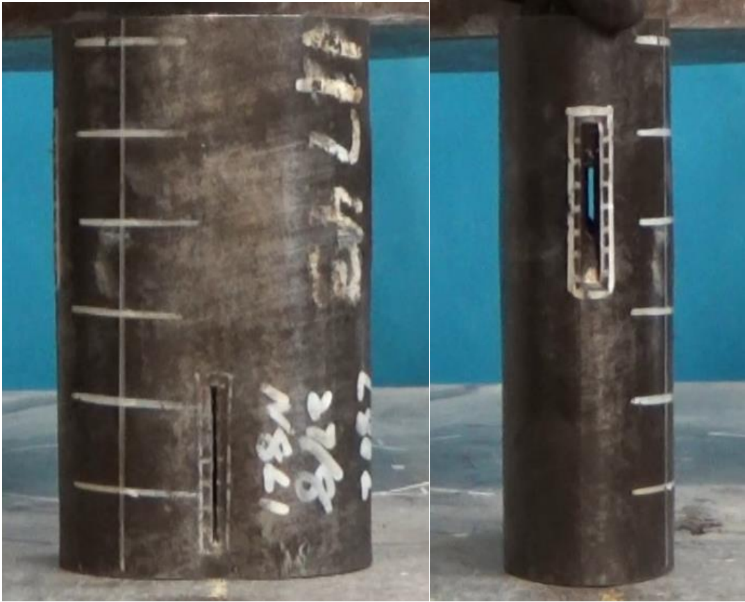
Figure 51 Experiment: slot deformation after line load collapse test. Load direction on the left, horizontal cross-section on the right.
