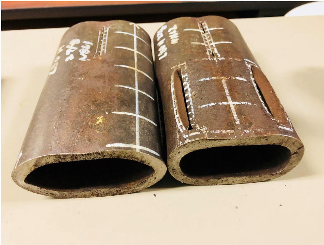
Figure 48 2 7/8" L80 thick wall samples after line load test
