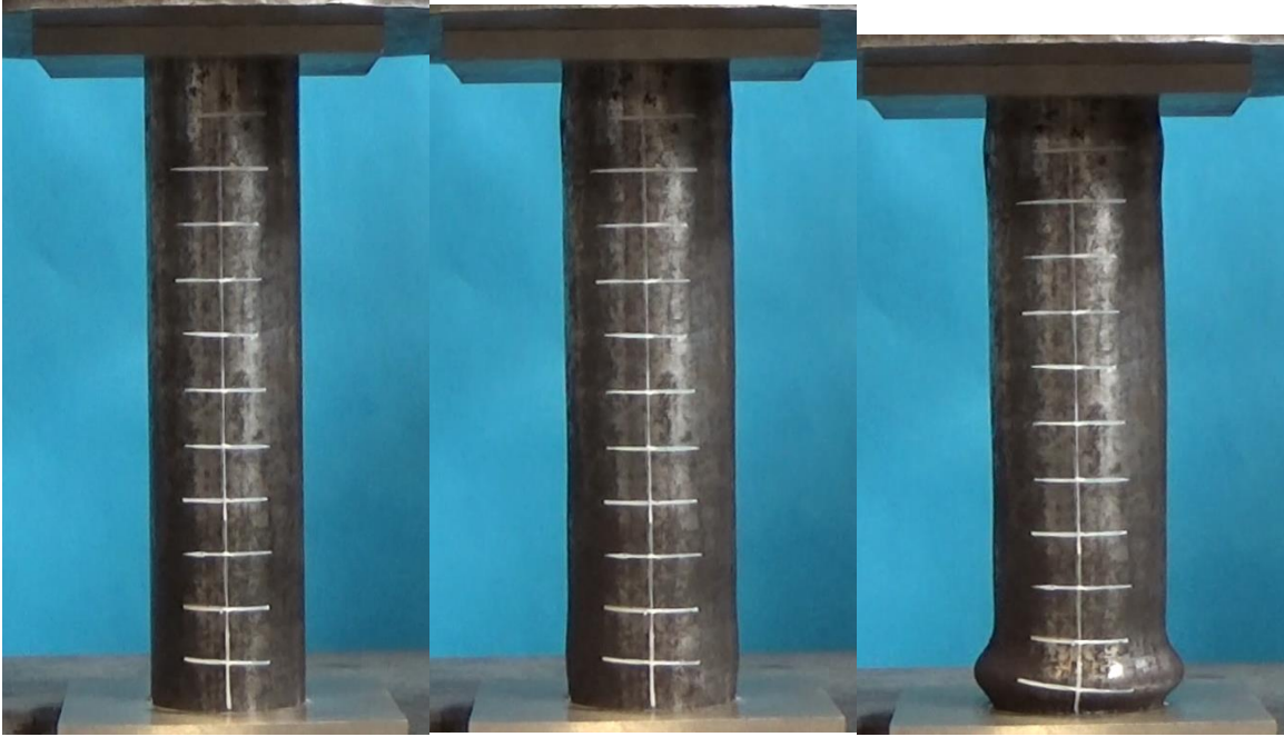
Figure 40 2 7/8" light L80 at yield point, peak strength, 10% axial strain
