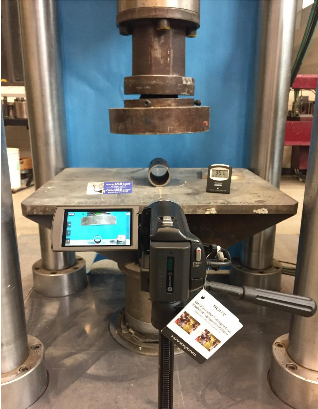
Figure 45 Experimental setup for line load test
