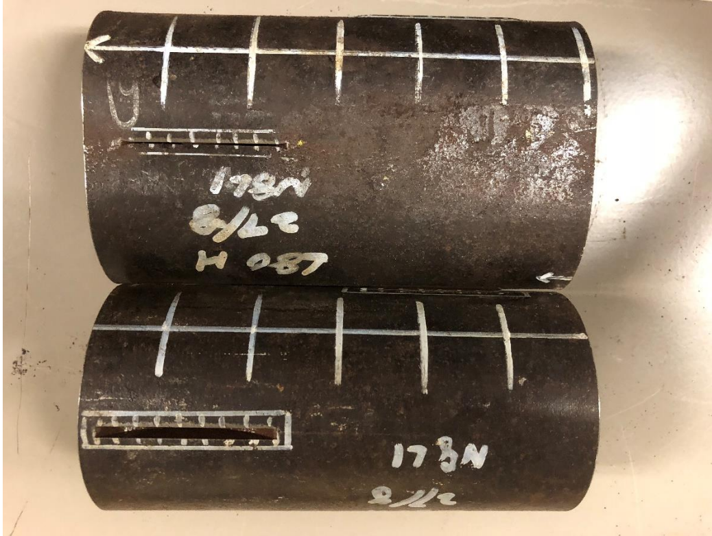
Figure 50 Slot closing under the load on the loading direction comparing with original slot
