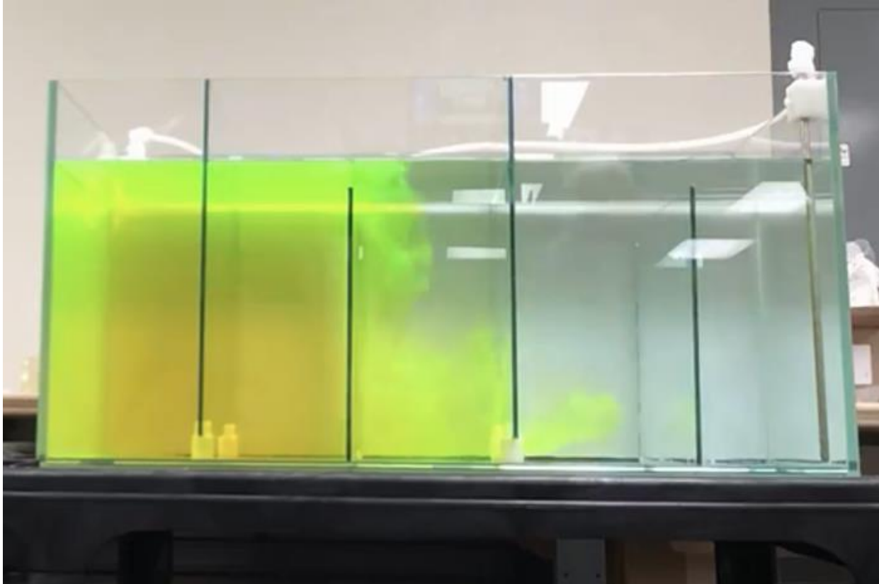
Figure 2: Demonstrating the baffled circulation tank that were used to mix the oil, Corexit, and natural microbial communities for each treatment.
