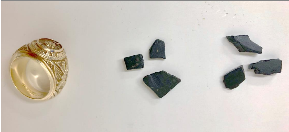
Fig. 23 – Generated Rock Chip Samples and the Size Comparison (From Left to Right: Size 8.5 Aggie Ring, WT CR Rock Chips, and WT QR Rock Chips)
