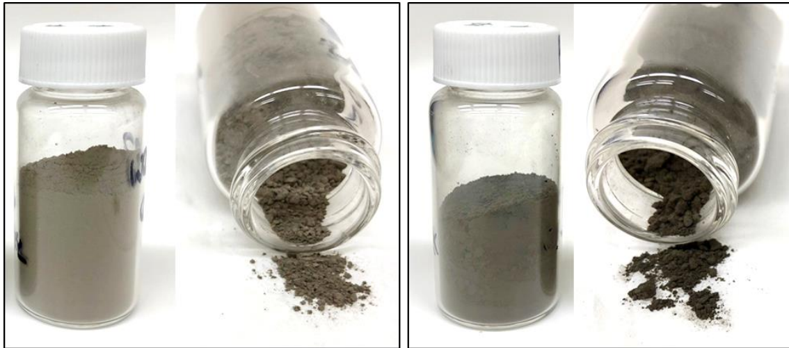
Fig. 17 – Crushed Rock Particles for Zeta Potential Measurement: WT CR (Left) and WT QR (Right)
