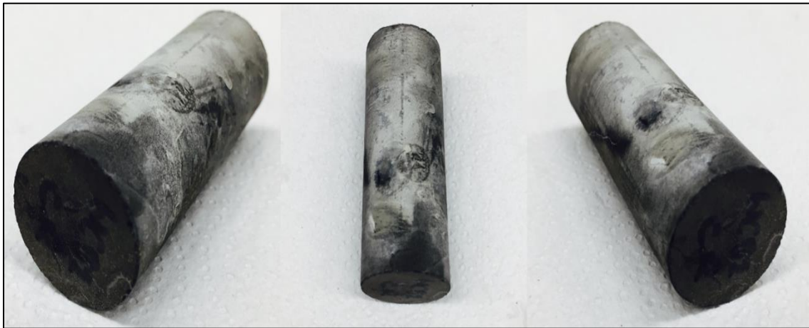
Fig. 128 – Observation of Scaling when Using Fluids with High Salinity
