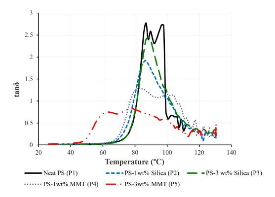
Figure 14 tand as a function of temperature for polystyrene and polystyrene nanocomposites
