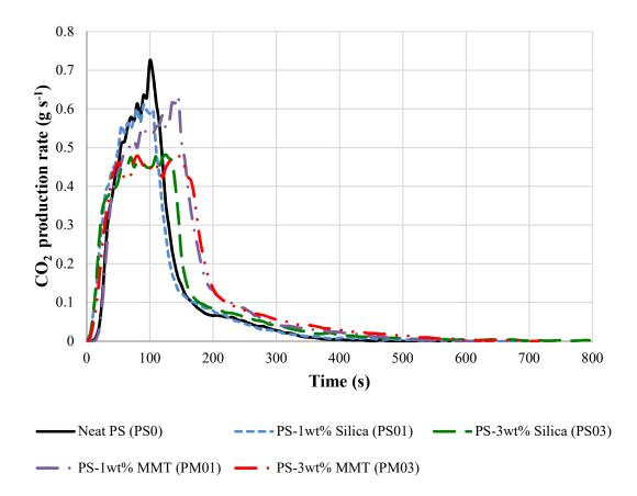
Figure 23 CO<sub>2</sub> production rate with respect to time for neat polystyrene and polystyrene nanocomposites
