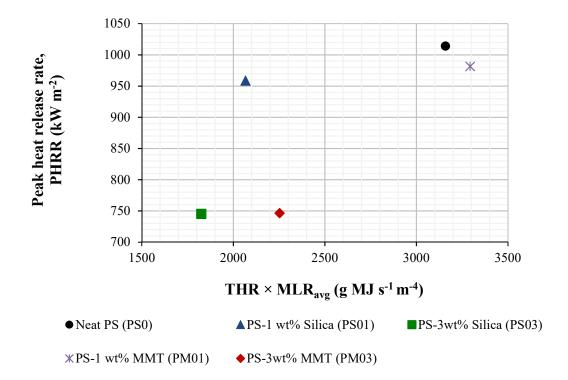
Figure 24 Peak heat release rates, PHRR (kWm<sup>-2</sup>) with respect to THR  $\times$  MLR<sub>avg</sub> (g MJ s<sup>-1</sup> m<sup>-4</sup>) for fire performance evaluation of polystyrene and polystyrene nanocomposites
