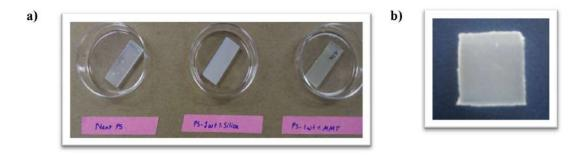
Figure 7 Polystyrene nanocomposites: a) 36 mm × 10 mm × 3.25 mm sample prepared for dynamic mechanical analysis and b) square 1 mm × 1mm sample made for nanoindentation
