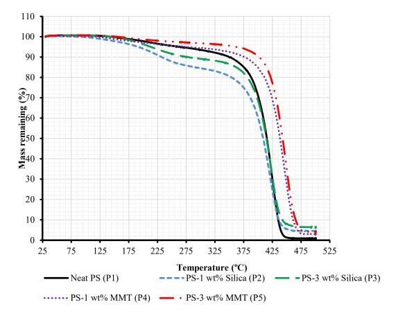
Figure 8 Thermogravimetric analysis curves for neat polystyrene and polystyrene nanocomposites
