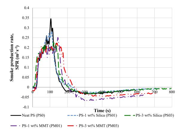
Figure 21 Smoke production rate (SPR) for the neat polystyrene and polystyrene nanocomposites
