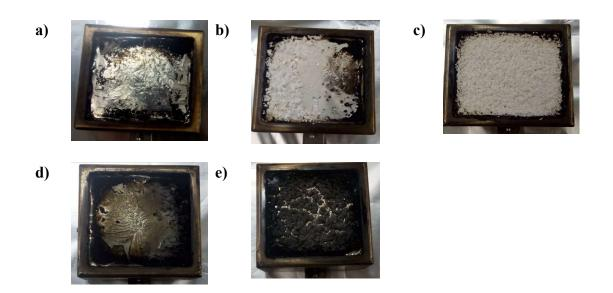
Figure 20 Images of polystyrene and polystyrene nanocomposites residue after cone calorimeter test (heat flux = 50 kWm<sup>-2</sup>, horizontal setting): a) neat PS (P0), b) PS-1wt% silica (PS01), c) PS-3wt% silica (PS03), d) PS-1wt% MMT (PM01), and e) PS-3wt% MMT (PM03)
