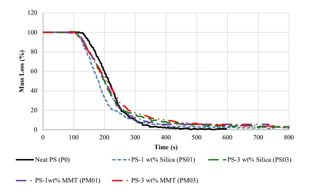
Figure 18 Mass loss data for polystyrene and polystyrene nanocomposites
