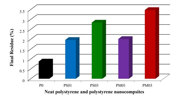
Figure 19 Char turnout for polystyrene and polystyrene nanocomposites
