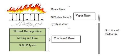
Figure 2 Physical heat-induced decomposition behaviors for non- charring polymers
