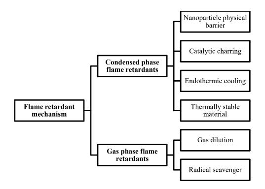
Figure 1 Classification of flame retardant additives based on the flame-retardant mechanism
