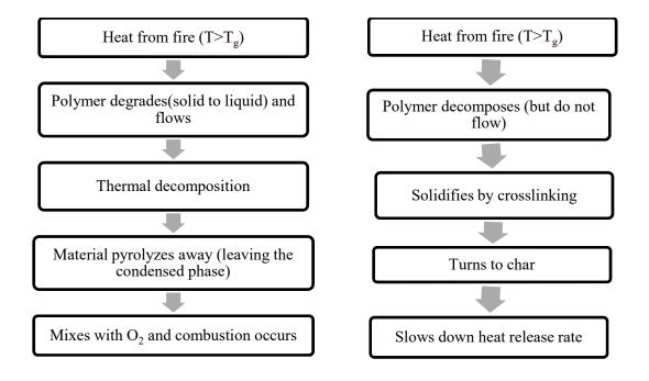
Figure 4 Flowchart showing steps of non-charring (left) and charring mechanism (right)
