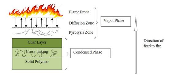
Figure 3 Physical heat-induced decomposition behaviors for charring polymers
