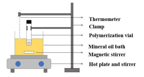
Figure 6 Schematic experimental setup for *in-situ* polymerization
