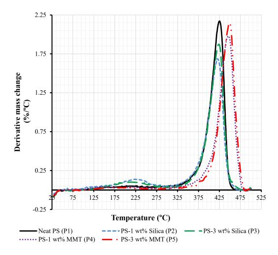
Figure 9 Derivative thermogravimetric analysis curves of neat polystyrene and polystyrene nanocomposites
