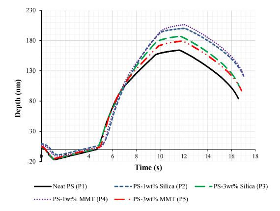
Figure 16 Depth versus time (creep data) for polystyrene and polystyrene nanocomposites
