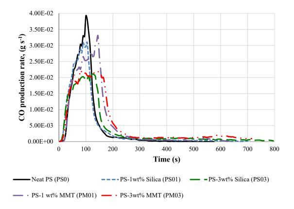
Figure 22 CO production rate with respect to time for neat polystyrene and polystyrene nanocomposites
