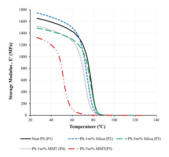
Figure 12 Storage modulus (E') as a function of temperature for polystyrene and polystyrene nanocomposites
