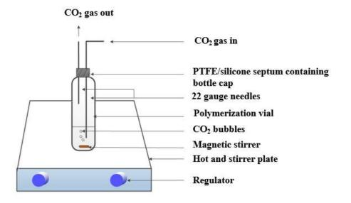
Figure 5 Schematic setup for inerting monomer solution
