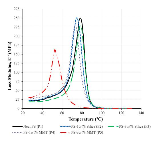
Figure 13 Loss modulus (E") as a function of temperature for polystyrene and polystyrene nanocomposites
