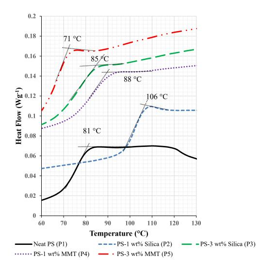
Figure 11 Heat flow versus temperature plot using differential scanning calorimetry
