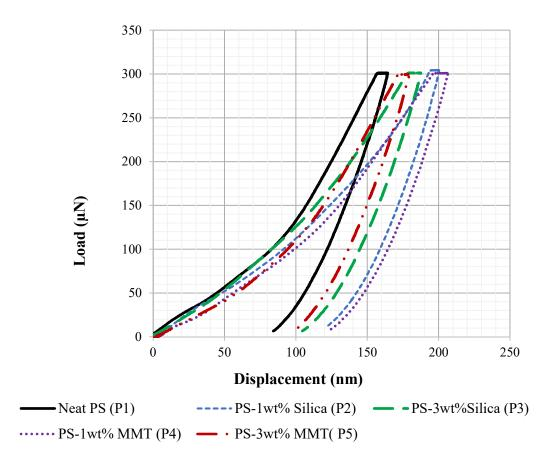
Figure 15 Load displacement data for polystyrene and polystyrene nanocomposites at room temperature
