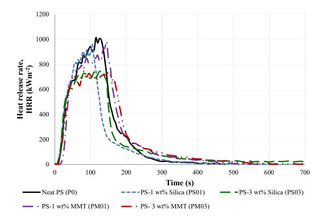
Figure 17 Heat release rate (HRR) with respect to time for neat polystyrene and polystyrene-nanocomposites at external heat flux =  $50 \text{ kWm}^{-2}$
