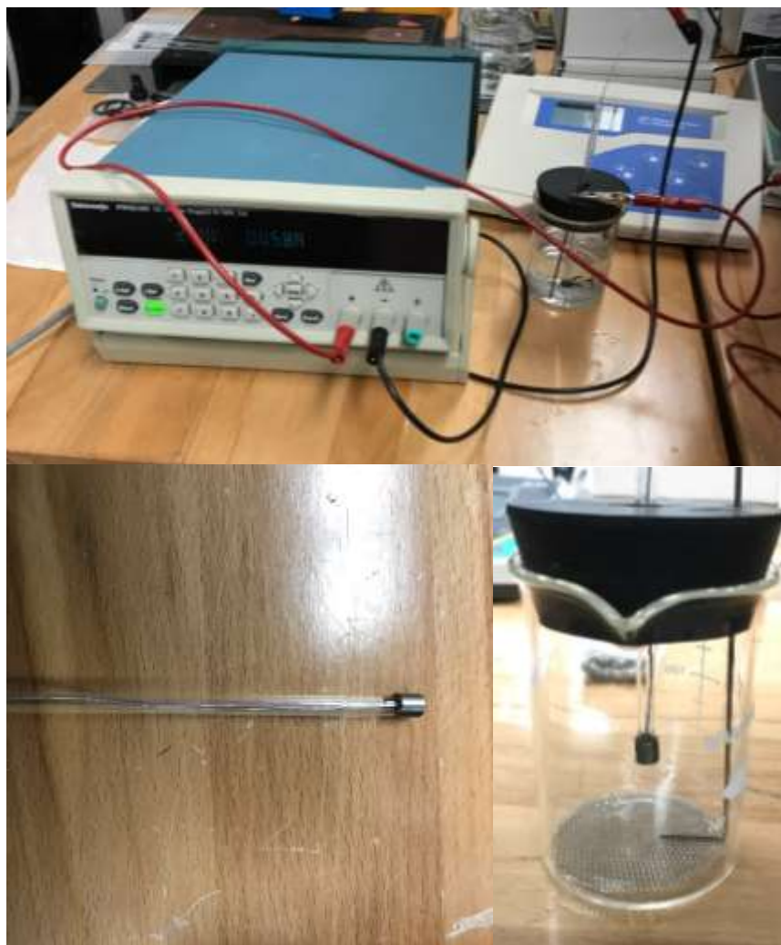
Figure 3: (Top) The electrochemical cell assembly powered by PWS 1825. \text{H}_2\text{SO}_4 solution fills the beaker to 100 mL ensuring proper submergence of the sample (Left) Sample-tubing assembly with connection made to steel sample. (Right) Electrochemical cell
