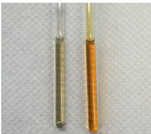
Figure II-1. Photograph of J. Young tubes for entries 3, Table II-1 (right) and 6, Table II-2 (left) after 1 day. A drop of Mercury can be seen in the left tube. The right tube has changed to a red/orange color indicating the presence of Pd nanoparticles.
