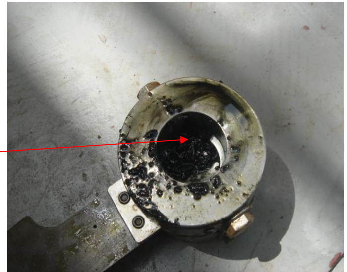
Outboard dry gas seal 1st leak line rupture disk was found ruptured and full of debris.
