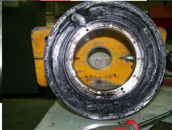
Outboard DGS 2nd seal, broken tungsten carbide pieces.
