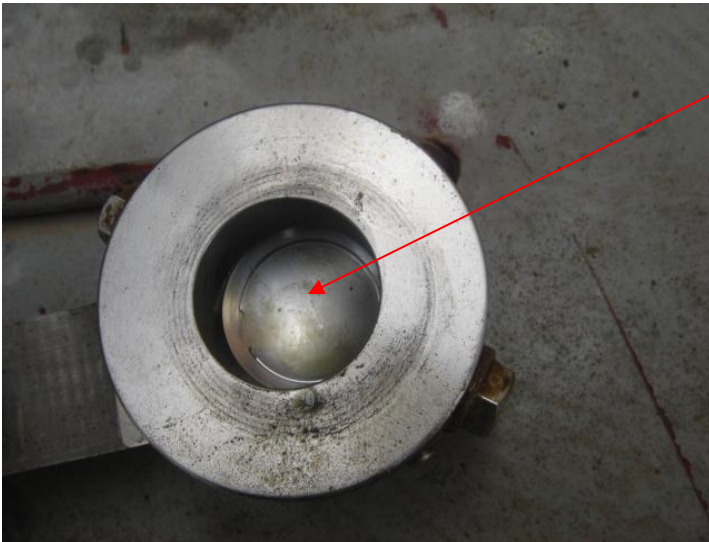
Outboard dry gas seal 1st leak line rupture disk was found ruptured and full of debris.
