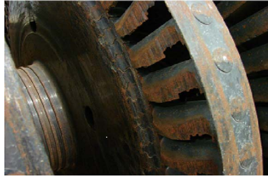
Figure 2 - Severe damage of Row #4 Blades
