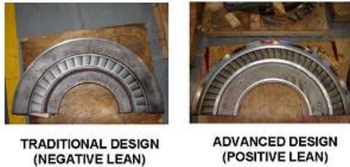
Figure 15 - Diaphragms with Different Tangential Lean of the Vanes
