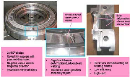
Figure 56 - Deficiencies of Obsolete 2 x 180 Degree Diaphragm Fabricated by Sub-Arc Welding
