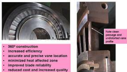
Figure 57 - Advantages of Current 1 x 360 Degree Diaphragm Fabricated by EB Welding with EDM-Wire Cutting
