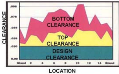
Figure 36 - Wear Pattern of Standard Shaft Seals
