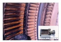
Figure 44 Deposit Condition of LP Section
