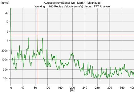
Left: Measured on the engine inboard casing in the vertical direction. Note the "picket fence" type response. Harmonics are ½ engine speed.
