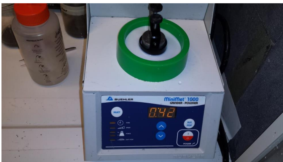
Figure 51: Final Polishing of Ion Beam Samples using the MiniMet™ 1000 and Chemical/Mechanical Polishing Slurry on Micro-Cloth
