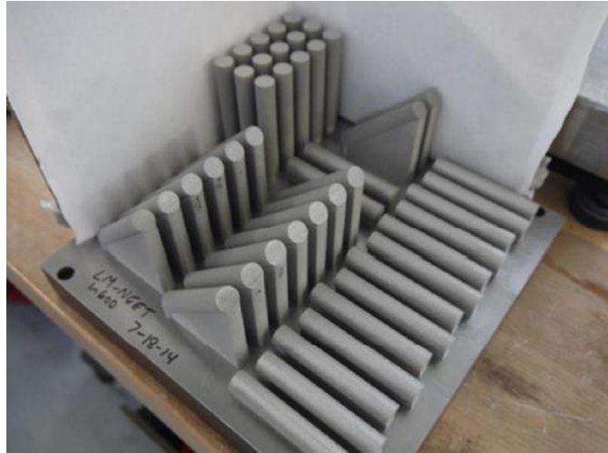
Figure 4: Vertical, Horizontal, and 45° Inconel 600 Rods Produced by LAM
