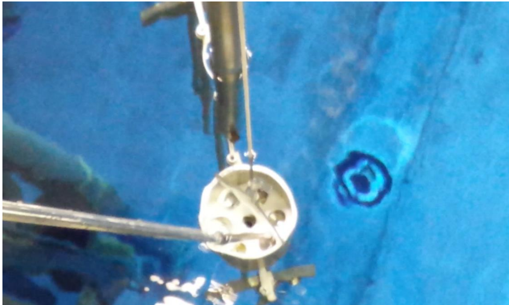
Figure 57: Tilting the Spear 30° and Rotating to Detach the Aluminum Can from the Spear, Guiding the Can into the Submerged Decay Funnel Tube
