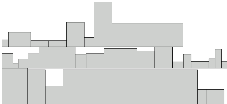
Figure 3.11: Floor plan of the CFAST model that is converted from the Revit model. All rooms are converted to cuboids.
