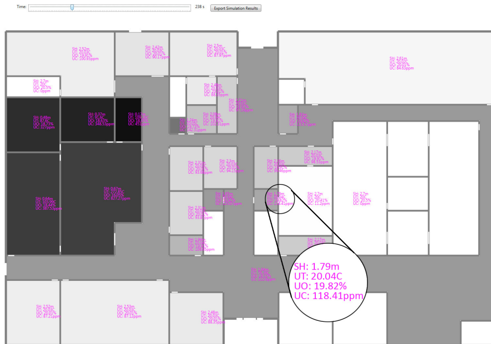
Figure 4.3: Color-coded floor plan to show smoke propagation and the information about the toxic gases.
