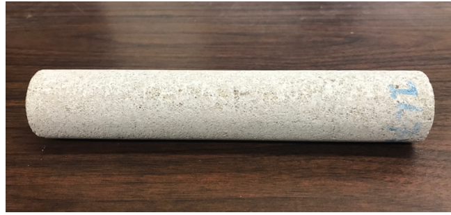
Figure 2.13 Indiana limestone core sample 1.5 inch by 8 inch
