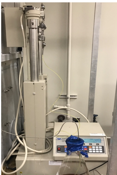
Figure 2.3 Teledyne ISCO syringe pump
