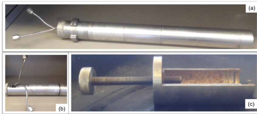
Figure 2.6 Core holder part: (a) inlet plug, (b) outlet plug, (c) inlet cap
