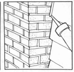
between 45° F and 55° F. At these temperatures expansion and contraction at joints are at a midway point.
