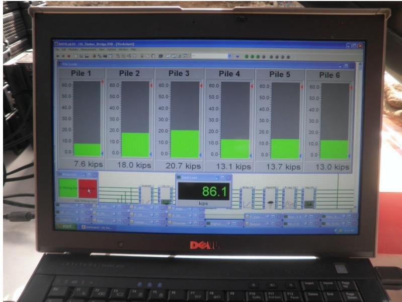
Figure 4. Laptop displaying load data during testing of the timber railroad bridge
