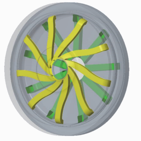
Figure 10: Pitot tube capacity curves; rotor cover (yellow) and rotor channels (green) reduce slip
