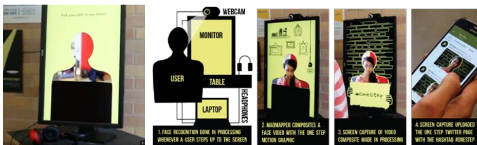
Figure 1: One Step Interactive Poster One: Installation setup, technical diagram, and social media connection (twitter)
