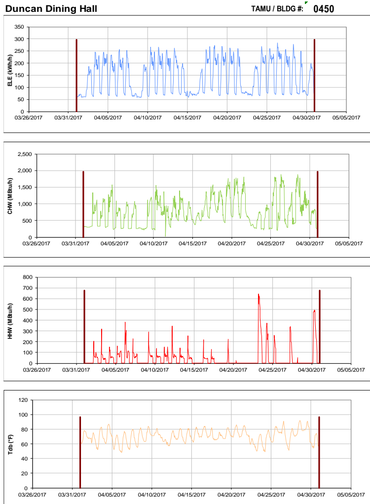
Figure III-73 Hourly Whole Building Electricity, Chilled Water, and Hot Water Consumption for Duncan Dining Hall during the Month of April 2017 and the Corresponding Hourly Outdoor Dry Bulb Temperature for College Station, TX
