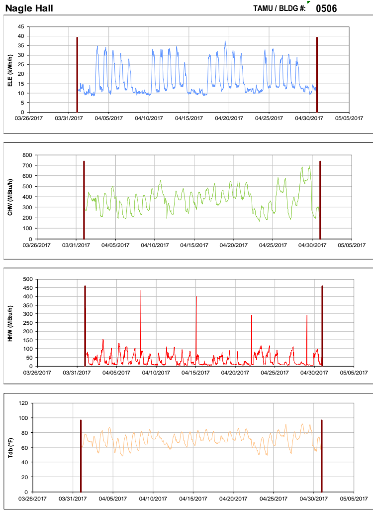
Figure III-103 Hourly Whole Building Electricity, Chilled Water, and Hot Water Consumption for Nagle Hall during the Month of April 2017 and the Corresponding Hourly Outdoor Dry Bulb Temperature for College Station, TX
