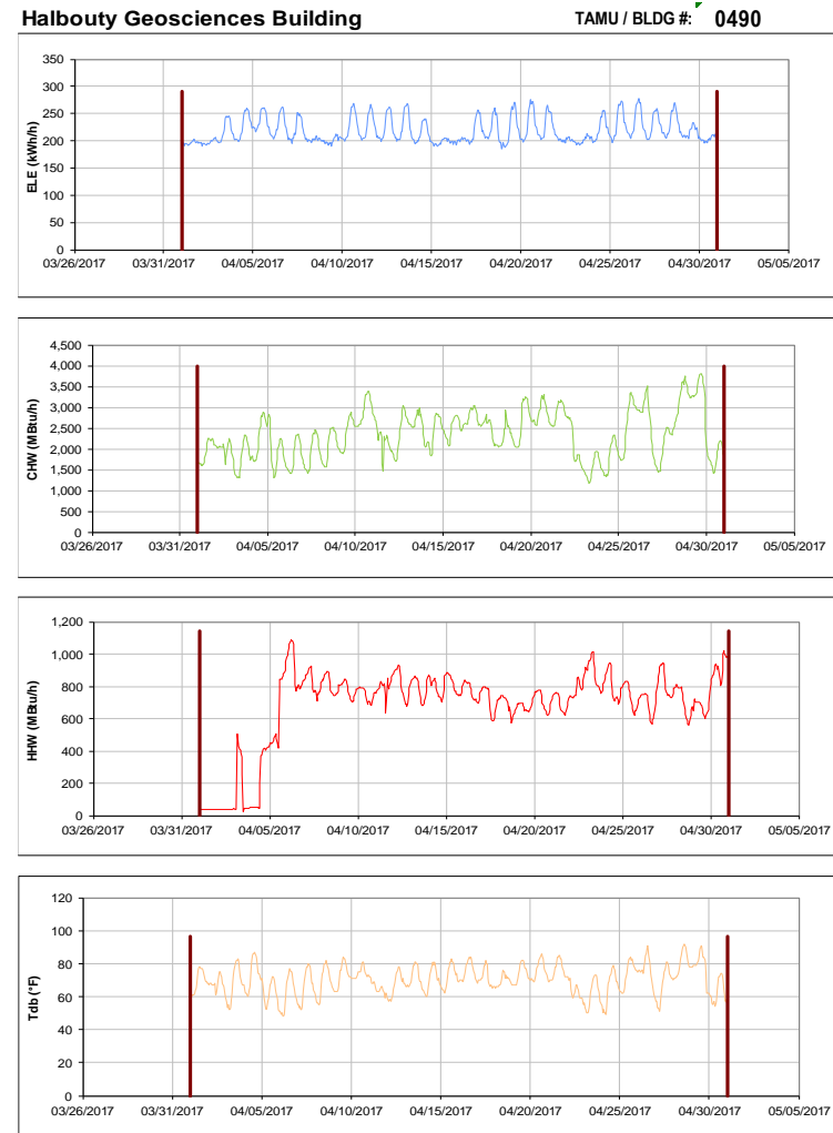
Figure III-98 Hourly Whole Building Electricity, Chilled Water, and Hot Water Consumption for Halbouty Geosciences Building during the Month of April 2017 and the Corresponding Hourly Outdoor Dry Bulb Temperature for College Station, TX
