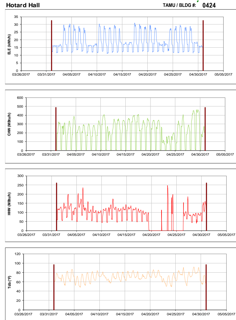
Figure III-46 Hourly Whole Building Electricity, Chilled Water, and Hot Water Consumption for Hotard Hall during the Month of April 2017 and the Corresponding Hourly Outdoor Dry Bulb Temperature for College Station, TX
