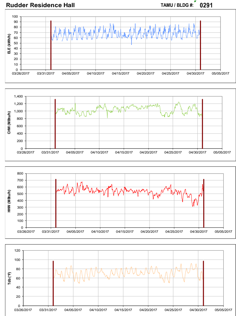
Figure III-4 Hourly Whole Building Electricity, Chilled Water, and Hot Water Consumption for Rudder Residence Hall during the Month of April 2017 and the Corresponding Hourly Outdoor Dry Bulb Temperature for College Station, TX
