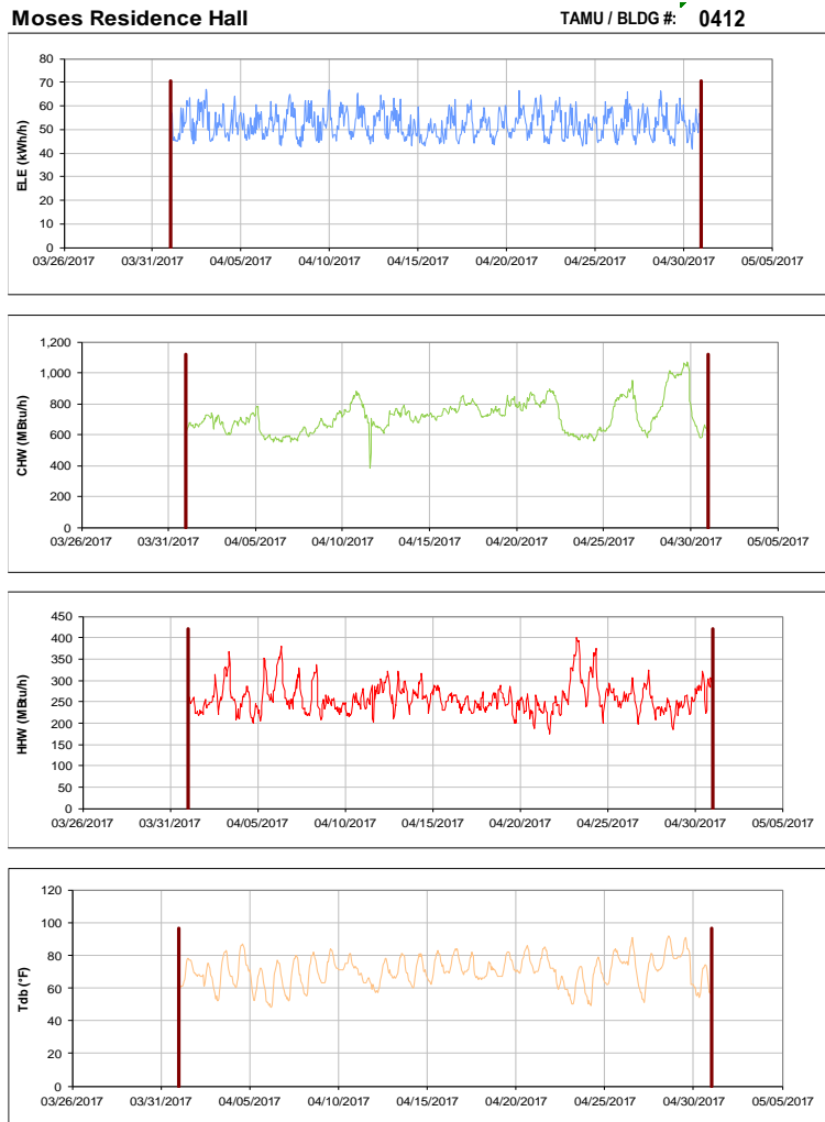
Figure III-41 Hourly Whole Building Electricity, Chilled Water, and Hot Water Consumption for Moses Residence Hall during the Month of April 2017 and the Corresponding Hourly Outdoor Dry Bulb Temperature for College Station, TX
