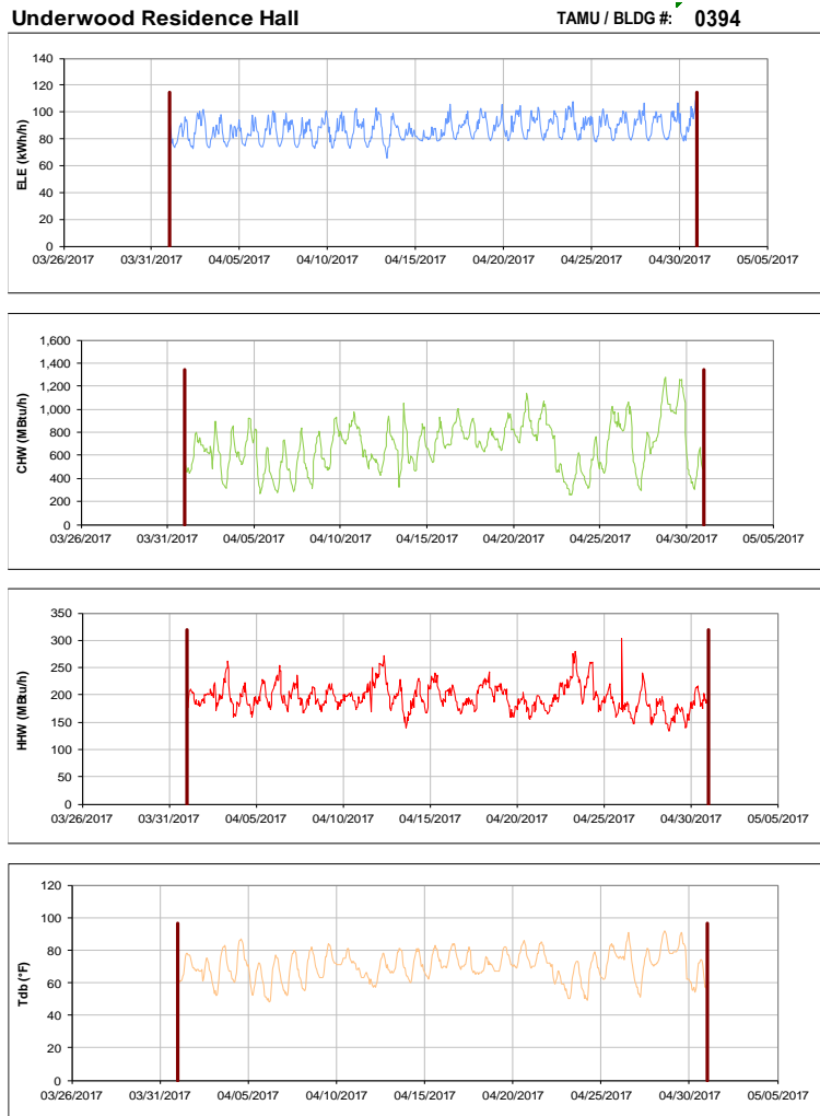
Figure III-23 Hourly Whole Building Electricity, Chilled Water, and Hot Water Consumption for Underwood Residence Hall during the Month of April 2017 and the Corresponding Hourly Outdoor Dry Bulb Temperature for College Station, TX
