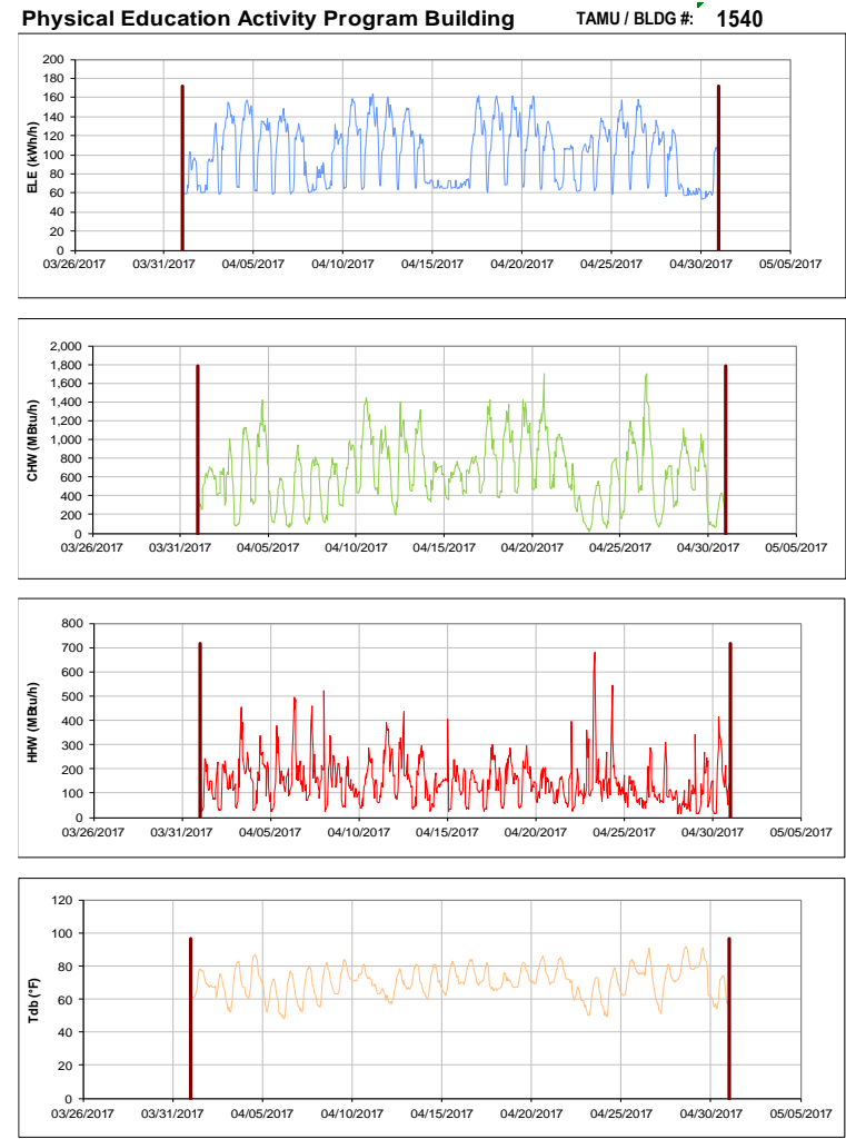
Figure III-170 Hourly Whole Building Electricity, Chilled Water, and Hot Water Consumption for Physical Education Activity Program Building during the Month of April 2017 and the Corresponding Hourly Outdoor Dry Bulb Temperature for College Station, TX
