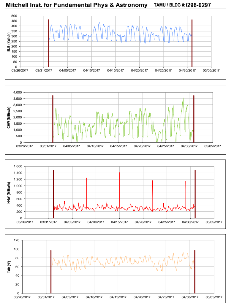
Figure III-8 Hourly Whole Building Electricity, Chilled Water, and Hot Water Consumption for Mitchell Inst. for Fundamental Phys & Astronomy during the Month of April 2017 and the Corresponding Hourly Outdoor Dry Bulb Temperature for College Station, TX
