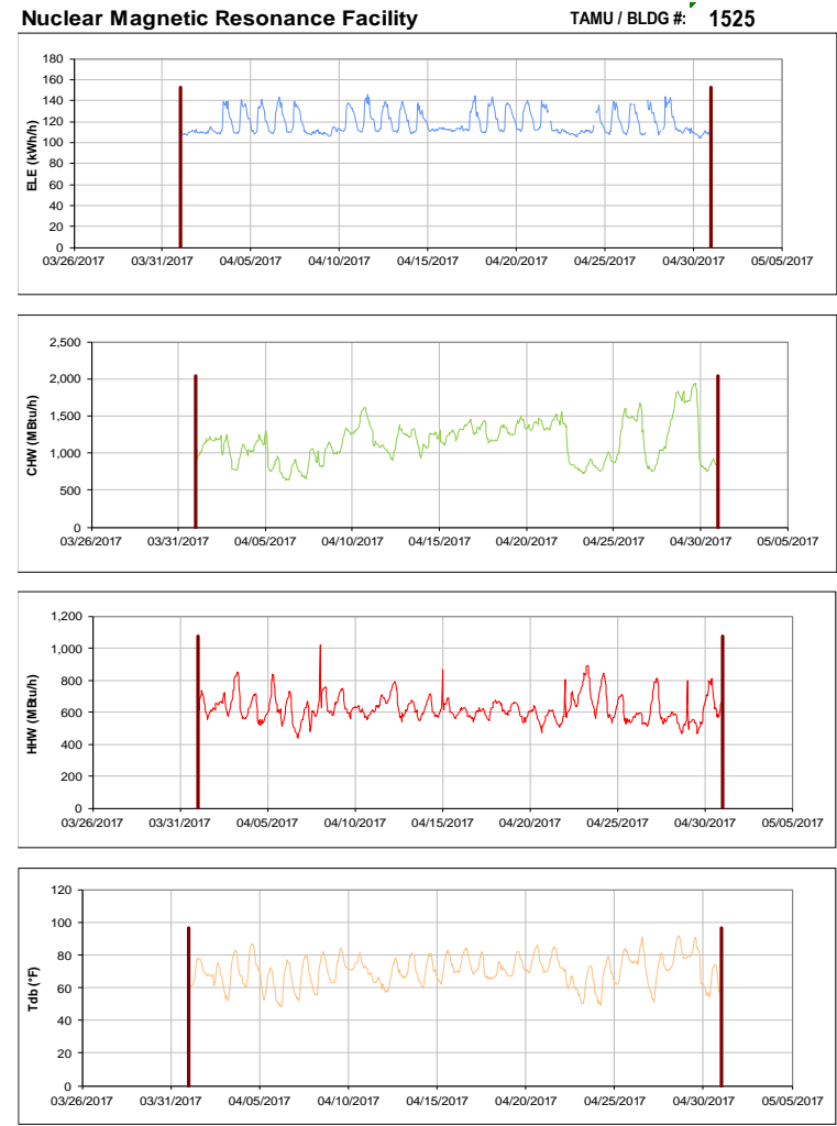
Figure III-164 Hourly Whole Building Electricity, Chilled Water, and Hot Water Consumption for Nuclear Magnetic Resonance Facility during the Month of April 2017 and the Corresponding Hourly Outdoor Dry Bulb Temperature for College Station, TX
