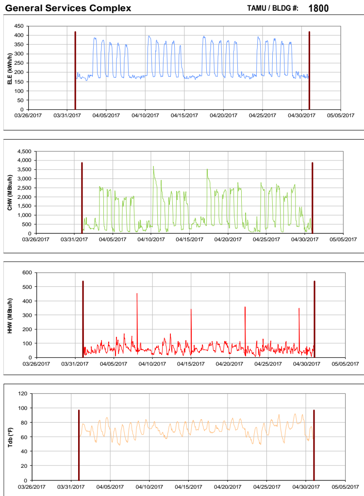
Figure III-189 Hourly Whole Building Electricity, Chilled Water, and Hot Water Consumption for General Services Complex during the Month of April 2017 and the Corresponding Hourly Outdoor Dry Bulb Temperature for College Station, TX
