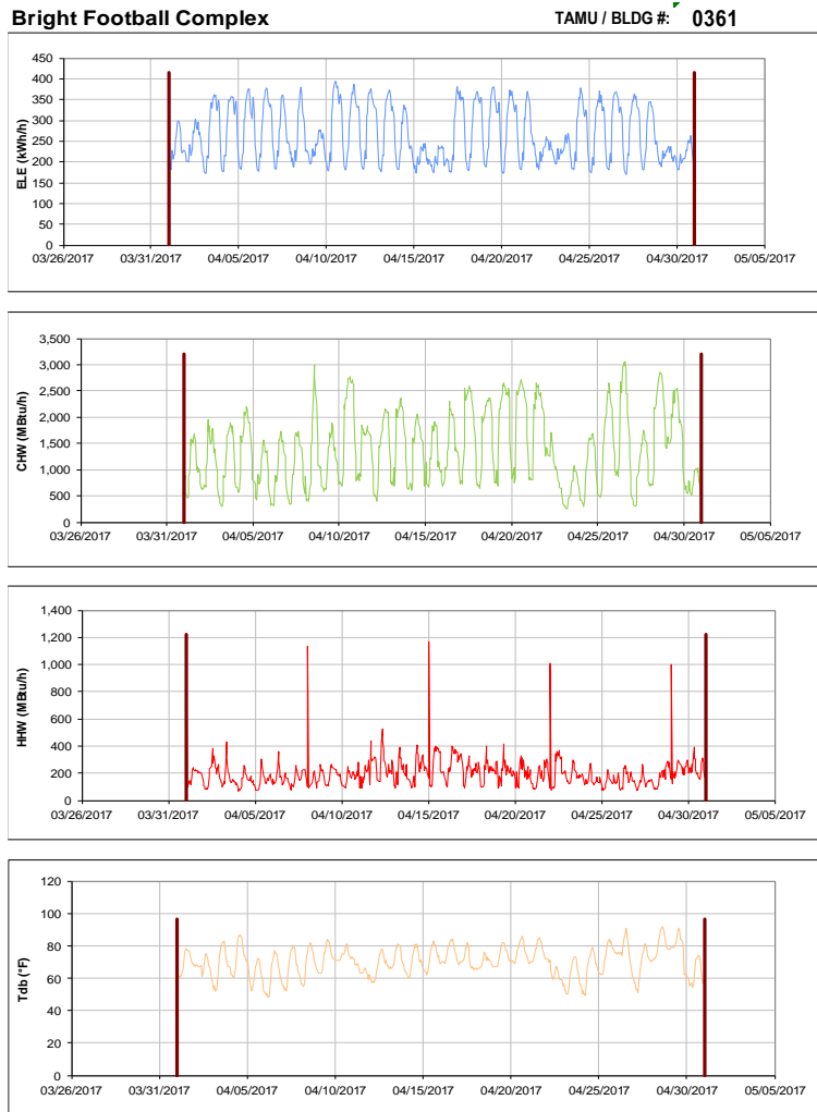
Figure III-15 Hourly Whole Building Electricity, Chilled Water, and Hot Water Consumption for Bright Football Complex during the Month of April 2017 and the Corresponding Hourly Outdoor Dry Bulb Temperature for College Station, TX
