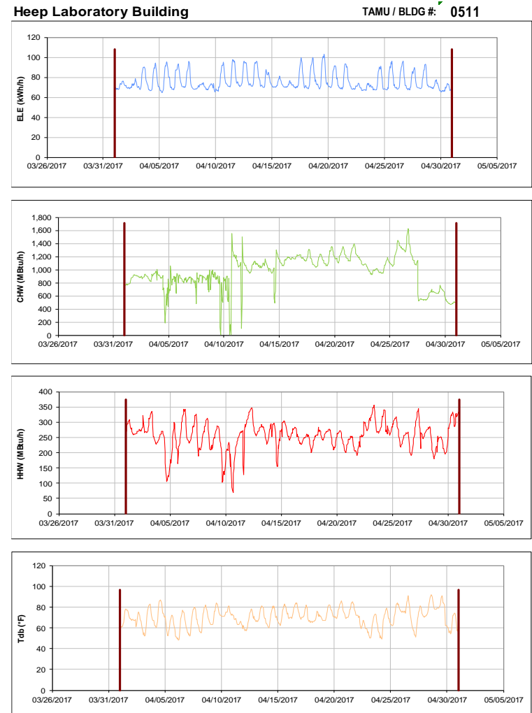
Figure III-108 Hourly Whole Building Electricity, Chilled Water, and Hot Water Consumption for Heep Laboratory Building during the Month of April 2017 and the Corresponding Hourly Outdoor Dry Bulb Temperature for College Station, TX
