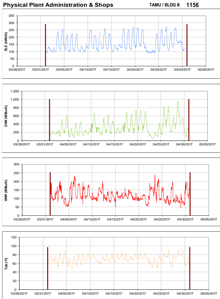
Figure III-133 Hourly Whole Building Electricity, Chilled Water, and Hot Water Consumption for Physical Plant Administration & Shops during the Month of April 2017 and the Corresponding Hourly Outdoor Dry Bulb Temperature for College Station, TX
