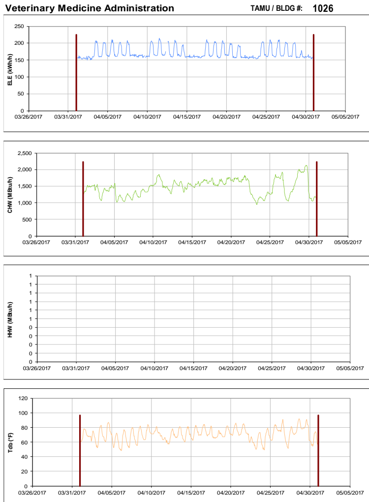
Figure III-107 Hourly Whole Building Electricity, Chilled Water, and Hot Water Consumption for Veterinary Medicine Administration during the Month of April 2017 and the Corresponding Hourly Outdoor Dry Bulb Temperature for College Station, TX
