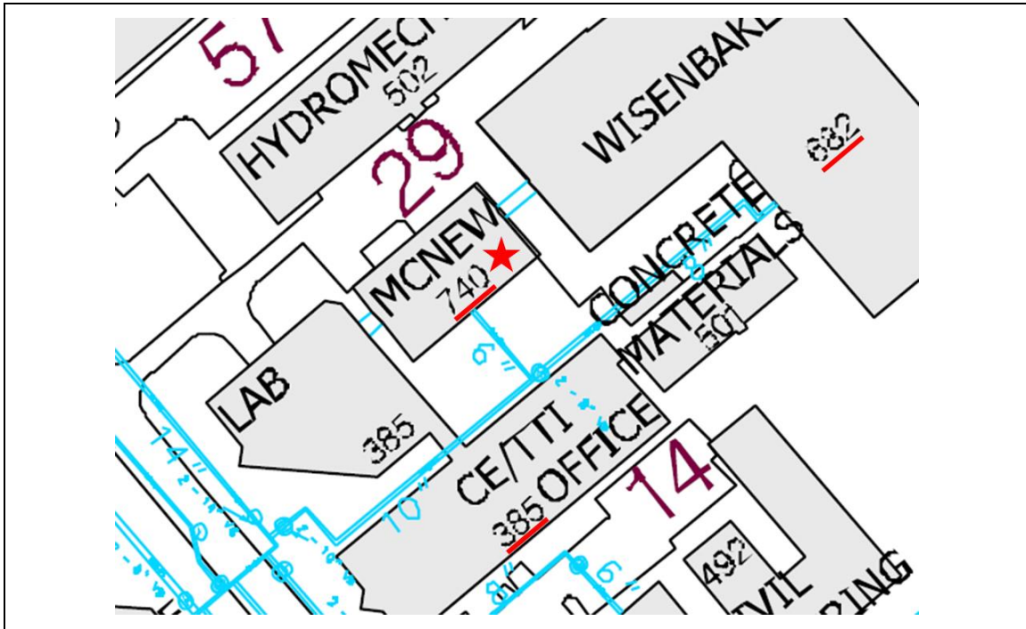
Explanatory Figure: CHW distribution with Bldgs. #740 McNew Laboratory, #682 Wisenbaker, and #385 CE/TTI Office during highlighted.
