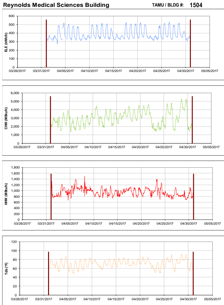
Figure III-153 Hourly Whole Building Electricity, Chilled Water, and Hot Water Consumption for Reynolds Medical Sciences Building during the Month of April 2017 and the Corresponding Hourly Outdoor Dry Bulb Temperature for College Station, TX
