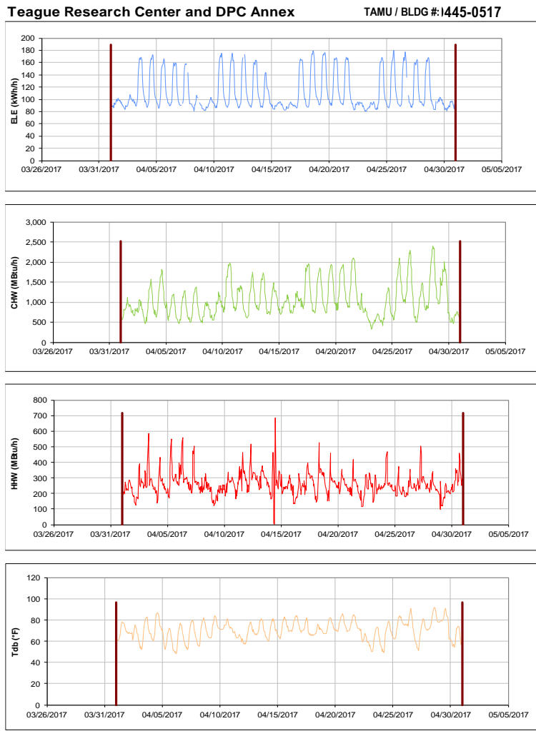
Figure III-65 Hourly Whole Building Electricity, Chilled Water, and Hot Water Consumption for Teague Research Center and DPC Annex during the Month of April 2017 and the Corresponding Hourly Outdoor Dry Bulb Temperature for College Station, TX
