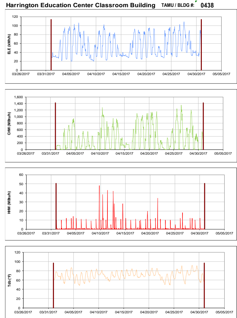
Figure III-62 Hourly Whole Building Electricity, Chilled Water, and Hot Water Consumption for Harrington Education Center Classroom Building during the Month of April 2017 and the Corresponding Hourly Outdoor Dry Bulb Temperature for College Station, TX
