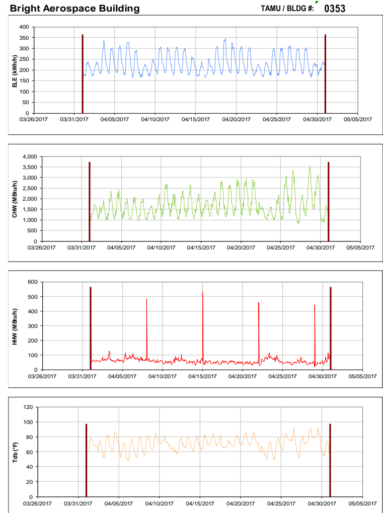
Figure III-10 Hourly Whole Building Electricity, Chilled Water, and Hot Water Consumption for Bright Aerospace Building during the Month of April 2017 and the Corresponding Hourly Outdoor Dry Bulb Temperature for College Station, TX
