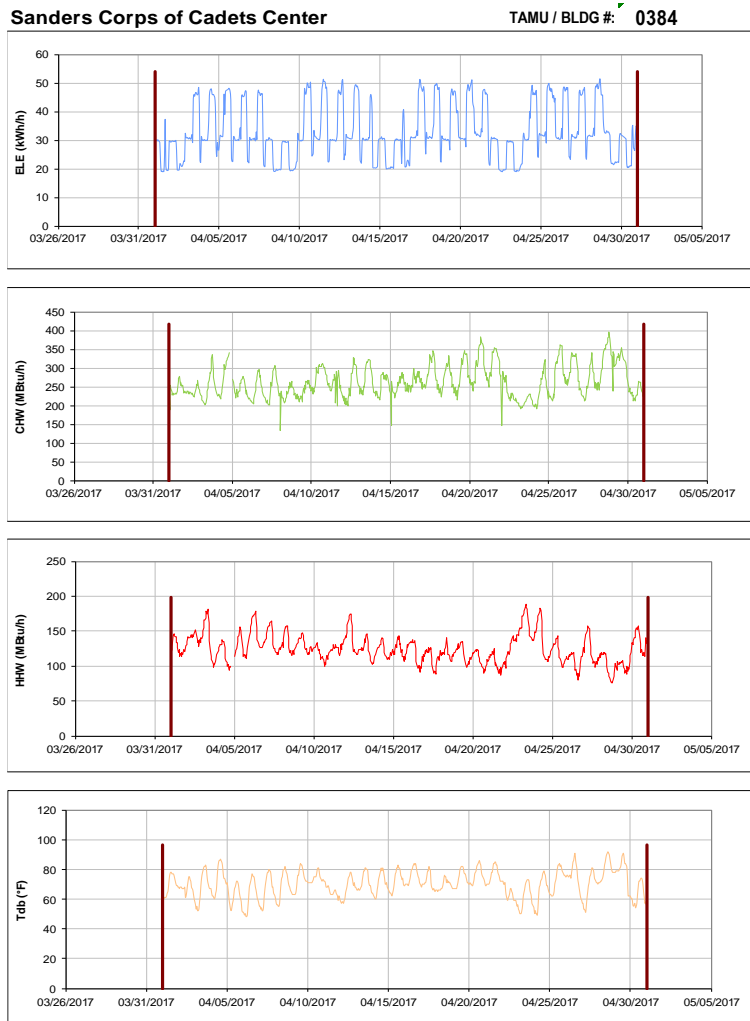
Figure III-19 Hourly Whole Building Electricity, Chilled Water, and Hot Water Consumption for Sanders Corps of Cadets Center during the Month of April 2017 and the Corresponding Hourly Outdoor Dry Bulb Temperature for College Station, TX
