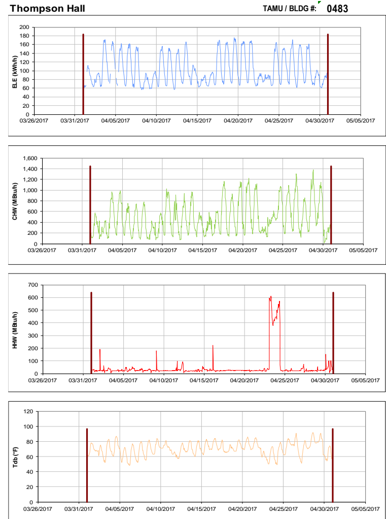
Figure III-96 Hourly Whole Building Electricity, Chilled Water, and Hot Water Consumption for Thompson Hall during the Month of April 2017 and the Corresponding Hourly Outdoor Dry Bulb Temperature for College Station, TX
