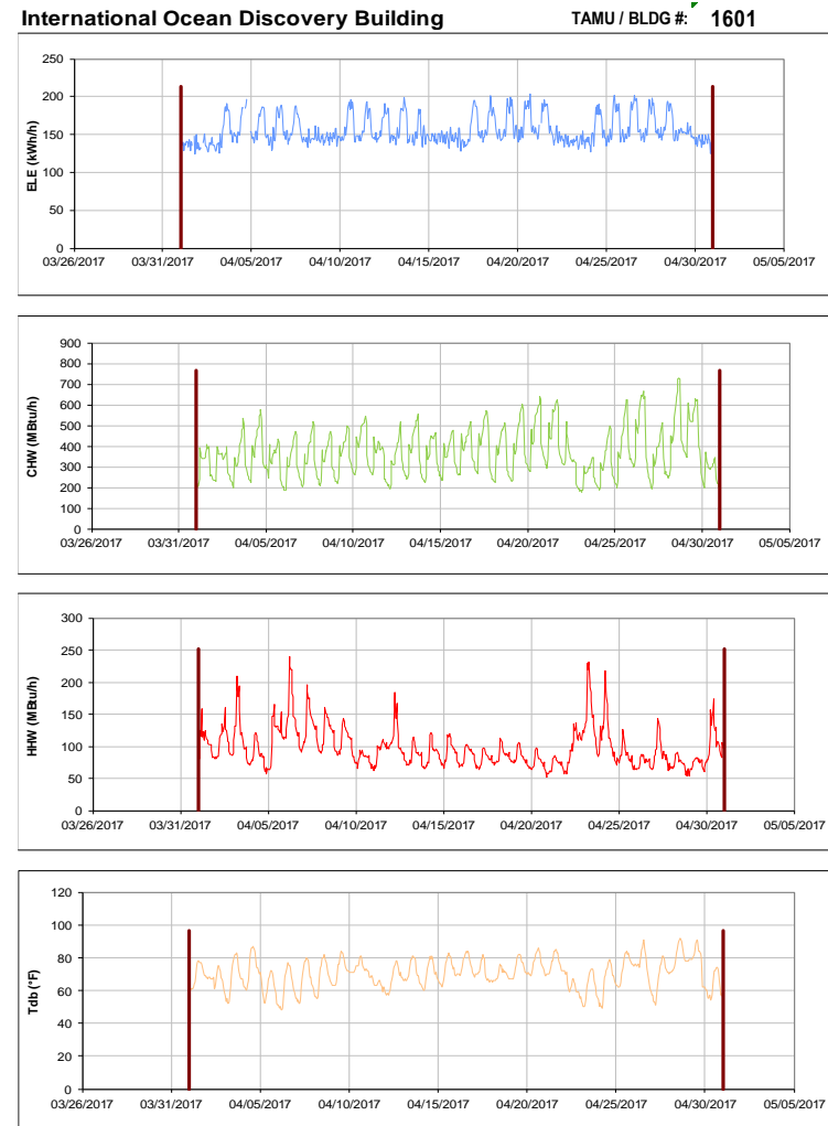
Figure III-182 Hourly Whole Building Electricity, Chilled Water, and Hot Water Consumption for International Ocean Discovery Building during the Month of April 2017 and the Corresponding Hourly Outdoor Dry Bulb Temperature for College Station, TX
