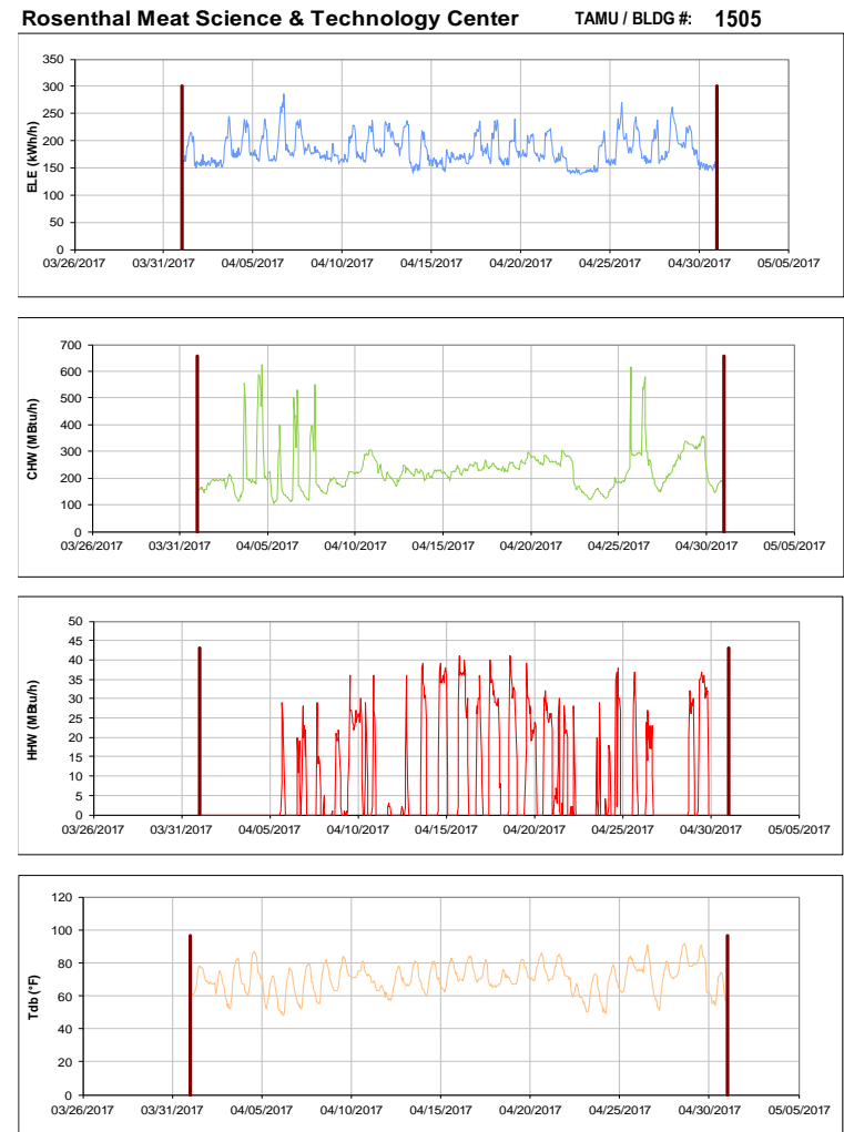
Figure III-154 Hourly Whole Building Electricity, Chilled Water, and Hot Water Consumption for Rosenthal Meat Science & Technology Center during the Month of April 2017 and the Corresponding Hourly Outdoor Dry Bulb Temperature for College Station, TX
