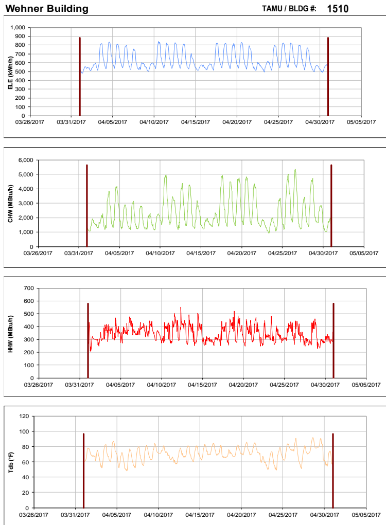
Figure III-159 Hourly Whole Building Electricity, Chilled Water, and Hot Water Consumption for Wehner Building during the Month of April 2017 and the Corresponding Hourly Outdoor Dry Bulb Temperature for College Station, TX
