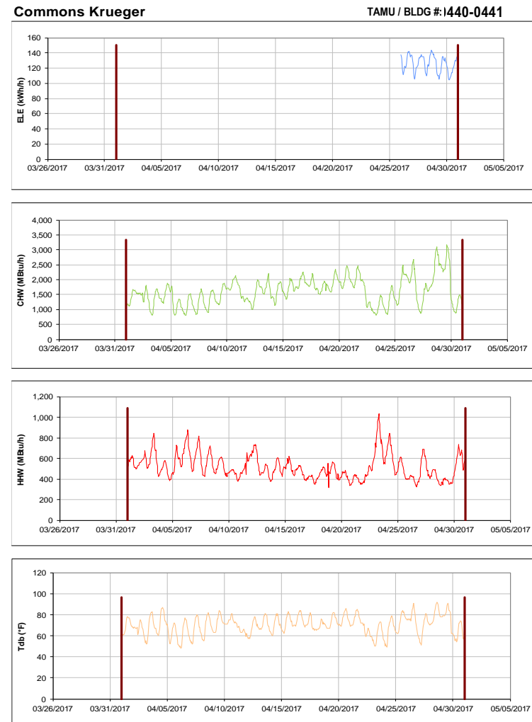
Figure III-52 Hourly Whole Building Electricity, Chilled Water, and Hot Water Consumption for Commons Krueger during the Month of April 2017 and the Corresponding Hourly Outdoor Dry Bulb Temperature for College Station, TX
