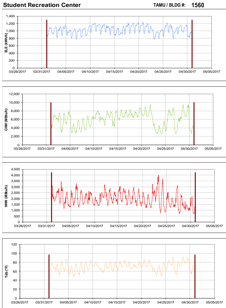
Figure III-177 Hourly Whole Building Electricity, Chilled Water, and Hot Water Consumption for Student Recreation Center during the Month of April 2017 and the Corresponding Hourly Outdoor Dry Bulb Temperature for College Station, TX
