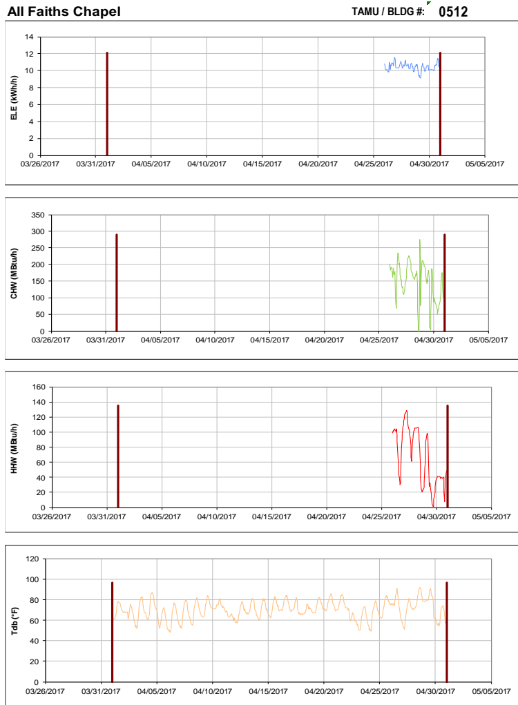
Figure III-109 Hourly Whole Building Electricity, Chilled Water, and Hot Water Consumption for All Faiths Chapel during the Month of April 2017 and the Corresponding Hourly Outdoor Dry Bulb Temperature for College Station, TX
