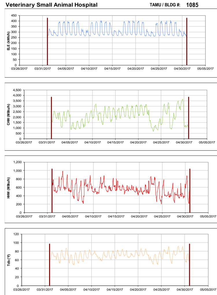
Figure III-130 Hourly Whole Building Electricity, Chilled Water, and Hot Water Consumption for Veterinary Small Animal Hospital during the Month of April 2017 and the Corresponding Hourly Outdoor Dry Bulb Temperature for College Station, TX
