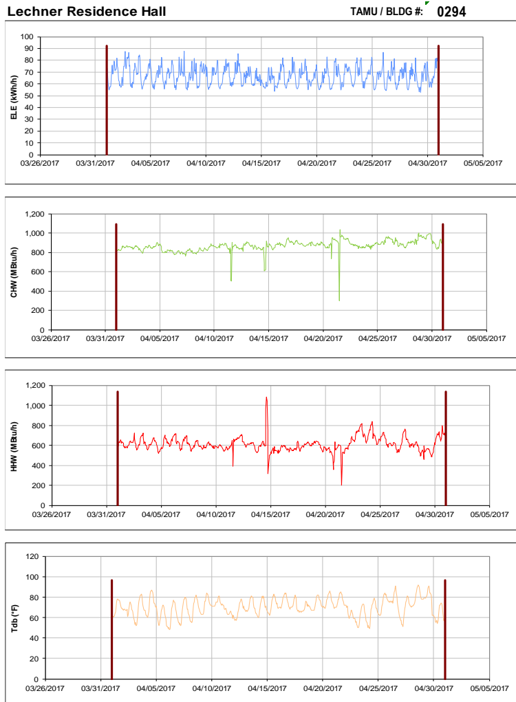
Figure III-7 Hourly Whole Building Electricity, Chilled Water, and Hot Water Consumption for Lechner Residence Hall during the Month of April 2017 and the Corresponding Hourly Outdoor Dry Bulb Temperature for College Station, TX
