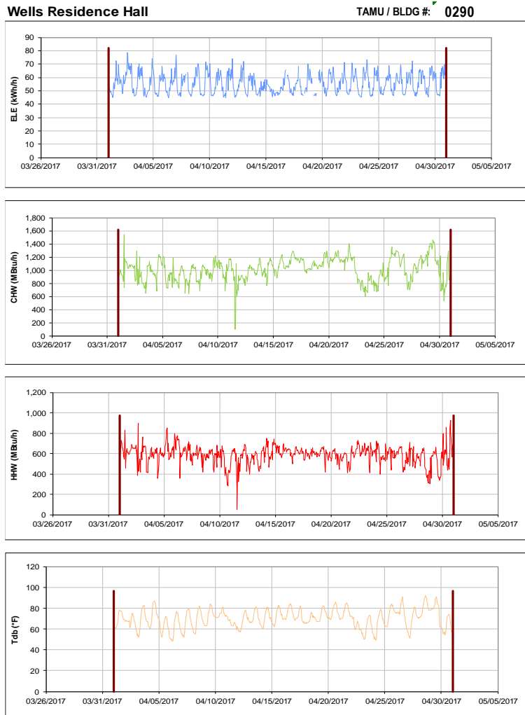
Figure III-3 Hourly Whole Building Electricity, Chilled Water, and Hot Water Consumption for Wells Residence Hall during the Month of April 2017 and the Corresponding Hourly Outdoor Dry Bulb Temperature for College Station, TX
