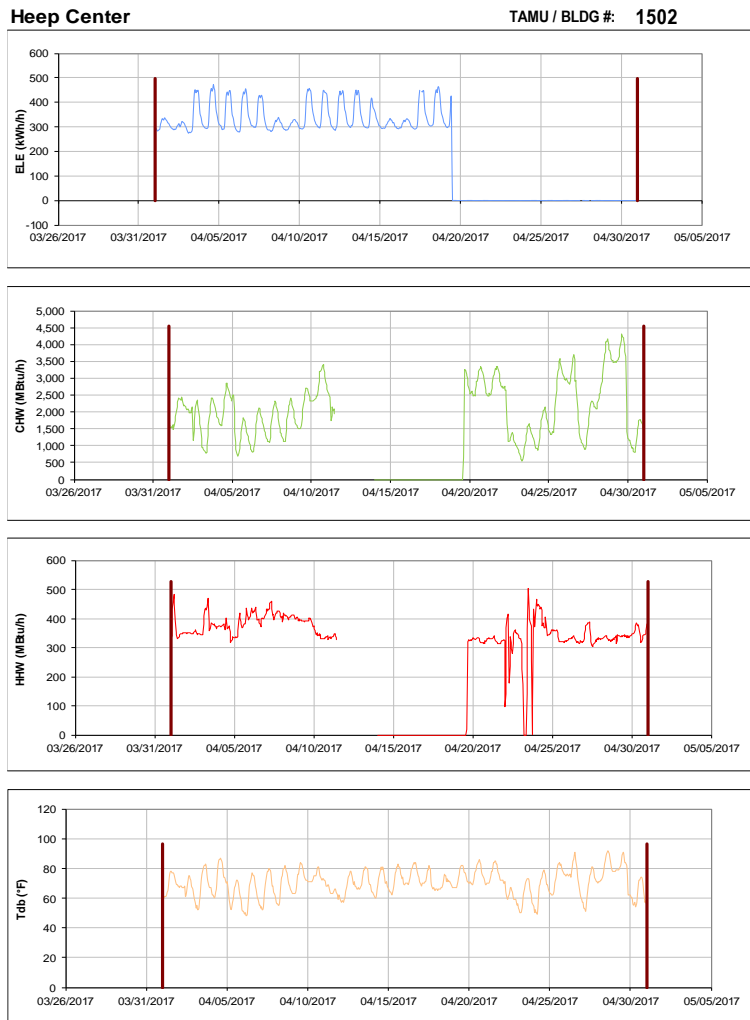
Figure III-151 Hourly Whole Building Electricity, Chilled Water, and Hot Water Consumption for Heep Center during the Month of April 2017 and the Corresponding Hourly Outdoor Dry Bulb Temperature for College Station, TX
