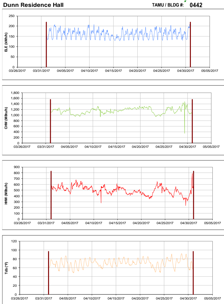
Figure III-55 Hourly Whole Building Electricity, Chilled Water, and Hot Water Consumption for Dunn Residence Hall during the Month of April 2017 and the Corresponding Hourly Outdoor Dry Bulb Temperature for College Station, TX
