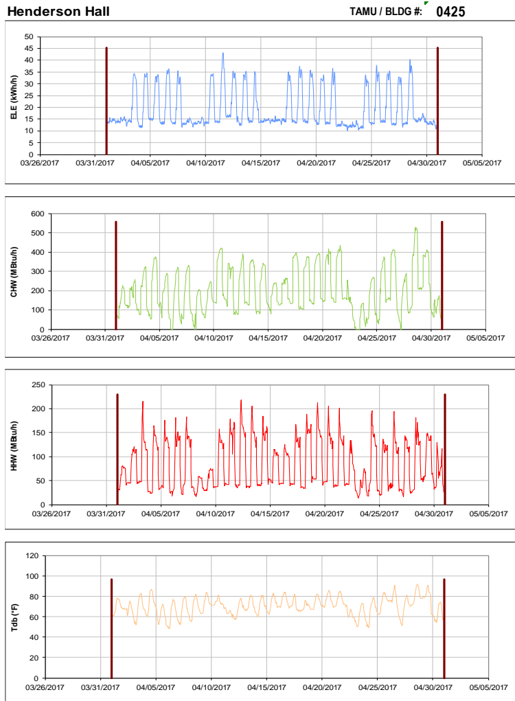
Figure III-47 Hourly Whole Building Electricity, Chilled Water, and Hot Water Consumption for Henderson Hall during the Month of April 2017 and the Corresponding Hourly Outdoor Dry Bulb Temperature for College Station, TX
