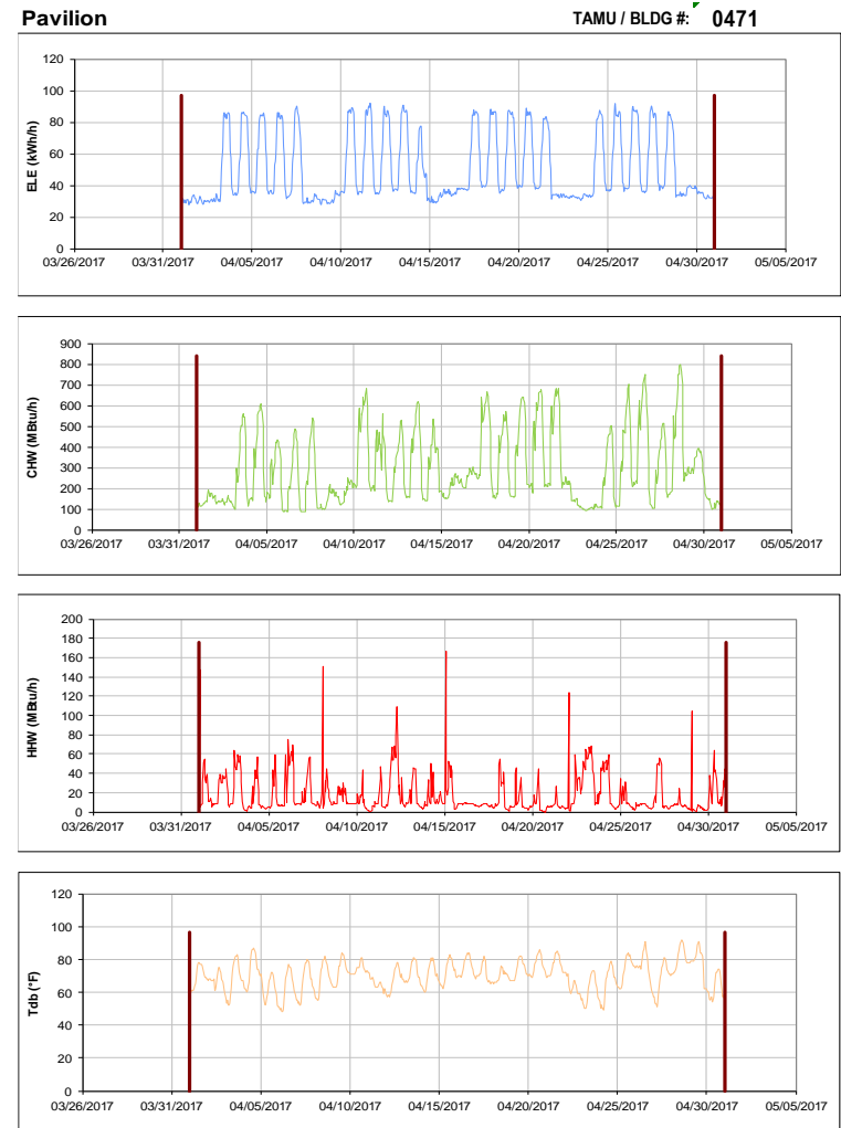
Figure III-86 Hourly Whole Building Electricity, Chilled Water, and Hot Water Consumption for Pavilion during the Month of April 2017 and the Corresponding Hourly Outdoor Dry Bulb Temperature for College Station, TX
