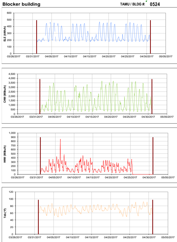
Figure III-115 Hourly Whole Building Electricity, Chilled Water, and Hot Water Consumption for Blocker building during the Month of April 2017 and the Corresponding Hourly Outdoor Dry Bulb Temperature for College Station, TX
