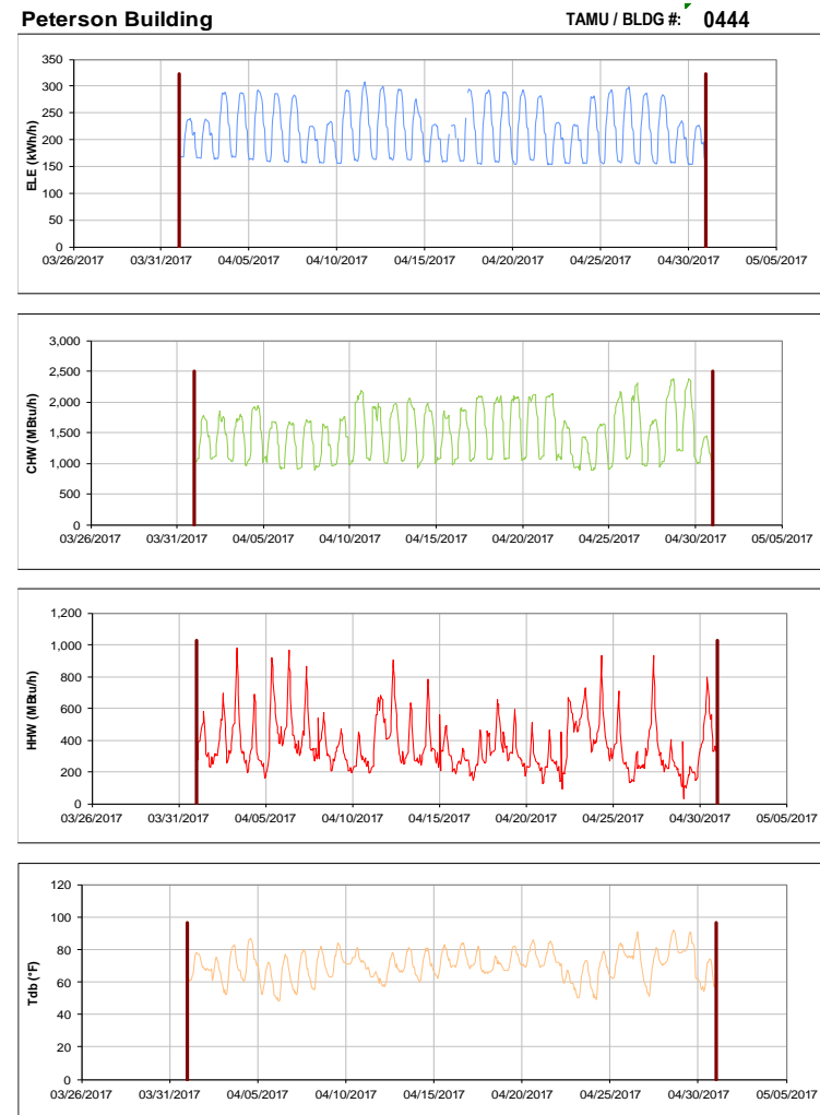
Figure III-64 Hourly Whole Building Electricity, Chilled Water, and Hot Water Consumption for Peterson Building during the Month of April 2017 and the Corresponding Hourly Outdoor Dry Bulb Temperature for College Station, TX
