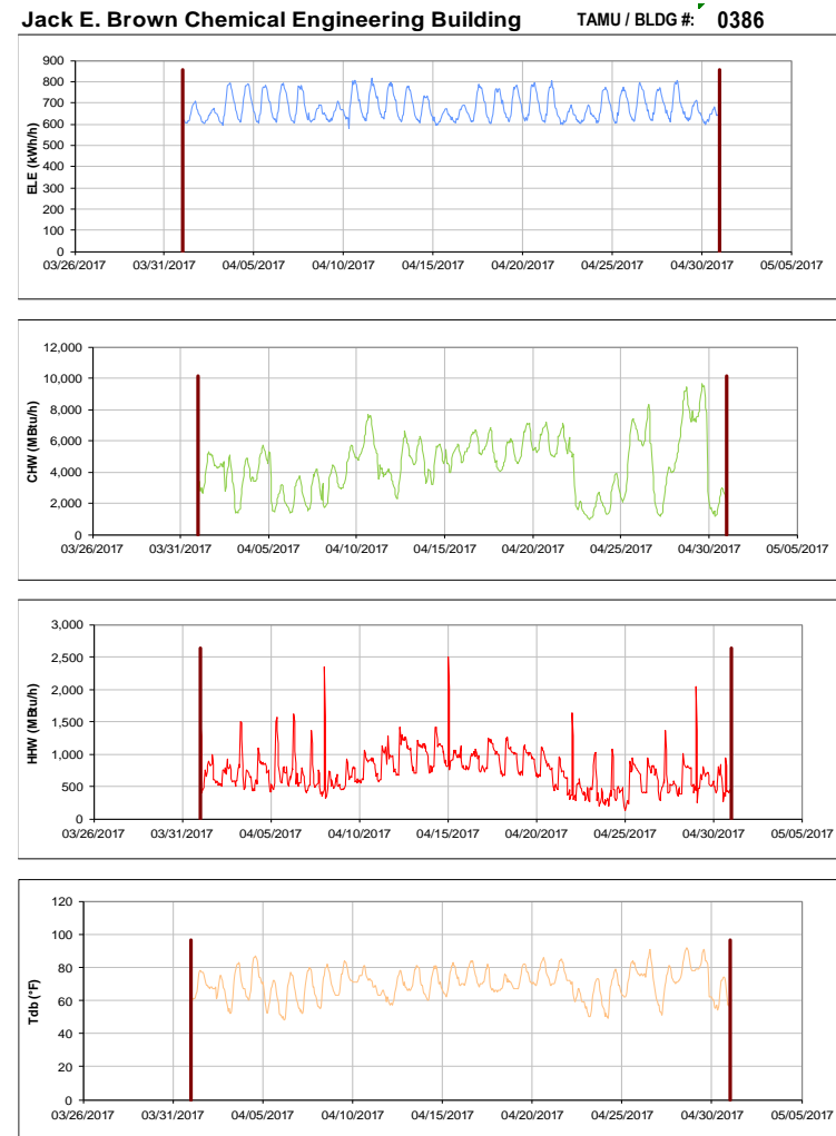
Figure III-20 Hourly Whole Building Electricity, Chilled Water, and Hot Water Consumption for Jack E. Brown Chemical Engineering Building during the Month of April 2017 and the Corresponding Hourly Outdoor Dry Bulb Temperature for College Station, TX
