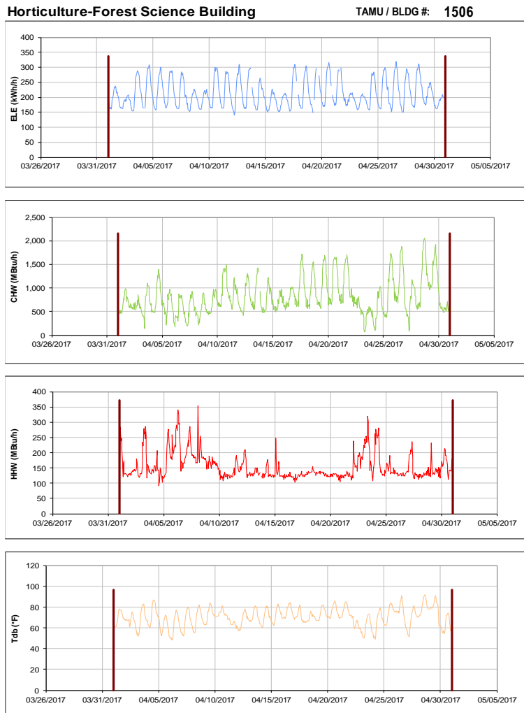
Figure III-155 Hourly Whole Building Electricity, Chilled Water, and Hot Water Consumption for Horticulture-Forest Science Building during the Month of April 2017 and the Corresponding Hourly Outdoor Dry Bulb Temperature for College Station, TX
