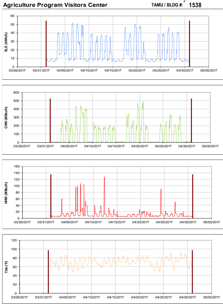
Figure III-169 Hourly Whole Building Electricity, Chilled Water, and Hot Water Consumption for Agriculture Program Visitors Center during the Month of April 2017 and the Corresponding Hourly Outdoor Dry Bulb Temperature for College Station, TX
