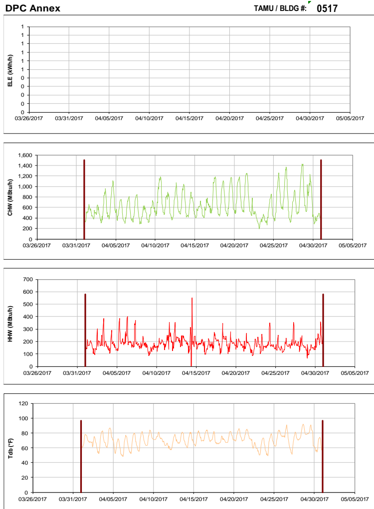
Figure III-67 Hourly Whole Building Electricity, Chilled Water, and Hot Water Consumption for DPC Annex during the Month of April 2017 and the Corresponding Hourly Outdoor Dry Bulb Temperature for College Station, TX
