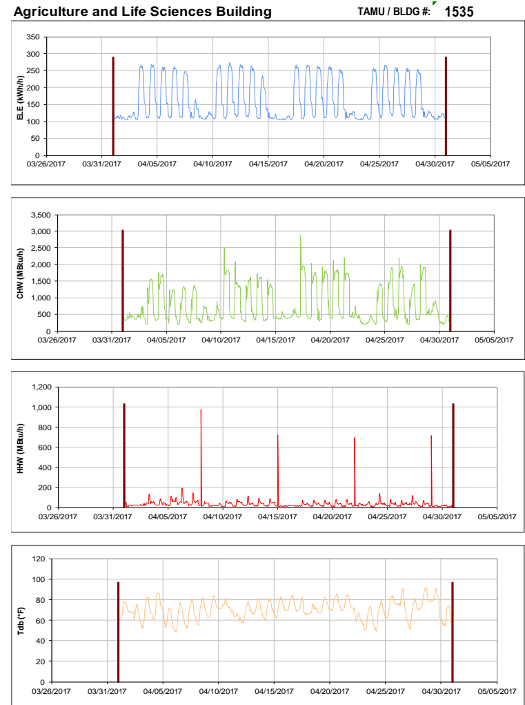
Figure III-166 Hourly Whole Building Electricity, Chilled Water, and Hot Water Consumption for Agriculture and Life Sciences Building during the Month of April 2017 and the Corresponding Hourly Outdoor Dry Bulb Temperature for College Station, TX
