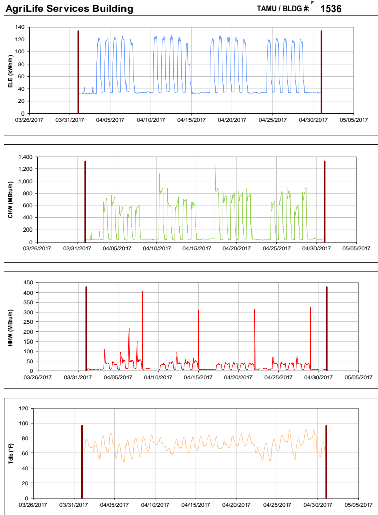
Figure III-167 Hourly Whole Building Electricity, Chilled Water, and Hot Water Consumption for AgriLife Services Building during the Month of April 2017 and the Corresponding Hourly Outdoor Dry Bulb Temperature for College Station, TX
