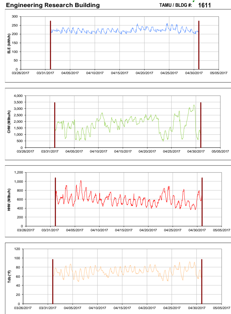
Figure III-188 Hourly Whole Building Electricity, Chilled Water, and Hot Water Consumption for Engineering Research Building during the Month of April 2017 and the Corresponding Hourly Outdoor Dry Bulb Temperature for College Station, TX
