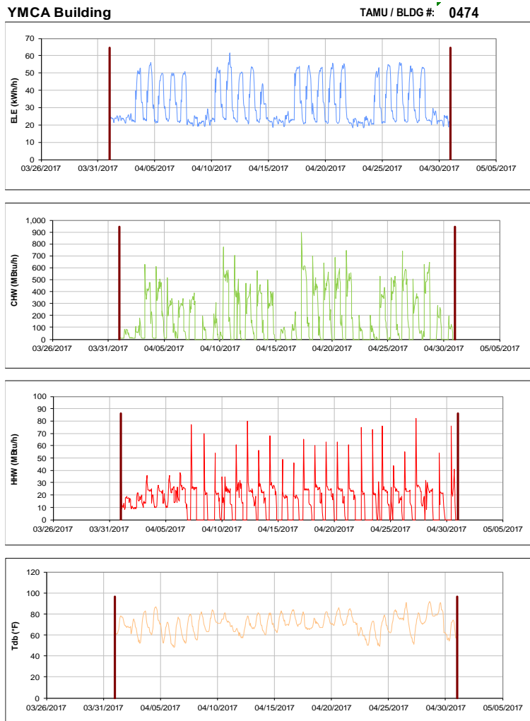
Figure III-89 Hourly Whole Building Electricity, Chilled Water, and Hot Water Consumption for YMCA Building during the Month of April 2017 and the Corresponding Hourly Outdoor Dry Bulb Temperature for College Station, TX
