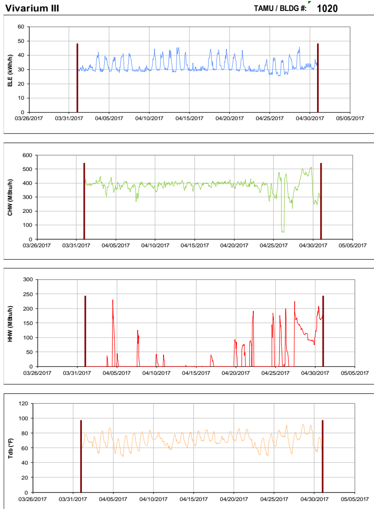
Figure III-127 Hourly Whole Building Electricity, Chilled Water, and Hot Water Consumption for Vivarium III during the Month of April 2017 and the Corresponding Hourly Outdoor Dry Bulb Temperature for College Station, TX
