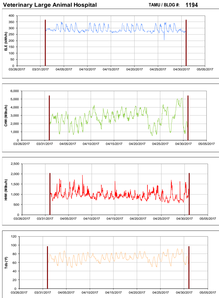
Figure III-135 Hourly Whole Building Electricity, Chilled Water, and Hot Water Consumption for Veterinary Large Animal Hospital during the Month of April 2017 and the Corresponding Hourly Outdoor Dry Bulb Temperature for College Station, TX
