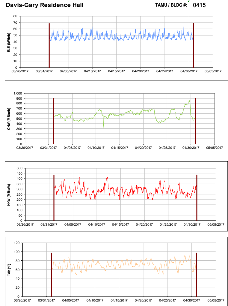
Figure III-42 Hourly Whole Building Electricity, Chilled Water, and Hot Water Consumption for Davis-Gary Residence Hall during the Month of April 2017 and the Corresponding Hourly Outdoor Dry Bulb Temperature for College Station, TX
