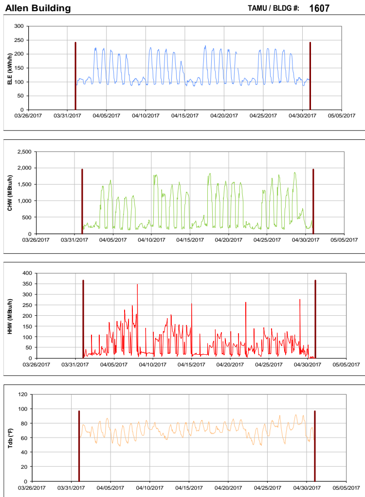
Figure III-185 Hourly Whole Building Electricity, Chilled Water, and Hot Water Consumption for Allen Building during the Month of April 2017 and the Corresponding Hourly Outdoor Dry Bulb Temperature for College Station, TX
