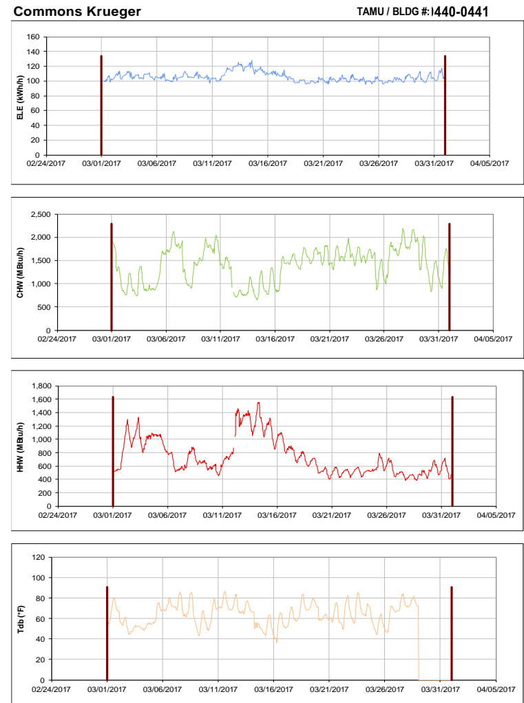
Figure III-52 Hourly Whole Building Electricity, Chilled Water, and Hot Water Consumption for Commons Krueger during the Month of March 2017 and the Corresponding Hourly Outdoor Dry Bulb Temperature for College Station, TX
