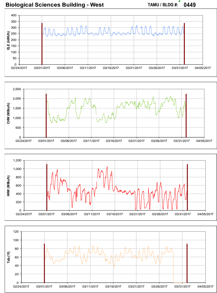
Figure III-72 Hourly Whole Building Electricity, Chilled Water, and Hot Water Consumption for Biological Sciences Building - West during the Month of March 2017 and the Corresponding Hourly Outdoor Dry Bulb Temperature for College Station, TX
