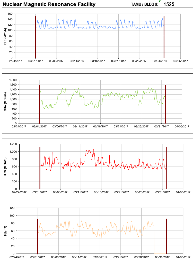
Figure III-163 Hourly Whole Building Electricity, Chilled Water, and Hot Water Consumption for Nuclear Magnetic Resonance Facility during the Month of March 2017 and the Corresponding Hourly Outdoor Dry Bulb Temperature for College Station, TX
