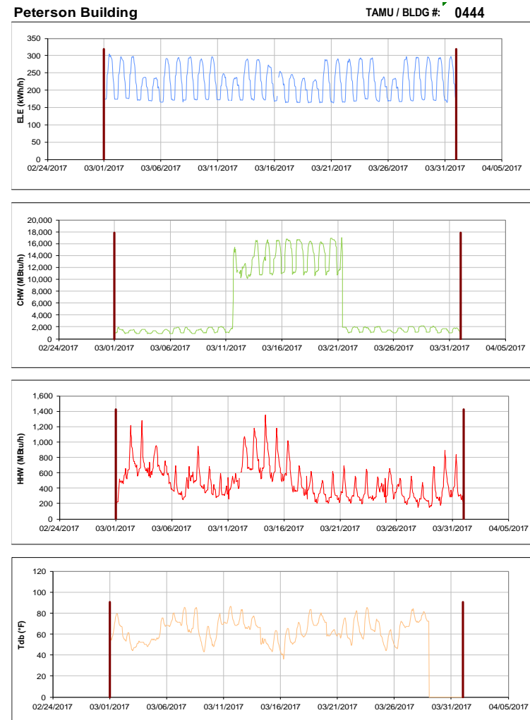
Figure III-64 Hourly Whole Building Electricity, Chilled Water, and Hot Water Consumption for Peterson Building during the Month of March 2017 and the Corresponding Hourly Outdoor Dry Bulb Temperature for College Station, TX
