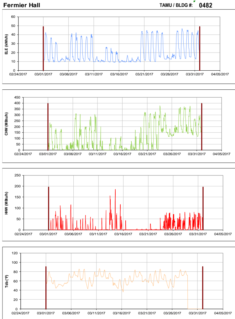
Figure III-95 Hourly Whole Building Electricity, Chilled Water, and Hot Water Consumption for Fermier Hall during the Month of March 2017 and the Corresponding Hourly Outdoor Dry Bulb Temperature for College Station, TX
