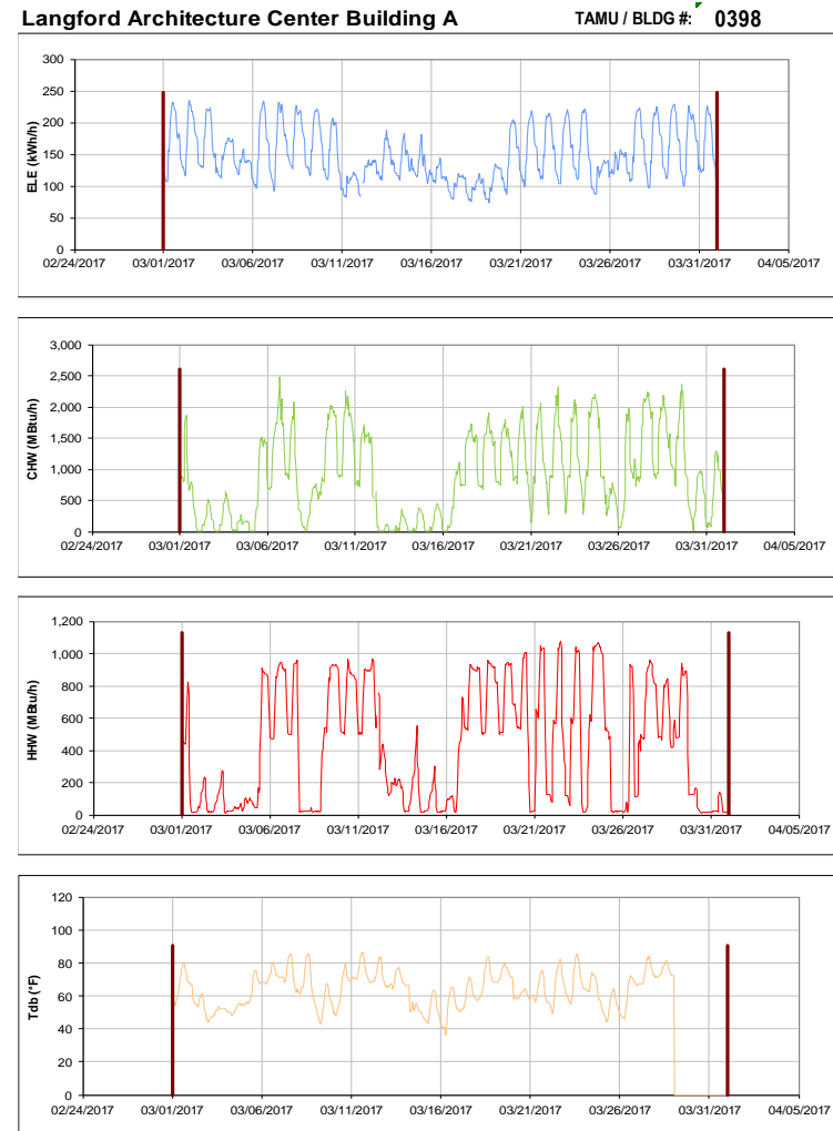
Figure III-24 Hourly Whole Building Electricity, Chilled Water, and Hot Water Consumption for Langford Architecture Center Building A during the Month of March 2017 and the Corresponding Hourly Outdoor Dry Bulb Temperature for College Station, TX
