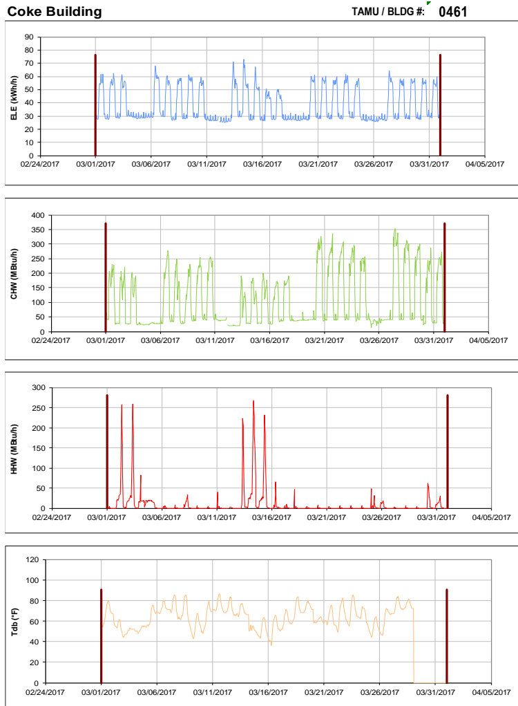
Figure III-77 Hourly Whole Building Electricity, Chilled Water, and Hot Water Consumption for Coke Building during the Month of March 2017 and the Corresponding Hourly Outdoor Dry Bulb Temperature for College Station, TX
