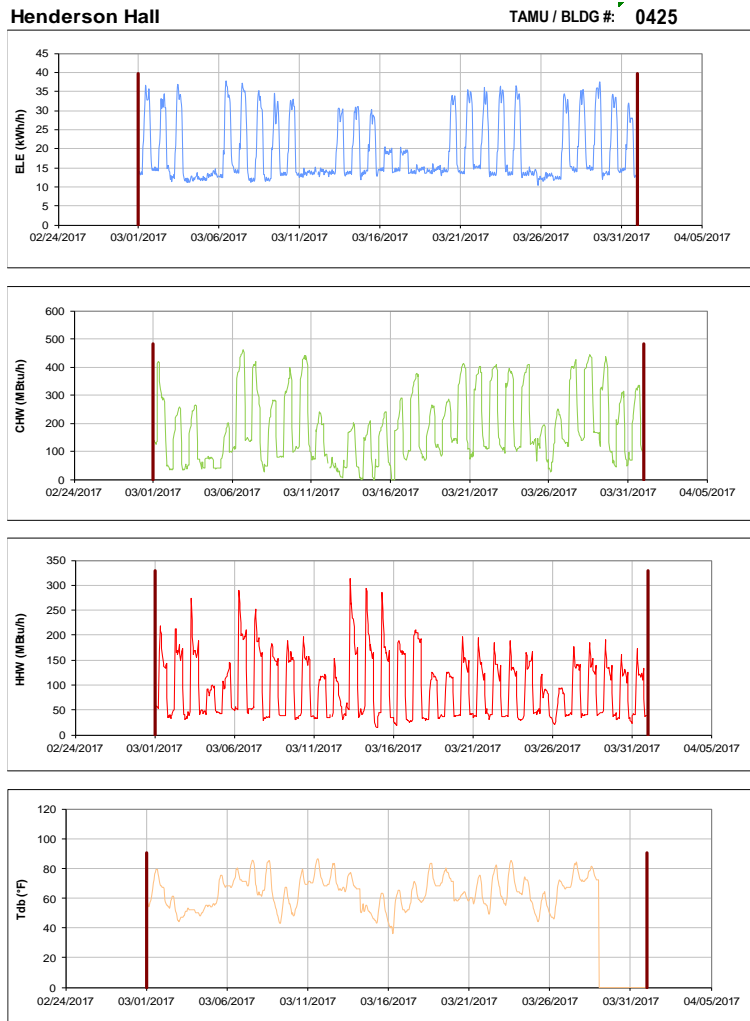
Figure III-47 Hourly Whole Building Electricity, Chilled Water, and Hot Water Consumption for Henderson Hall during the Month of March 2017 and the Corresponding Hourly Outdoor Dry Bulb Temperature for College Station, TX
