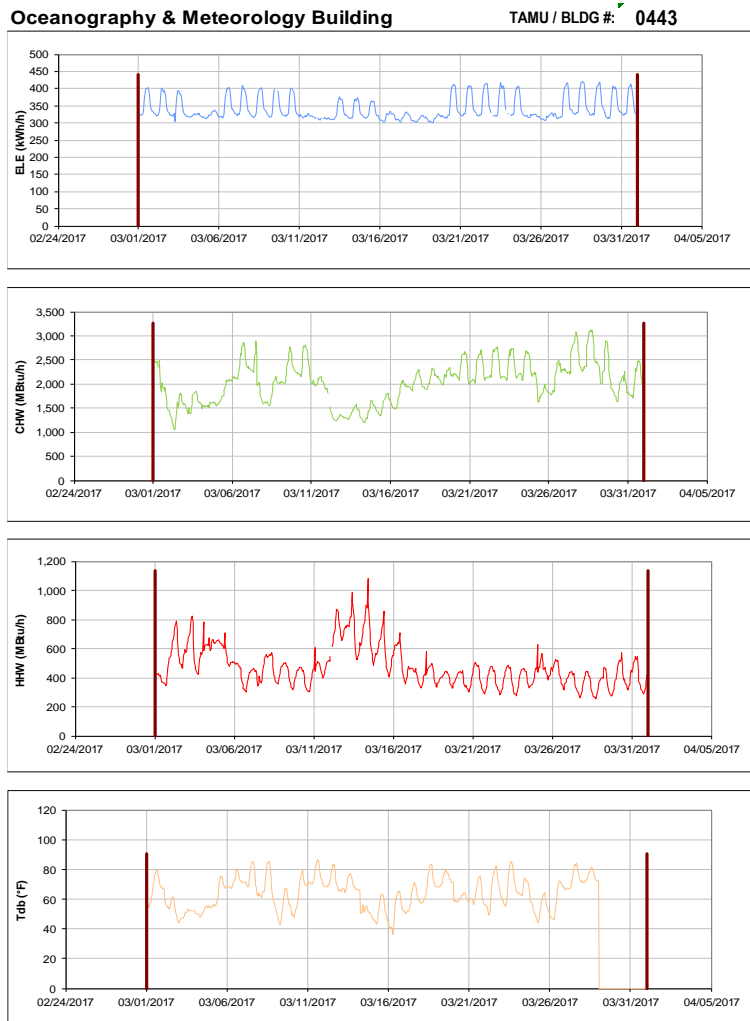
Figure III-63 Hourly Whole Building Electricity, Chilled Water, and Hot Water Consumption for Oceanography & Meteorology Building during the Month of March 2017 and the Corresponding Hourly Outdoor Dry Bulb Temperature for College Station, TX
