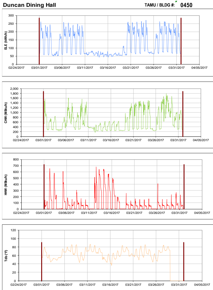
Figure III-73 Hourly Whole Building Electricity, Chilled Water, and Hot Water Consumption for Duncan Dining Hall during the Month of March 2017 and the Corresponding Hourly Outdoor Dry Bulb Temperature for College Station, TX
