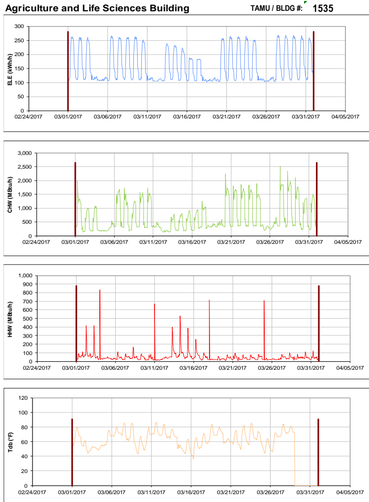
Figure III-165 Hourly Whole Building Electricity, Chilled Water, and Hot Water Consumption for Agriculture and Life Sciences Building during the Month of March 2017 and the Corresponding Hourly Outdoor Dry Bulb Temperature for College Station, TX
