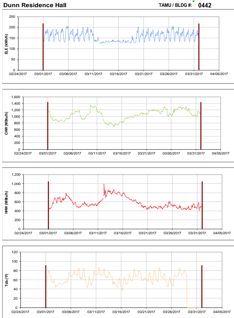
Figure III-55 Hourly Whole Building Electricity, Chilled Water, and Hot Water Consumption for Dunn Residence Hall during the Month of March 2017 and the Corresponding Hourly Outdoor Dry Bulb Temperature for College Station, TX
