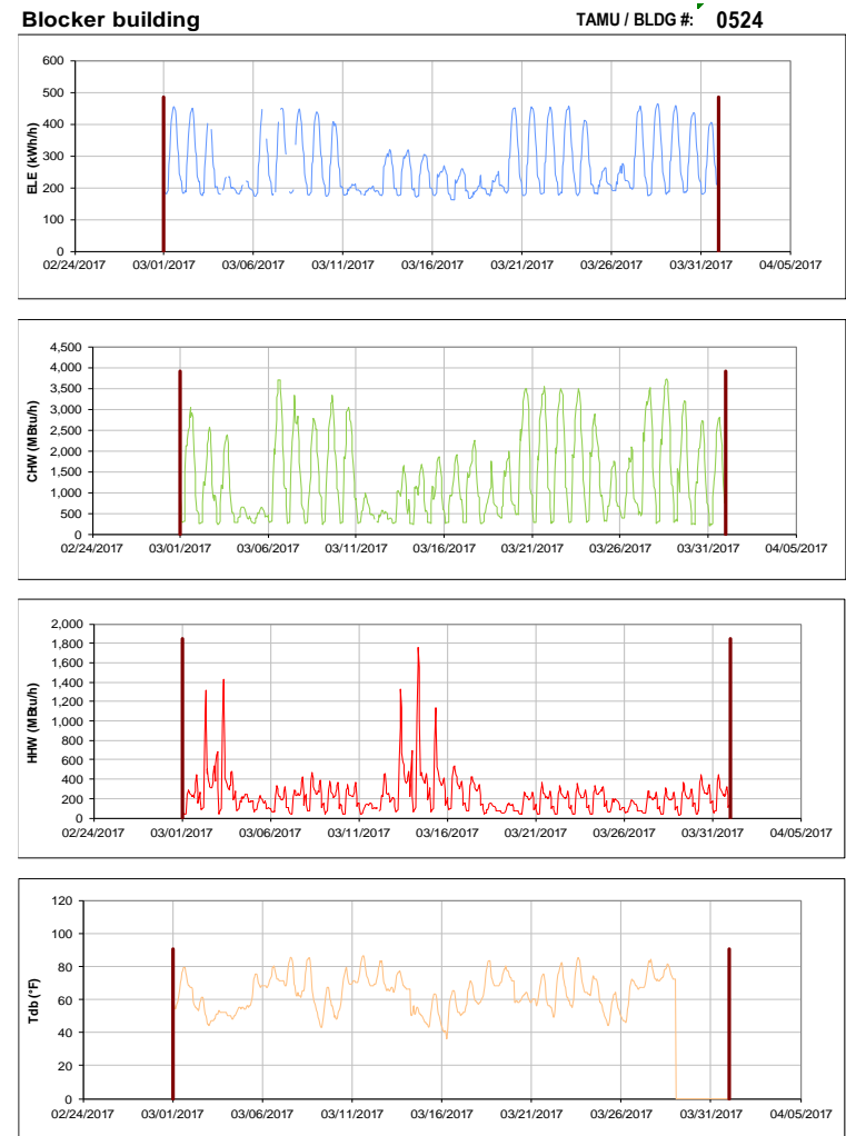
Figure III-114 Hourly Whole Building Electricity, Chilled Water, and Hot Water Consumption for Blocker building during the Month of March 2017 and the Corresponding Hourly Outdoor Dry Bulb Temperature for College Station, TX
