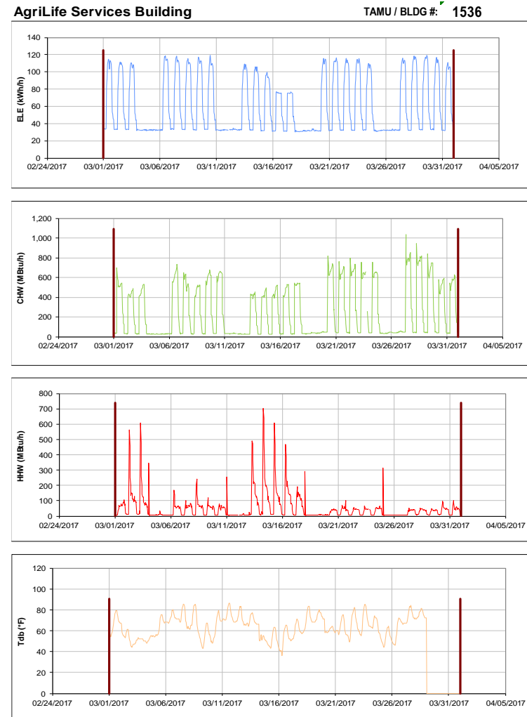
Figure III-166 Hourly Whole Building Electricity, Chilled Water, and Hot Water Consumption for AgriLife Services Building during the Month of March 2017 and the Corresponding Hourly Outdoor Dry Bulb Temperature for College Station, TX
