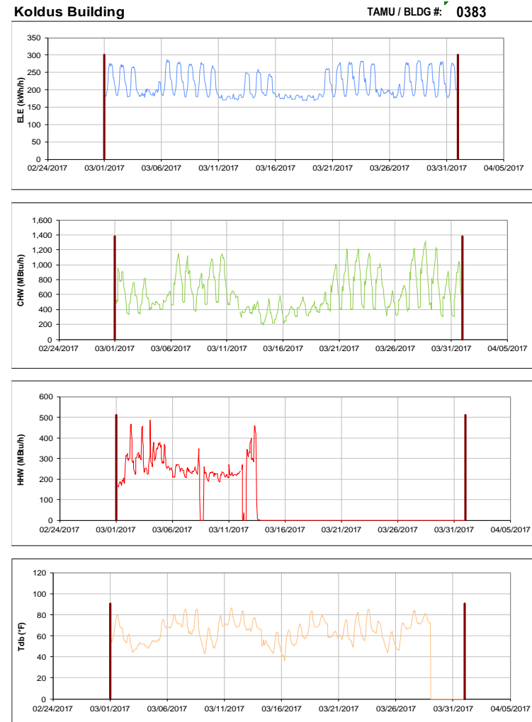
Figure III-18 Hourly Whole Building Electricity, Chilled Water, and Hot Water Consumption for Koldus Building during the Month of March 2017 and the Corresponding Hourly Outdoor Dry Bulb Temperature for College Station, TX
