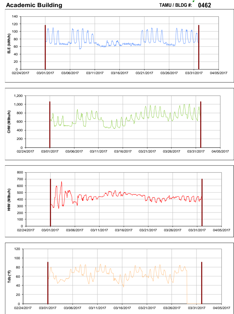
Figure III-78 Hourly Whole Building Electricity, Chilled Water, and Hot Water Consumption for Academic Building during the Month of March 2017 and the Corresponding Hourly Outdoor Dry Bulb Temperature for College Station, TX
