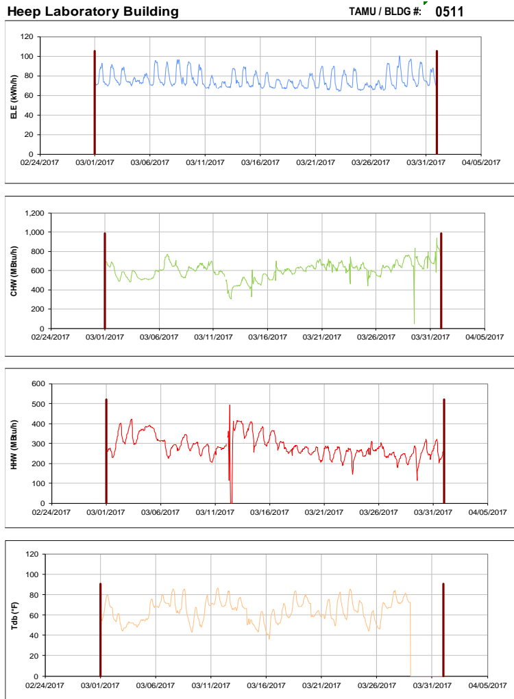
Figure III-107 Hourly Whole Building Electricity, Chilled Water, and Hot Water Consumption for Heep Laboratory Building during the Month of March 2017 and the Corresponding Hourly Outdoor Dry Bulb Temperature for College Station, TX
