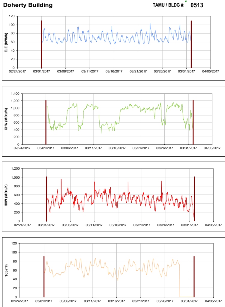
Figure III-109 Hourly Whole Building Electricity, Chilled Water, and Hot Water Consumption for Doherty Building during the Month of March 2017 and the Corresponding Hourly Outdoor Dry Bulb Temperature for College Station, TX
