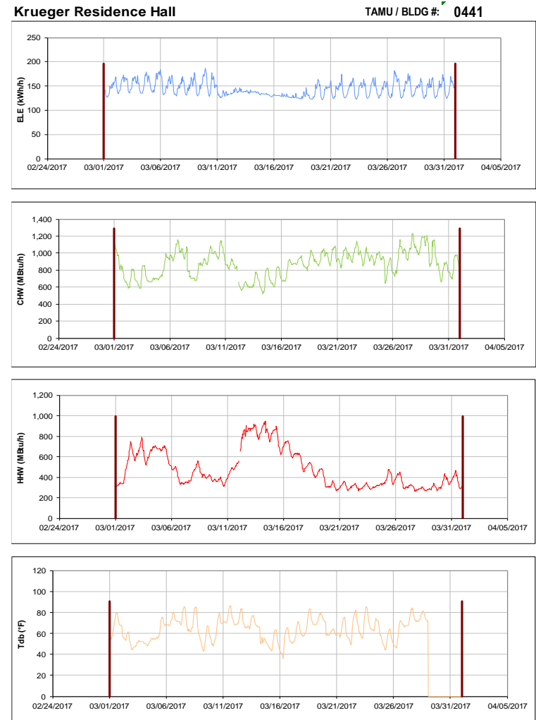
Figure III-54 Hourly Whole Building Electricity, Chilled Water, and Hot Water Consumption for Krueger Residence Hall during the Month of March 2017 and the Corresponding Hourly Outdoor Dry Bulb Temperature for College Station, TX
