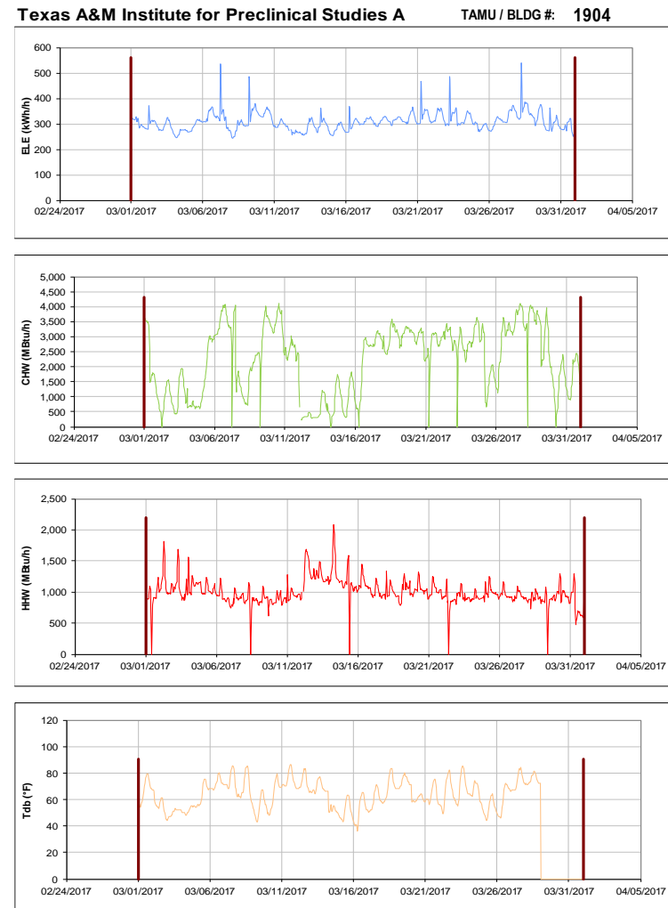
Figure III-194 Hourly Whole Building Electricity, Chilled Water, and Hot Water Consumption for Texas A&M Institute for Preclinical Studies A during the Month of March 2017 and the Corresponding Hourly Outdoor Dry Bulb Temperature for College Station, TX
