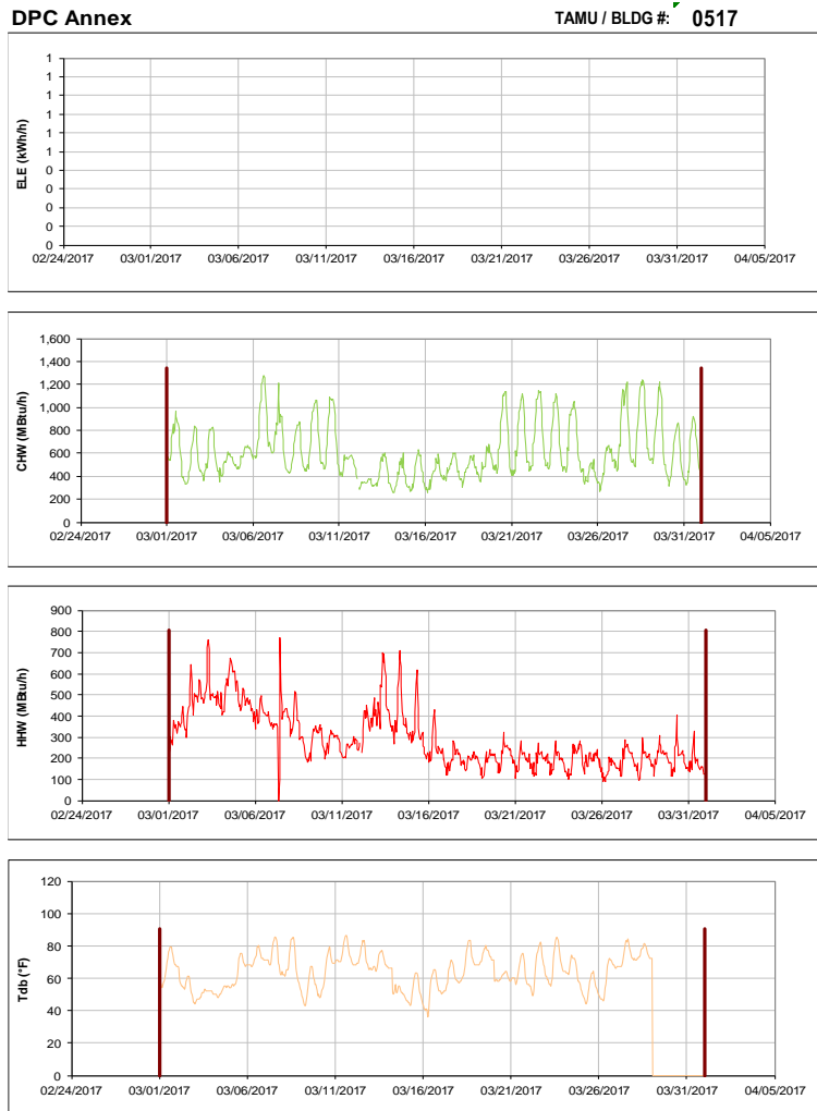
Figure III-67 Hourly Whole Building Electricity, Chilled Water, and Hot Water Consumption for DPC Annex during the Month of March 2017 and the Corresponding Hourly Outdoor Dry Bulb Temperature for College Station, TX
