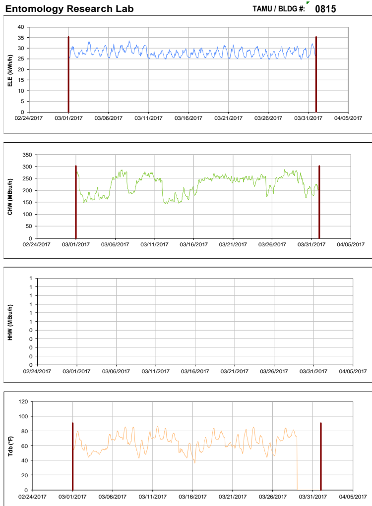
Figure III-123 Hourly Whole Building Electricity, Chilled Water, and Hot Water Consumption for Entomology Research Lab during the Month of March 2017 and the Corresponding Hourly Outdoor Dry Bulb Temperature for College Station, TX
