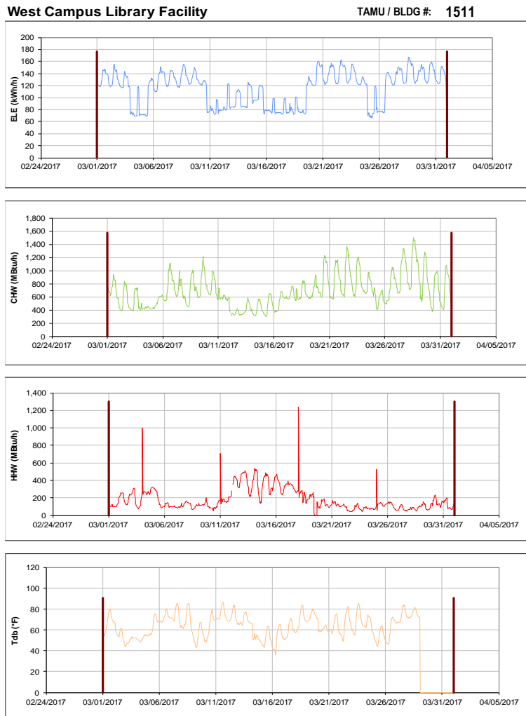
Figure III-159 Hourly Whole Building Electricity, Chilled Water, and Hot Water Consumption for West Campus Library Facility during the Month of March 2017 and the Corresponding Hourly Outdoor Dry Bulb Temperature for College Station, TX
