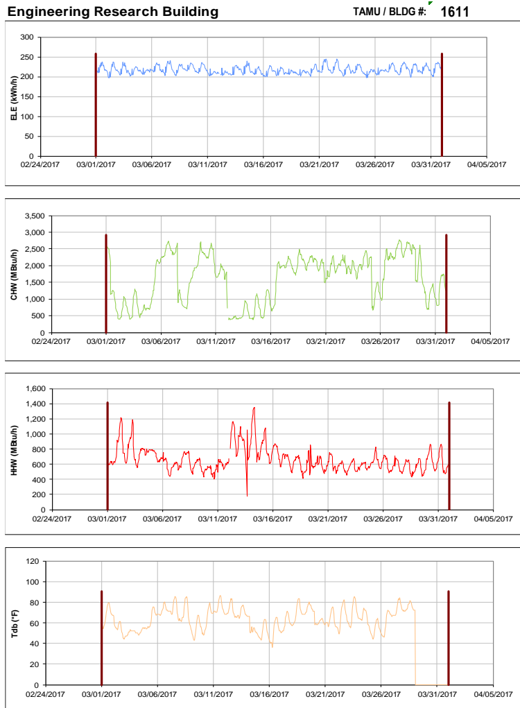
Figure III-187 Hourly Whole Building Electricity, Chilled Water, and Hot Water Consumption for Engineering Research Building during the Month of March 2017 and the Corresponding Hourly Outdoor Dry Bulb Temperature for College Station, TX
