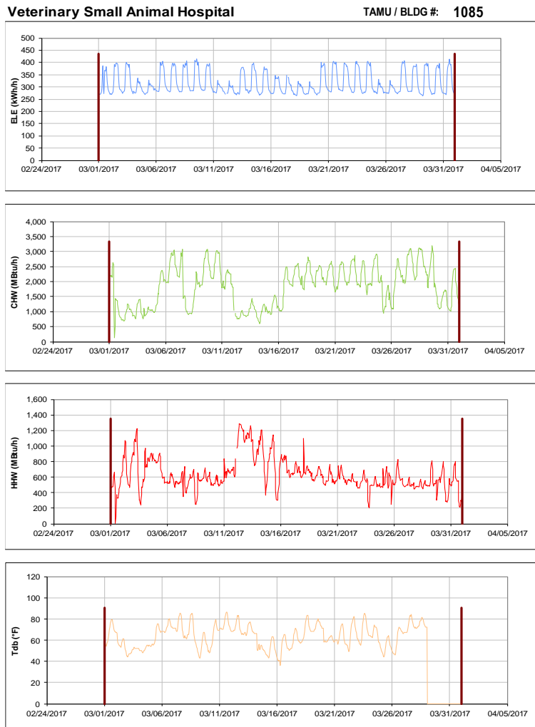
Figure III-129 Hourly Whole Building Electricity, Chilled Water, and Hot Water Consumption for Veterinary Small Animal Hospital during the Month of March 2017 and the Corresponding Hourly Outdoor Dry Bulb Temperature for College Station, TX
