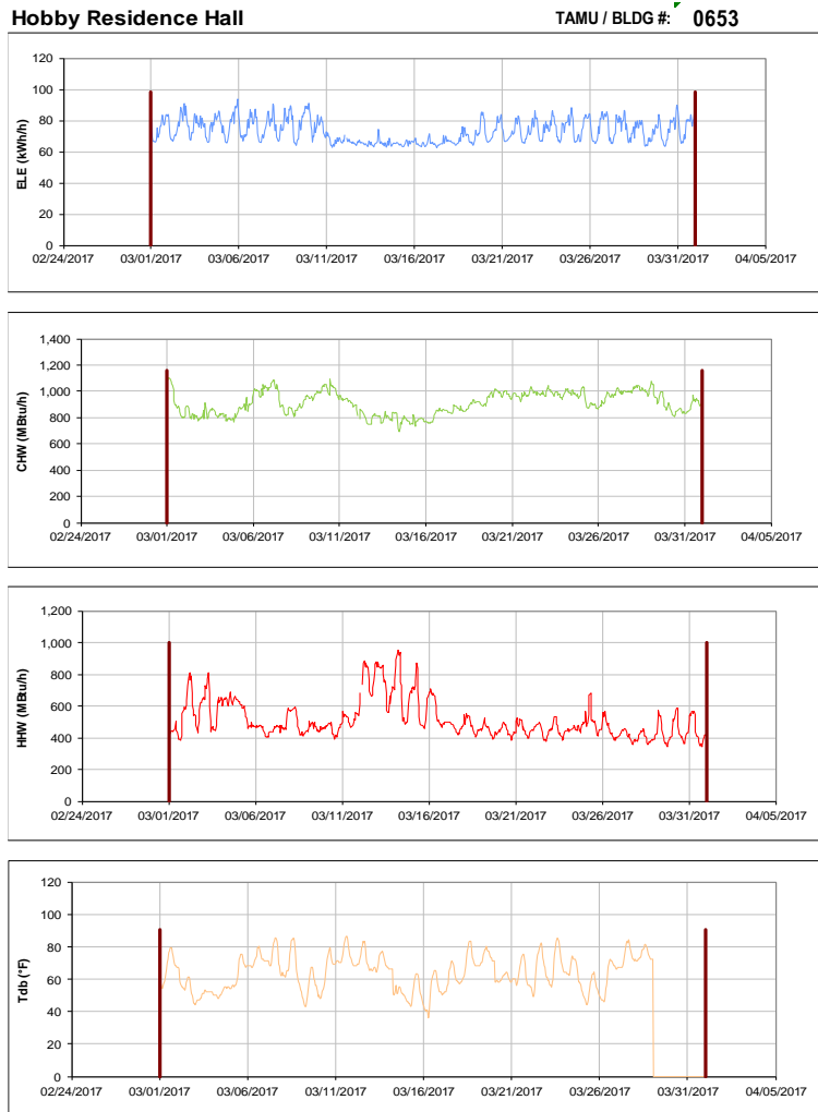
Figure III-119 Hourly Whole Building Electricity, Chilled Water, and Hot Water Consumption for Hobby Residence Hall during the Month of March 2017 and the Corresponding Hourly Outdoor Dry Bulb Temperature for College Station, TX
