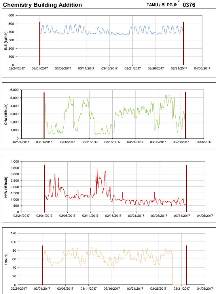
Figure III-17 Hourly Whole Building Electricity, Chilled Water, and Hot Water Consumption for Chemistry Building Addition during the Month of March 2017 and the Corresponding Hourly Outdoor Dry Bulb Temperature for College Station, TX
