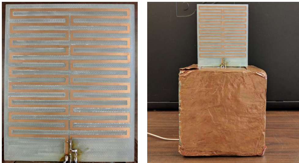
Figure 91. Fabricated loop antenna.
