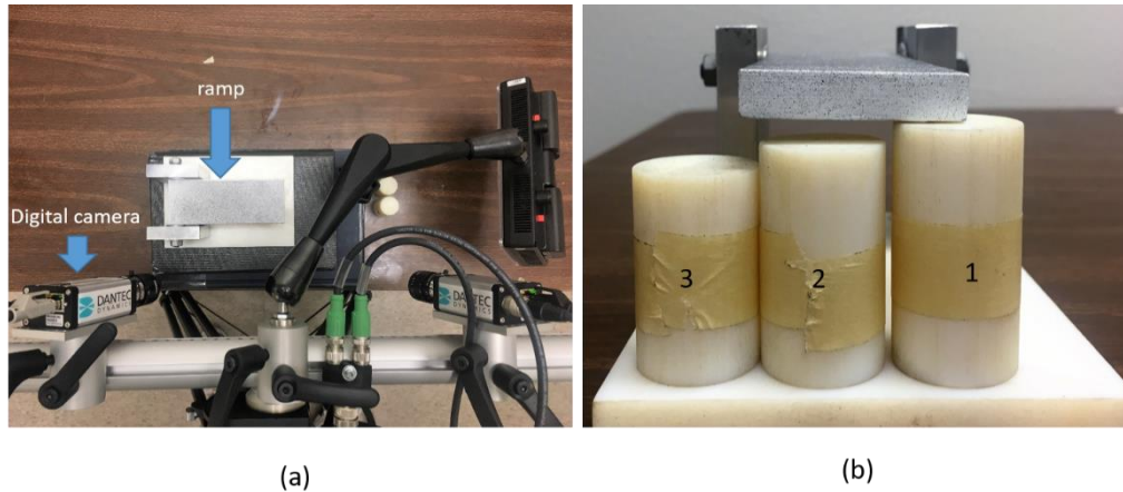
Figure 5-19: The experimental setup to perform noise analysis of the boundary displacement measurements utilizing a digital image correlation system. (a) top view of the experimental setup with digital cameras focusing on the ramp’s top face; (b) side view of the ramp with three columns having different height.
