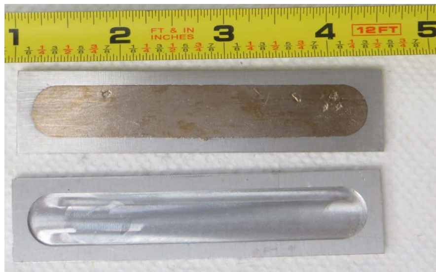
Figure 10. The basic target backing is shown, bare, and filled with bismuth.
