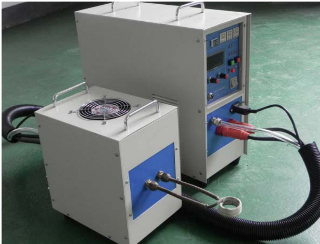
Figure 56. A commercially available miniature induction furnace. The coil is capable of inducing temperatures more than 1100 °C. The power supply and controller may be remotely mounted.
