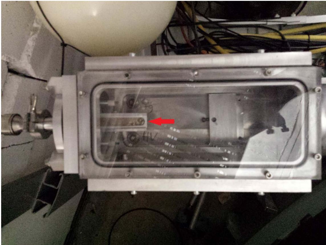
Figure 40. A view from the top of the vacuum enclosure, looking down on the target, located by the red arrow. The beam enters from the right.
