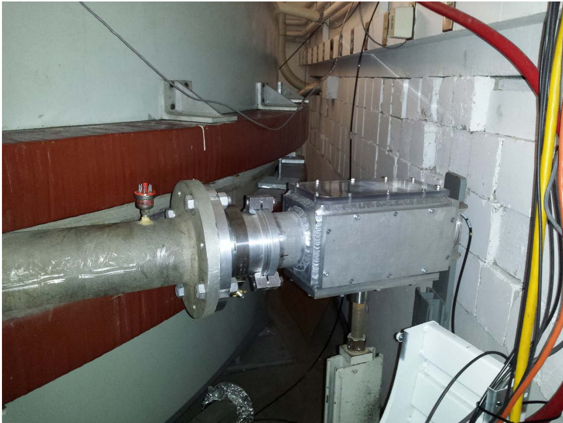
Figure 39. A view of the target vacuum enclosure. The beam line enters from the left. Note the shield wall to the right. The target is accessed by removing the screws and side plate facing the camera.
