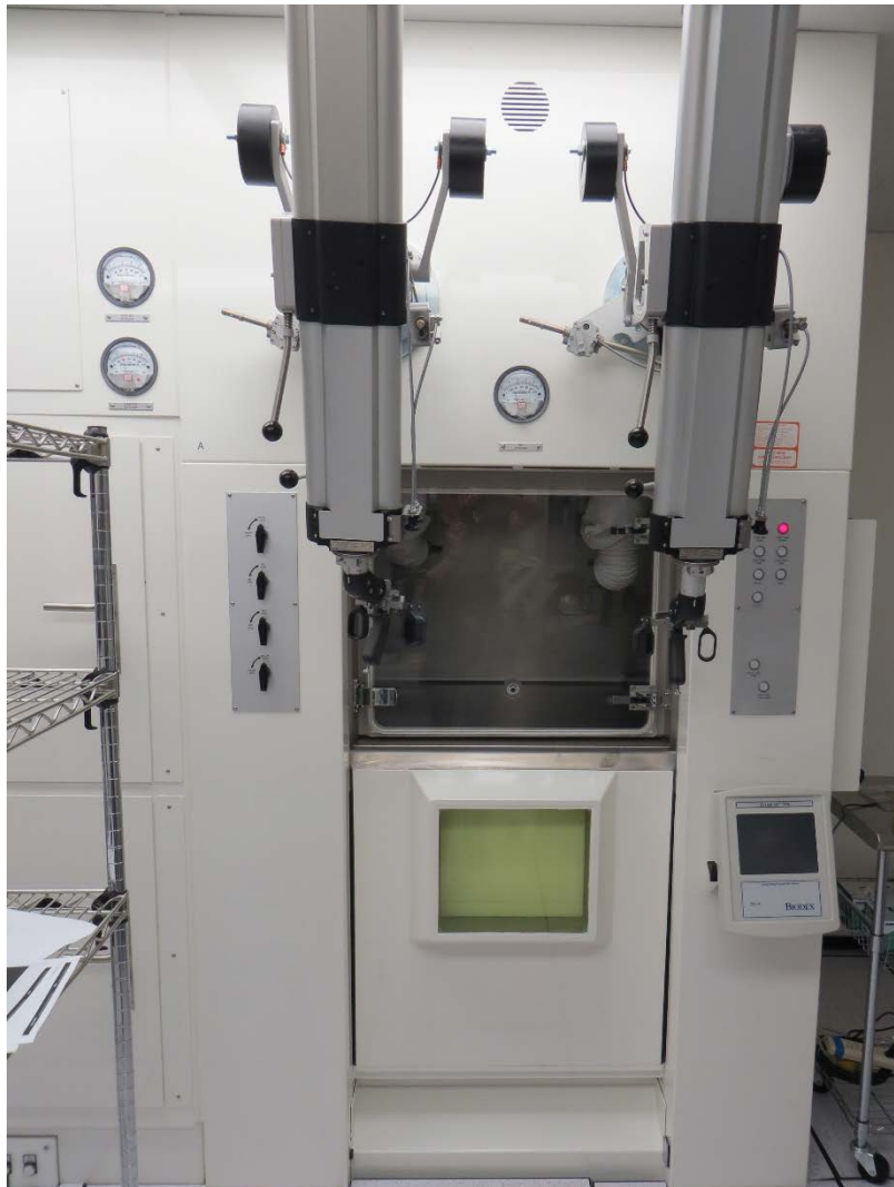
Figure 35. The hot cell, featuring remote manipulator arms, is shown. Note the control (lower right) for the dose calibrator (inside). Doors to the dual chemical enclosures are just visible to the left of the image.
