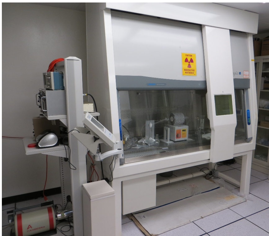
Figure 36. The fume hood with movable front shield is shown. Detection and assay equipment are visible to the left of frame.
