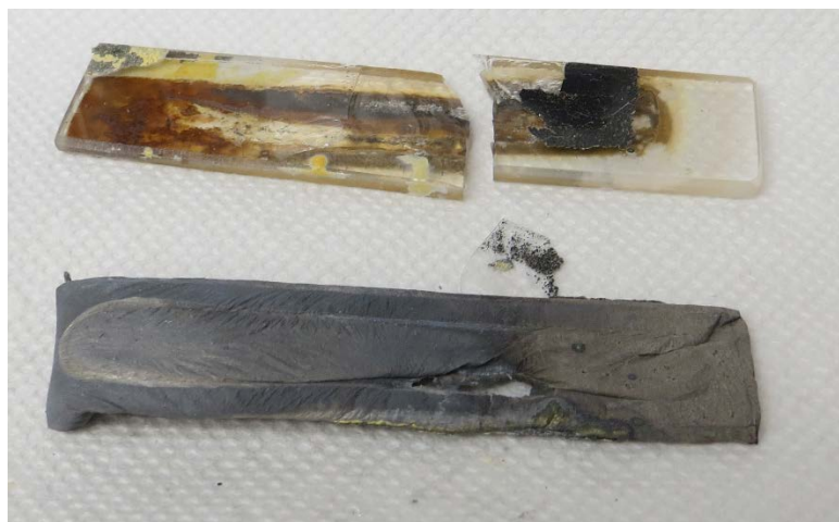
Figure 43. The target/target backing and quartz tray for Experiment 2 are shown after distillation.
