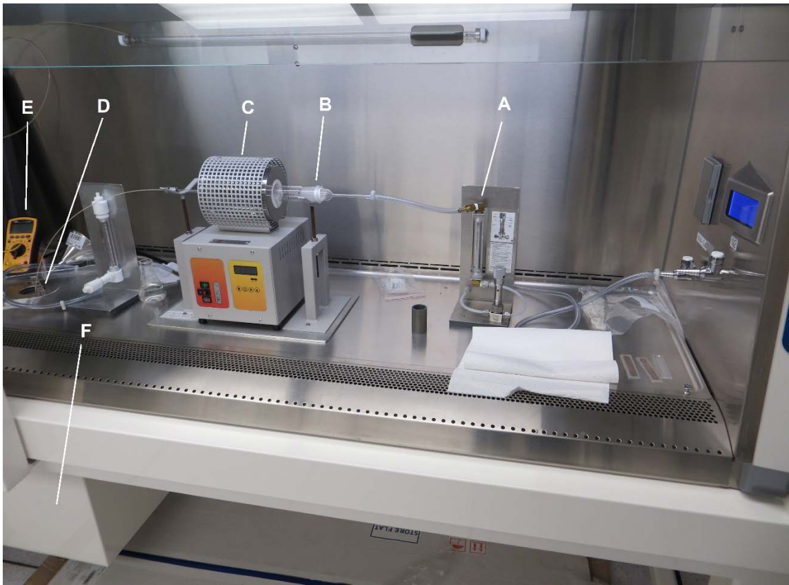
Figure 16. The distillation setup is shown. Argon is flowed through the regulator on the right (A), through the quartz tube (B) located within the tube furnace (C), and then through the capillary on the left into the cold trap (D). The cold trap is monitored for temperature (E) and is located in the shielded dose calibrator well (F), which allows for online monitoring of radioactivity (qualitative only).
