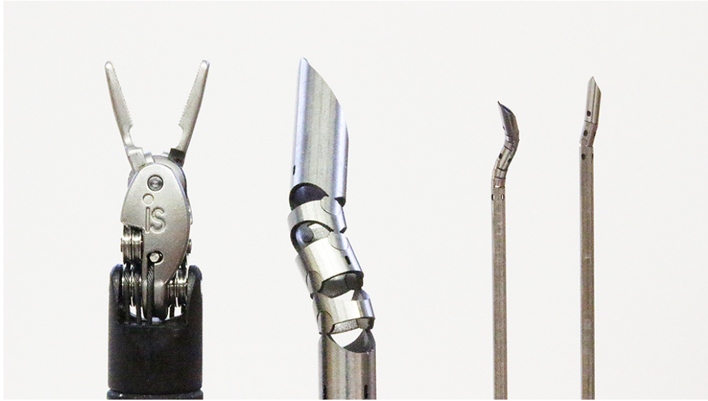
Figure 1.1: Examples of multi-DoF hinge joints embedded on miniature tubes by on-axis laser machining. From the left, an 8 mm diameter EndoWrist arm used in the da Vinci surgical robotic system (added for the size comparison), a 5 mm diameter Stainless Steel tube with 2-2 orthogonal hinge joints, a 1.27 mm diameter NiTi tube with 3-3 orthogonal hinge joints, and a 1.27 mm diameter NiTi tube with 1-1 orthogonal hinge joints.
