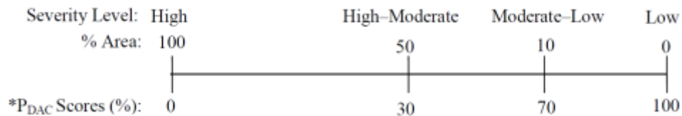
Figure 23. SCI Distress Evaluation and Scores—Distress Area Coverage (DAC).
