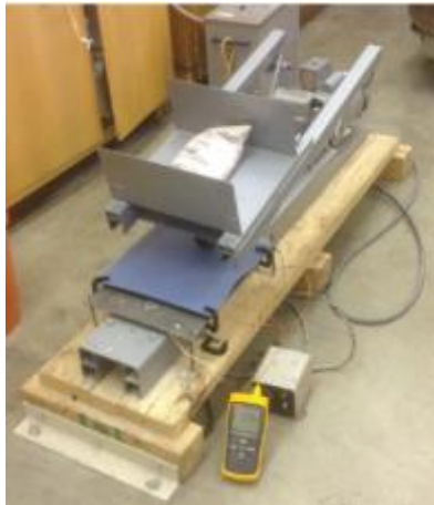
Figure 4. Final Modified Loaded Wheel Test Equipment, Reprinted From [23].
