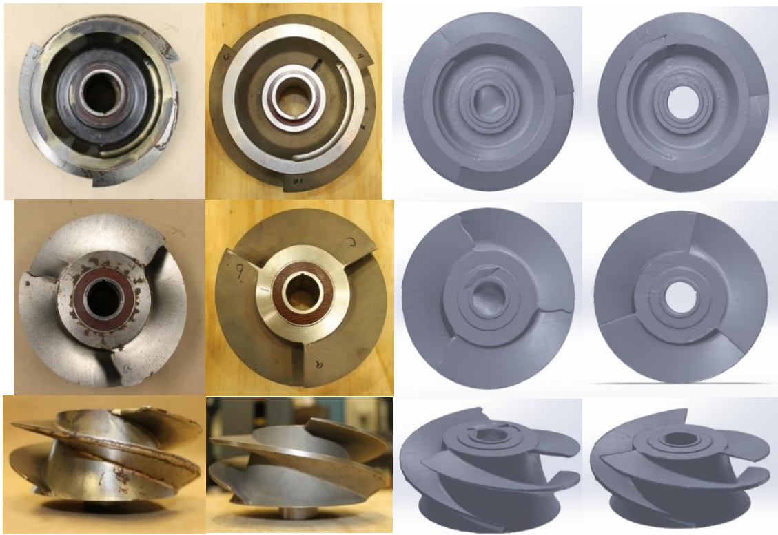
Figure 49: 1 st Impeller(Eroded and Original) Captured by Camera(left) and 3-D Scanner(right)
