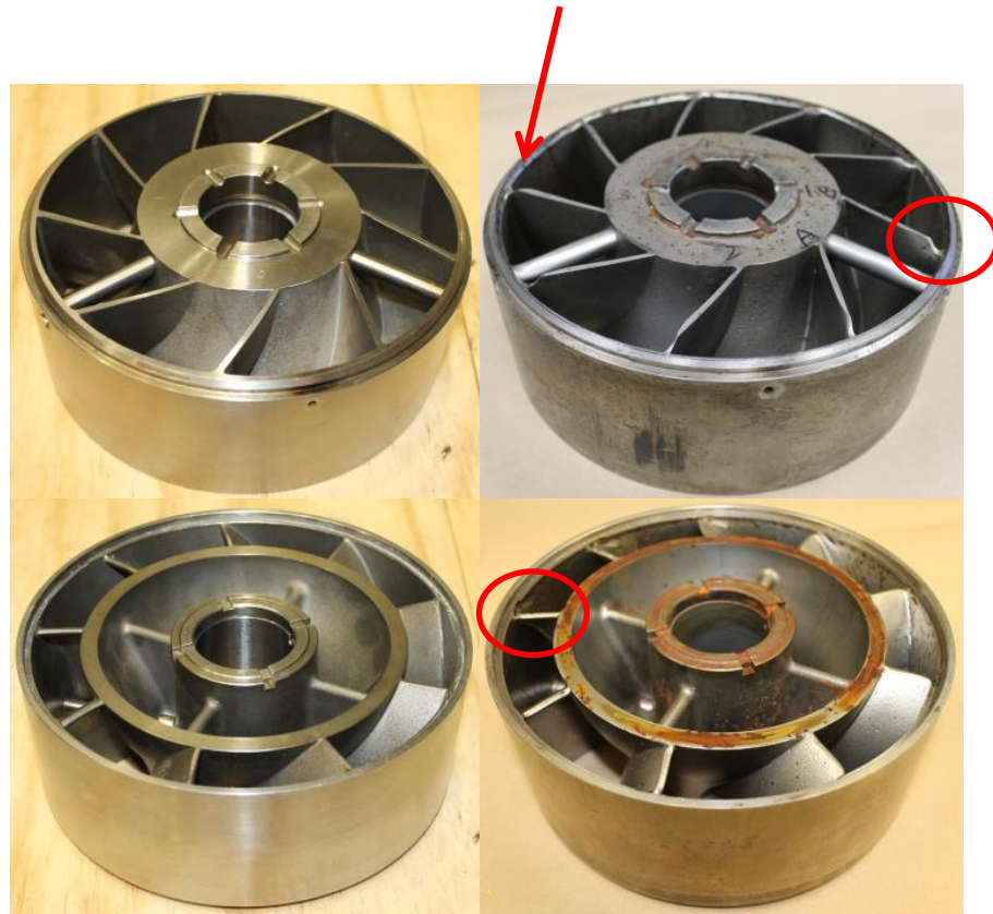
Figure 61: New and Eroded Diffuser of the 2nd Stage
