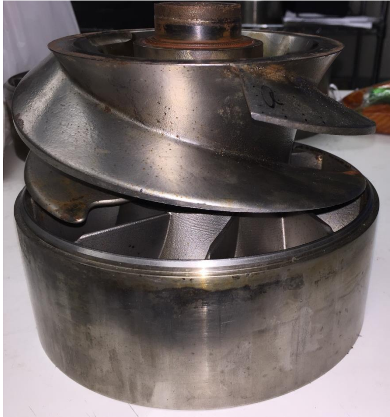
Figure 112: Eroded 1 st Diffuser and Eroded 2 nd Impeller
