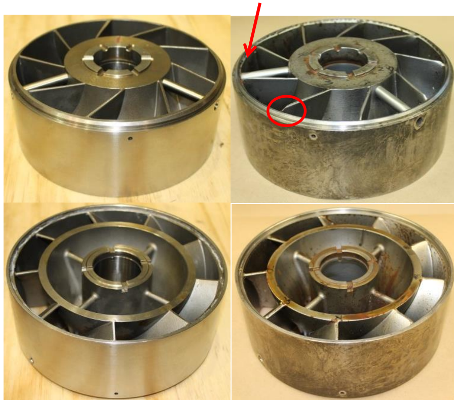
Figure 60: New and Eroded Diffuser of the 1 st Stage
