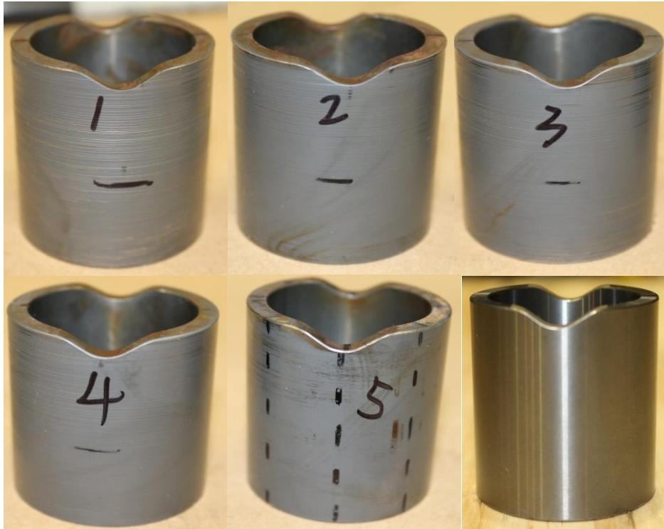
Figure 125: New and Eroded Journal Bearings
