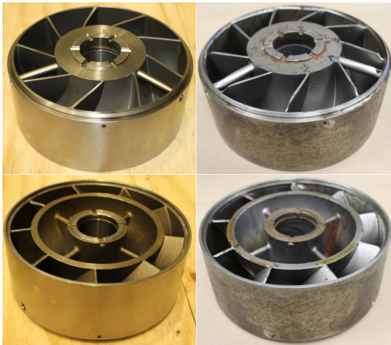
Figure 129: 3 rd Diffuser Comparison, Left: New, Right: Eroded
