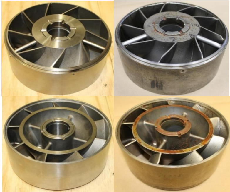
Figure 128: 2 nd Diffuser Comparison, Left: New, Right: Eroded
