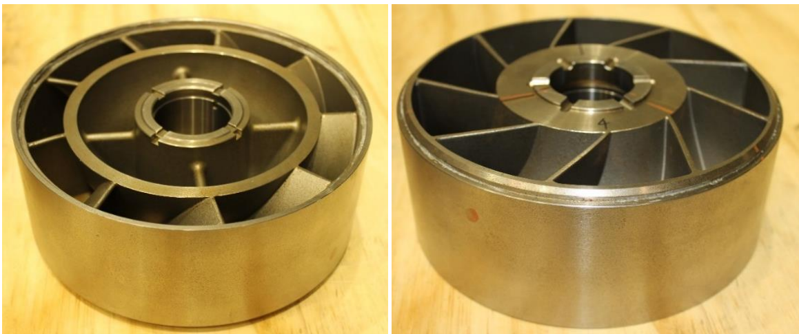
Figure 31: Diffuser of Poseidon ESP
