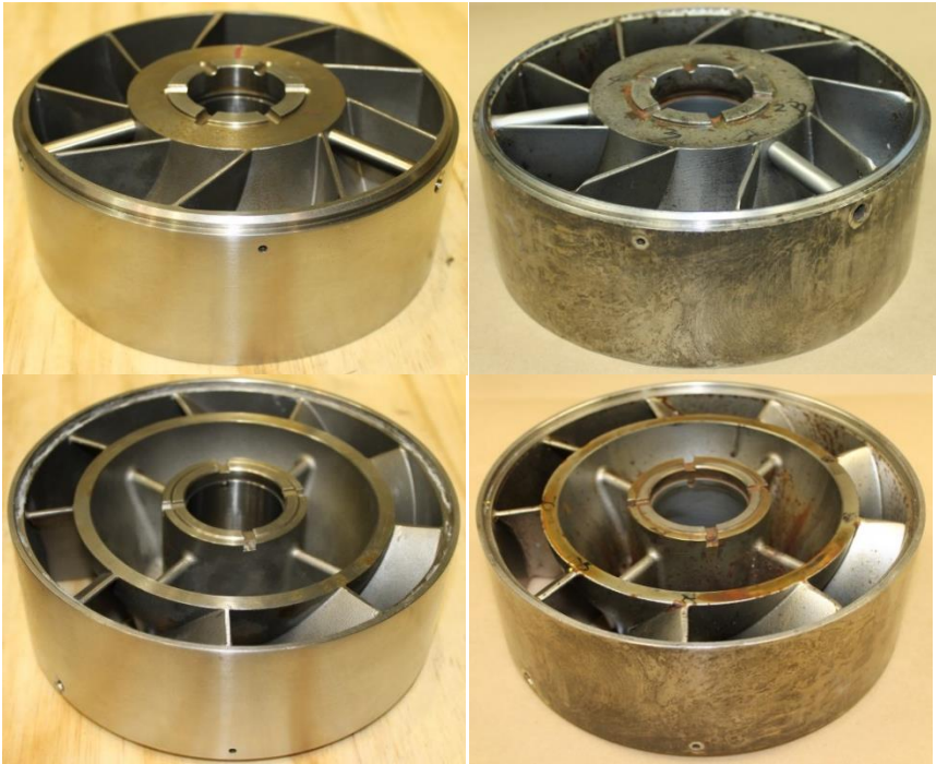
Figure 127: 1 st Diffuser Comparison, Left: New, Right: Eroded
