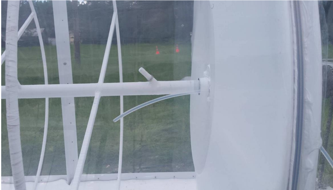
Figure 2. Picture of FEP tube extending inside of the chamber. This allows for the replacement of filtered air inside the chamber during sampling.
