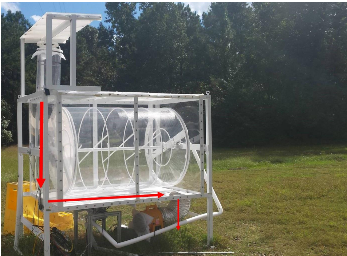
Figure 3. Ambient air flow system inside the chamber enclosures. Ambient air is pulled by a blower on the bottom through a hole in the top. The air path is shown in red.
