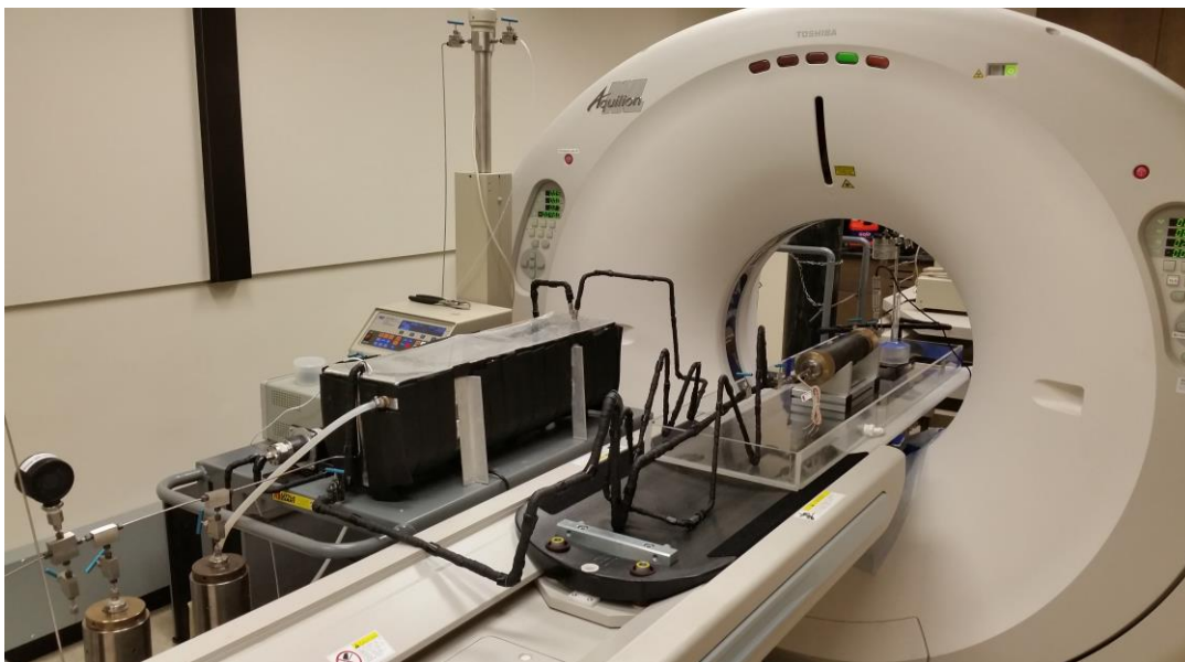
Figure 10. Experimental setup for core-flooding experiments in ULR.
