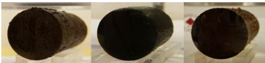
Figure 26. Cores Bk-2/1 (left), EF-1/2 (center) and W-1/4 (right) under spontaneous imbibition experiment. Reprinted with permission from Alvarez and Schechter (2016c).
