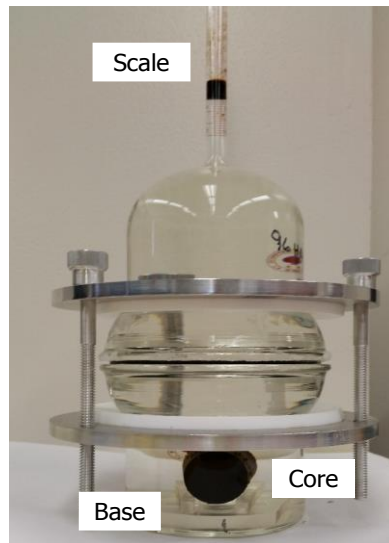
Figure 7. Modified Amott cell for spontaneous imbibition experiments. Reprinted with permission from Alvarez and Schechter (2017)
