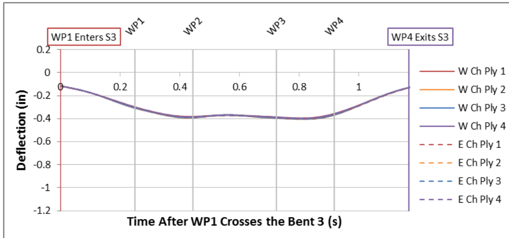
Figure A-116: IC1 20 MPH Total Midspan Stringer Deflections
