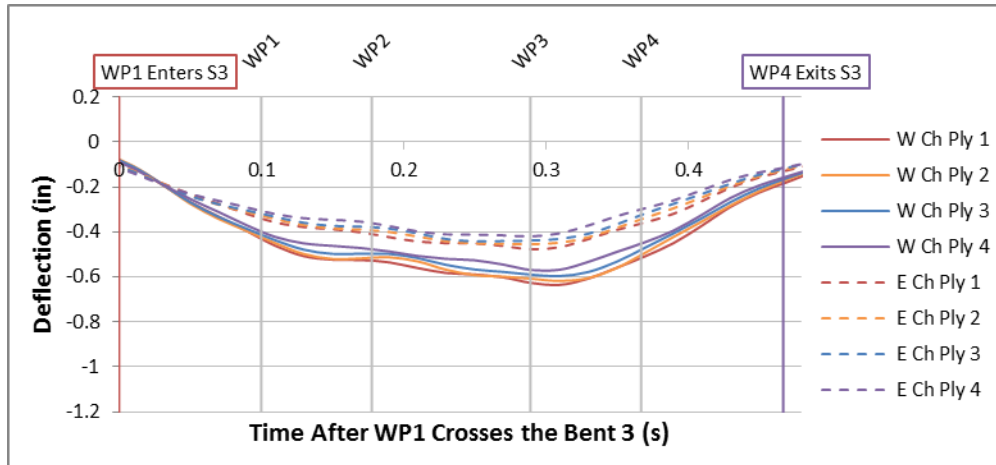
Figure A-170: IC4 50 MPH Total Midspan Stringer Deflections
