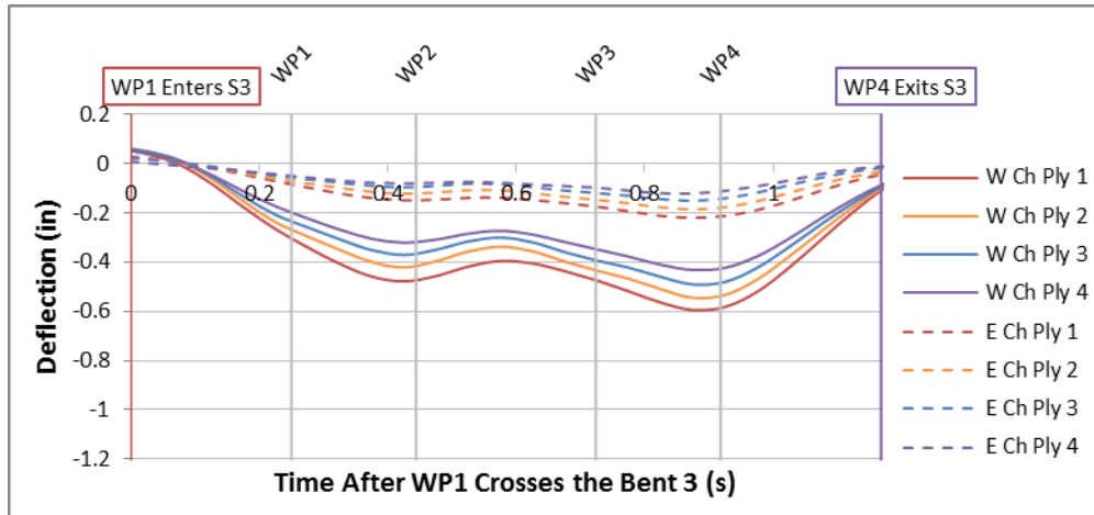
Figure A-129: IC5 20 MPH Net Midspan Stringer Deflections
