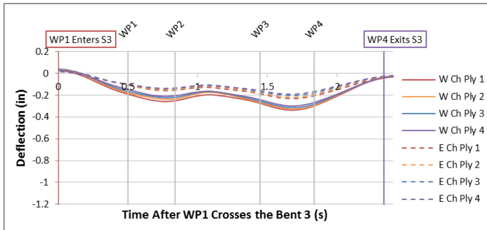
Figure A-111: IC4 10 MPH Net Midspan Stringer Deflections
