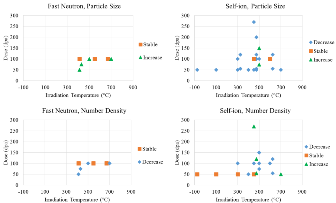
Figure 6-6. Summary of size and number density of oxide particle in ODS alloy irradiated by fast neutron or self-ion from open literatures.
