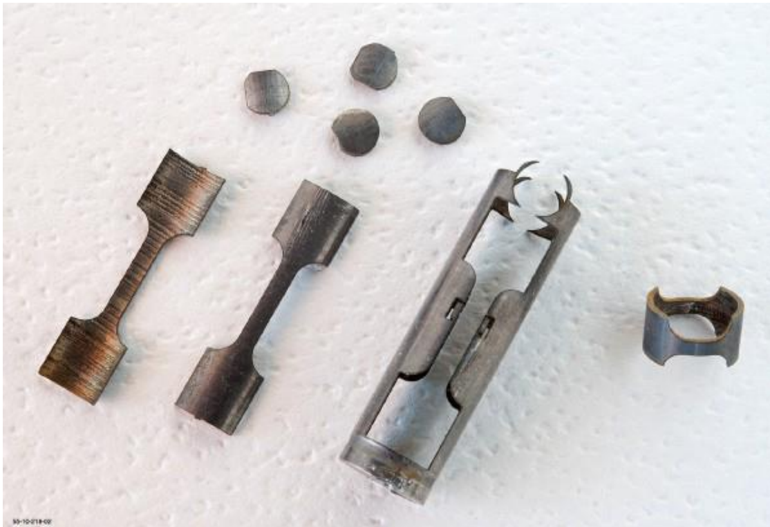
Figure 3-1. Photo of pressurized tubes and specimens cut from it.
