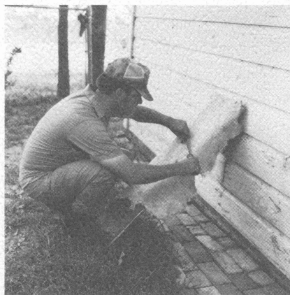
All flesh must be removed from the hide before tanning. This is done by repeated scraping with a knife.
