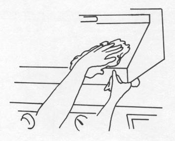
Occasionally take the metal filter out of the hood. Put the filter in warm, soapy water. Let it soak for a few minutes. Wash and rinse it. Dry the filter and put it back in the hood.
