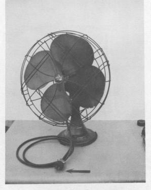
5. This fan has the proper 3 prong plug and "grounded" cord attached. It will provide a safe appliance if used with a properly grounded receptacle.
