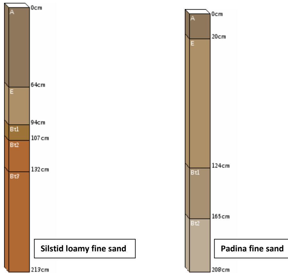
Figure 1. Soil profile of the burned watershed soil Silstid loamy fine sand (left) and the unburned watershed soil Padina fine sand (right) (Soil Survey Staff 2013).
