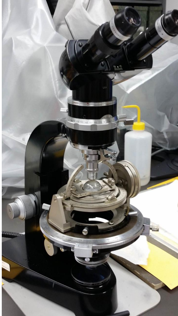
Figure 13. Universal Stage Microscope used to measure lattice preferred orientations of sample EG-2 that shows major axis a and minor axis c
