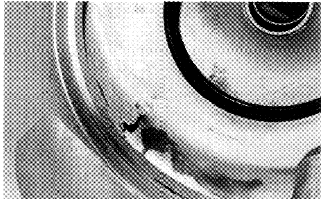
Figure 6. Closeup View Showing Wear of Plasma Applied Tungsten Carbide Coating in Pump Casing After One Year of Service.
