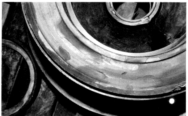
Figure 7. Pump Head, Showing Failure of Plasma Applied Tungsten Carbide Coating After One Year Service.
