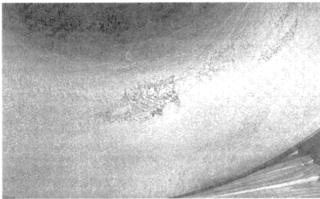
Figure 4. Early Suction Bell Damage Is Localized.
