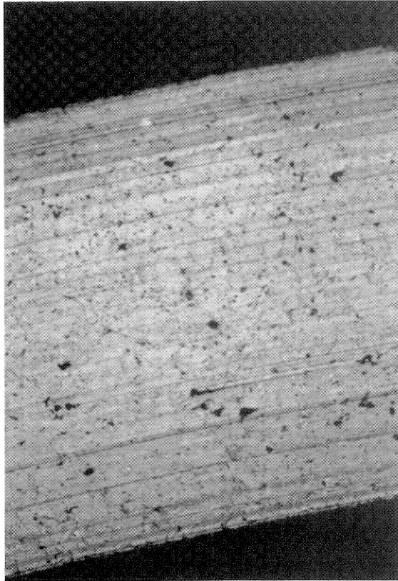
Figure 13. Face of the C Ring of a Textured Seal after 550 Hours of Operation in Sandy Water.
